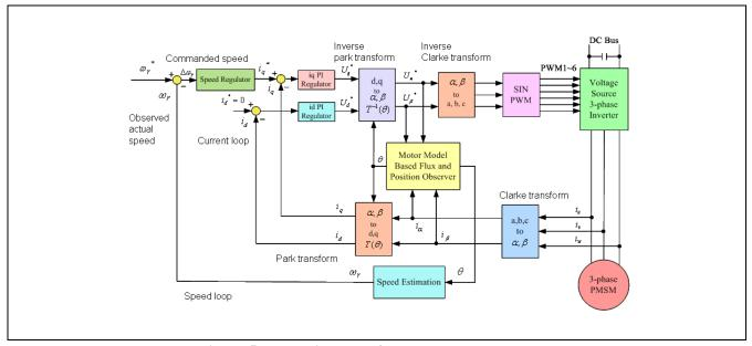
Figure 5 Block diagram of sensorless vector control
