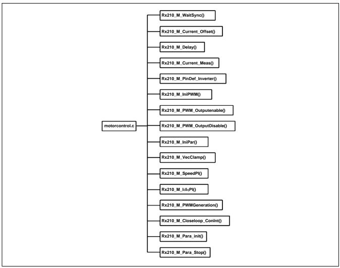
Figure 11 Functions in motorcontrol.c
