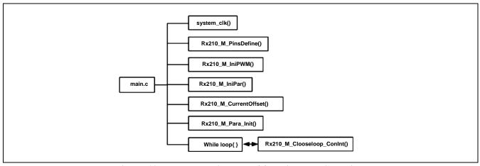
Figure 10 Block diagram of function calls in main.c
