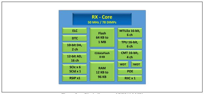
Figure 3 Block diagram of RX210 MCU
