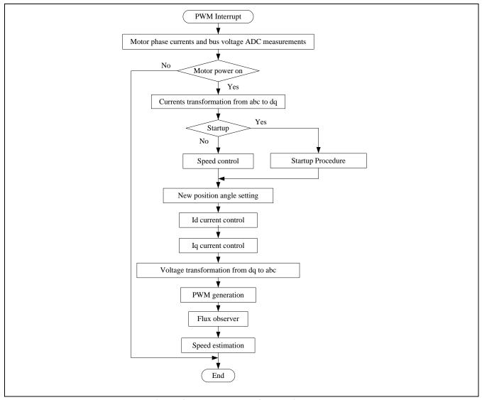
Figure 9 Flowchart of PWM interrupt
