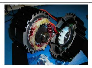
Figure 13 A physical BLDC motor for parameter tuning
