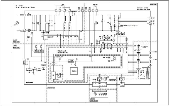
Figure 2 System block diagram for High Voltage Inverter Platform
