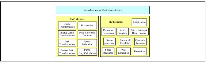
Figure 6 Software architecture of RX210 SVC
