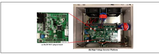
Figure 1 System setup with (a) RX210 MCU plug-in board and (b) High Voltage Inverter Platform
