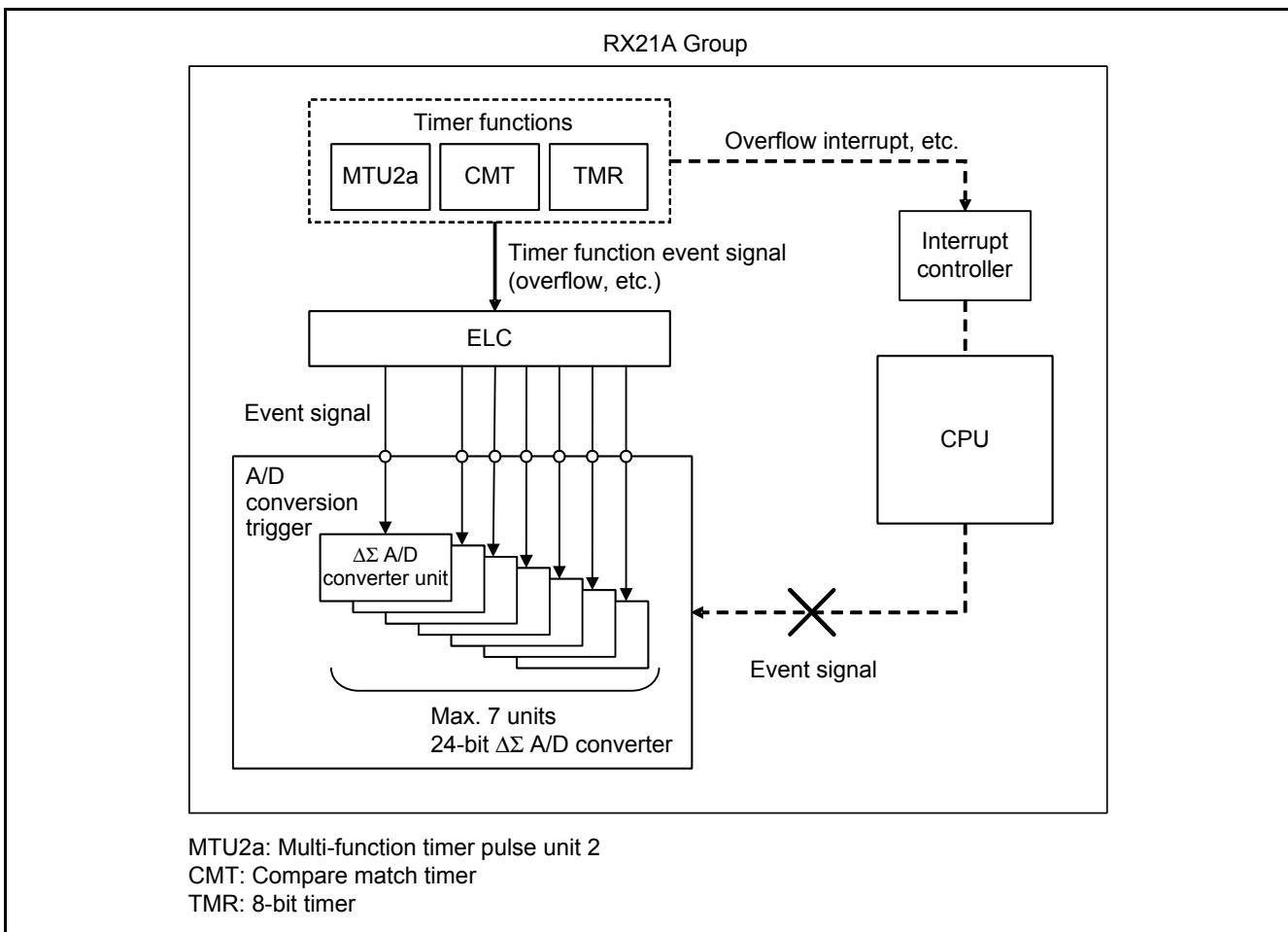
Figure 2.2 A/D Conversion Trigger Signal Sequence
