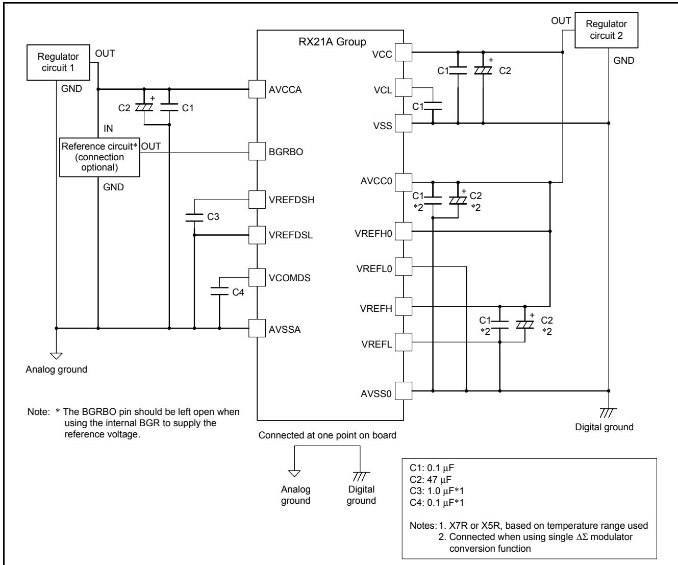
Figure 3.1 Example Power Supply Circuit for Use with  $\Delta\Sigma$  A/D Converter of RX21A Group
