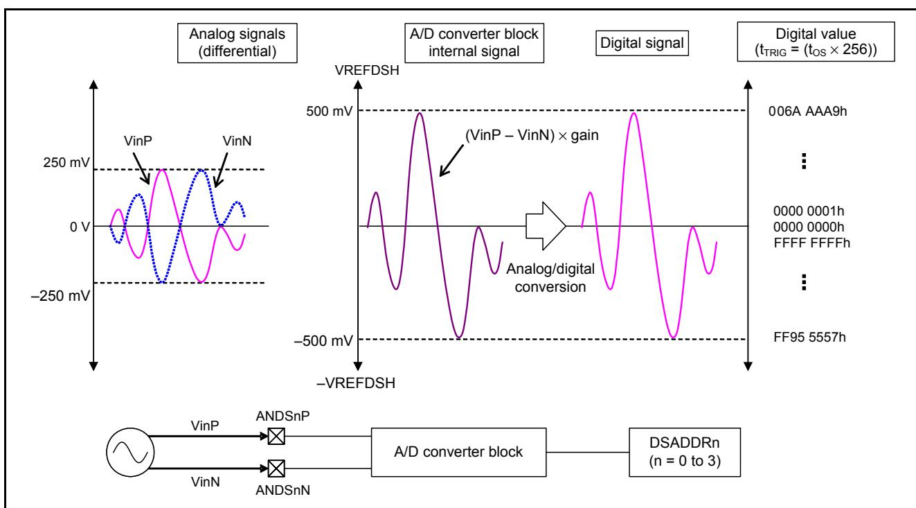
Figure 2.10 Example of Differential Input
