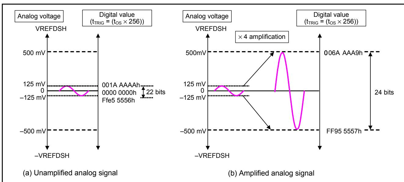
Figure 2.7 Usage Example of Gain Function
