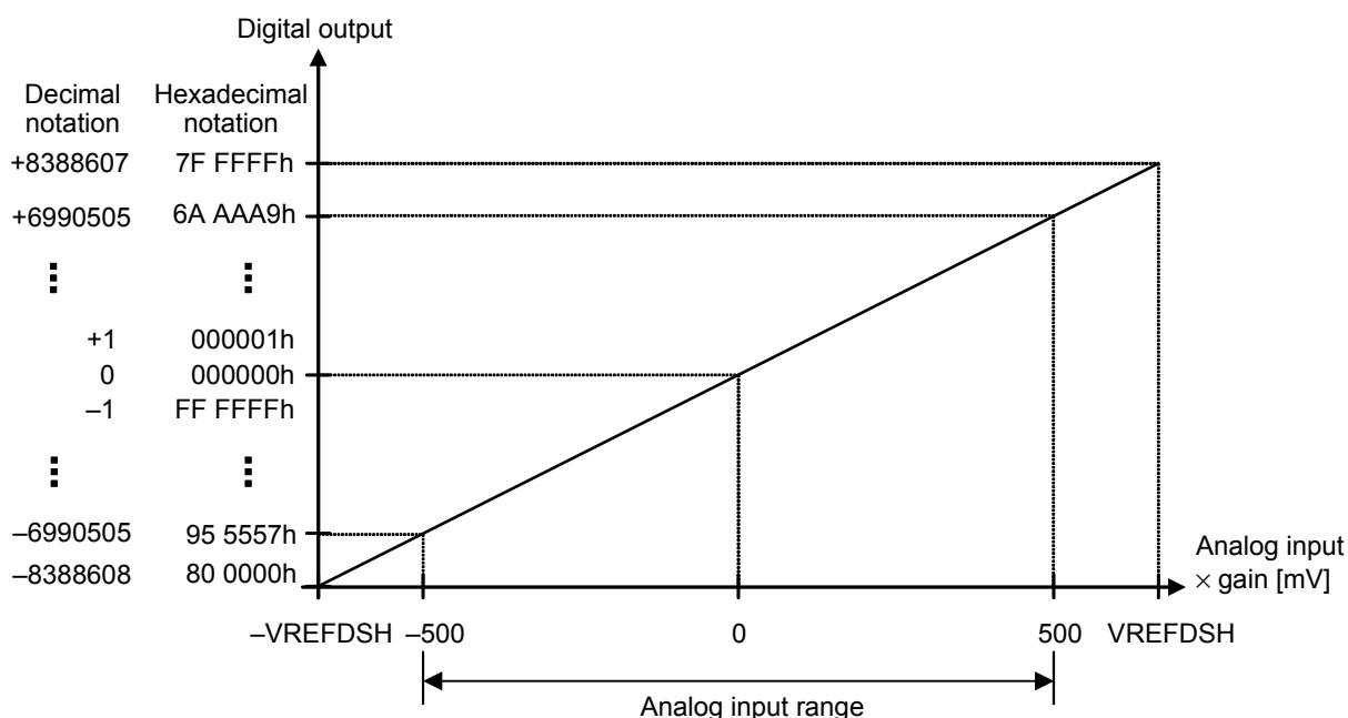
Figure 2.4 Relationship between Analog Input and Digital Output
