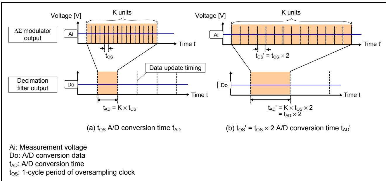
**Figure 2.5 Outline of A/D Conversion Time of  $\Delta\Sigma$  A/D Converter**
