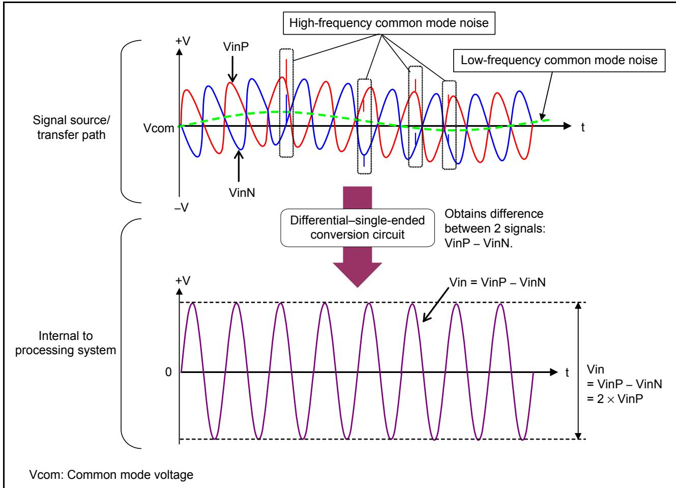
Figure 2.9 Conceptual View of Differential Signals
