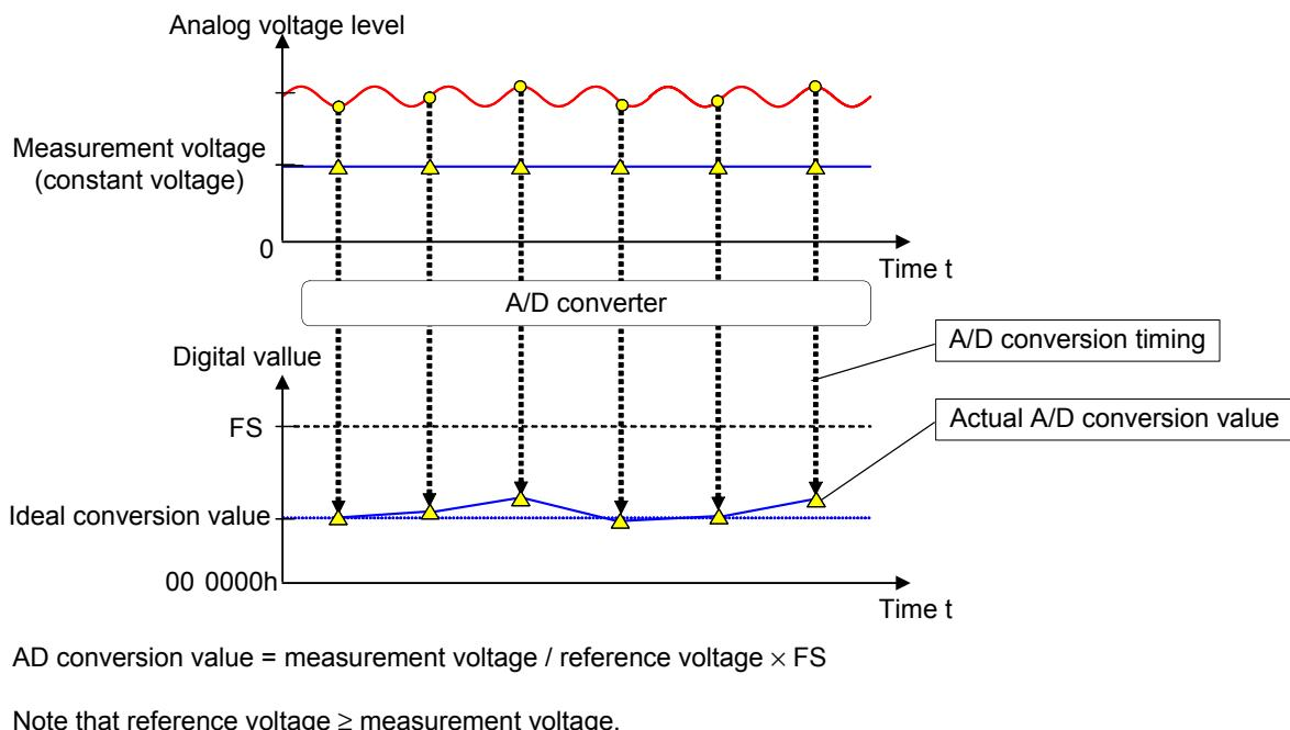
**Figure 2.11 A/D Conversion Results with Low-Accuracy Reference Voltage**
