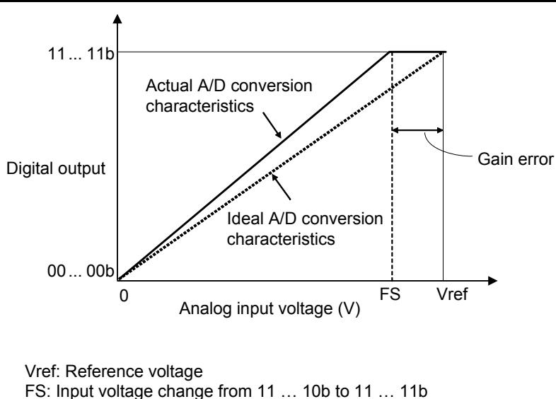
**Figure 6.1 Gain Error of A/D Converter**
