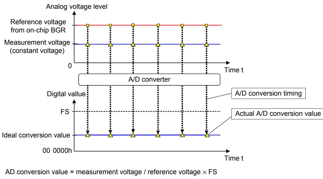
**Figure 2.12 A/D Conversion Results with Highly Accuracy Reference Voltage**
