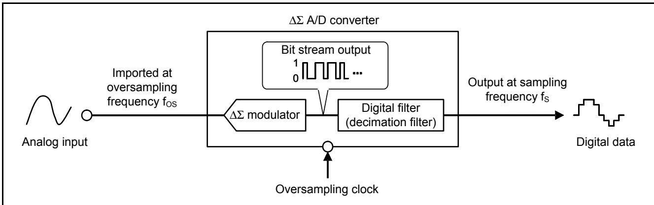
**Figure 1.3  $\Delta\Sigma$  A/D Converter Block Diagram**
