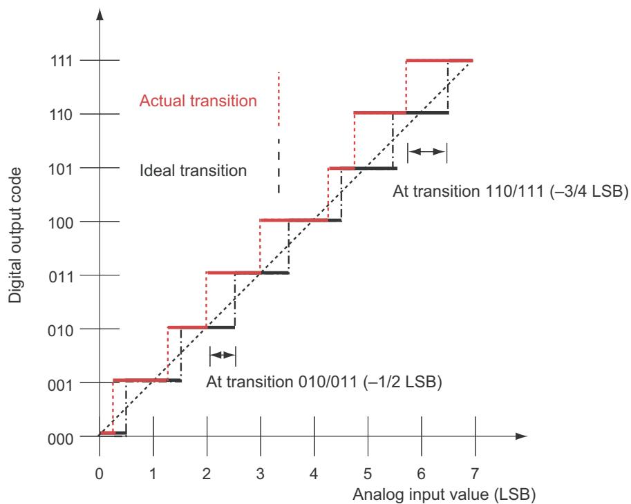
Figure 6.5 Integral Nonlinearity Error
