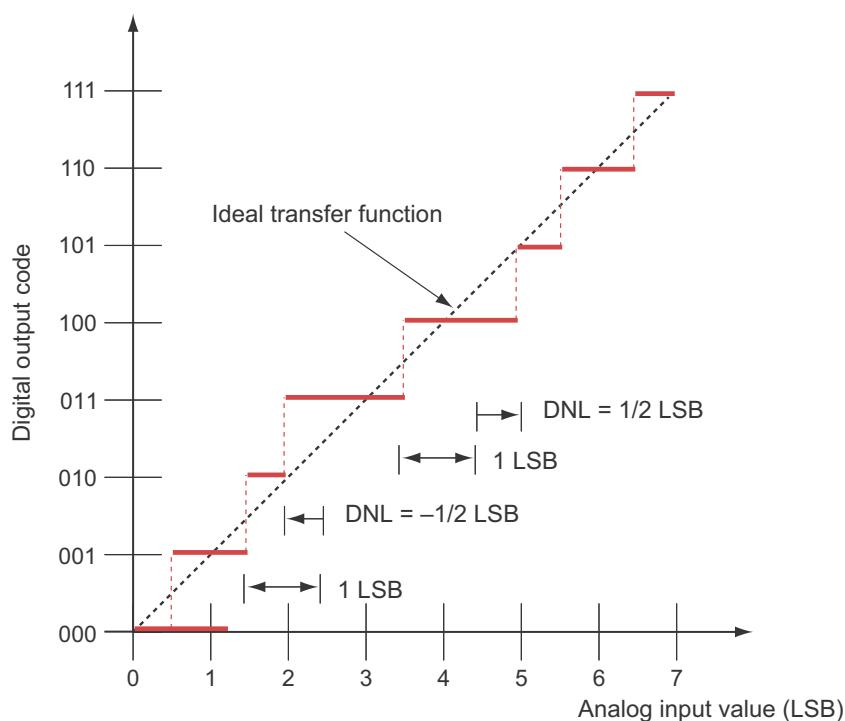
Figure 6.4 Differential Nonlinearity Error
