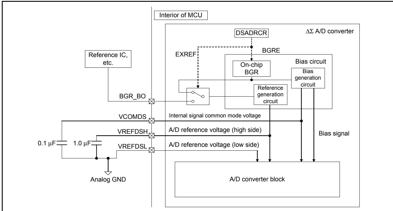
**Figure 2.13 Block Diagram of On-Chip Reference Circuit**
