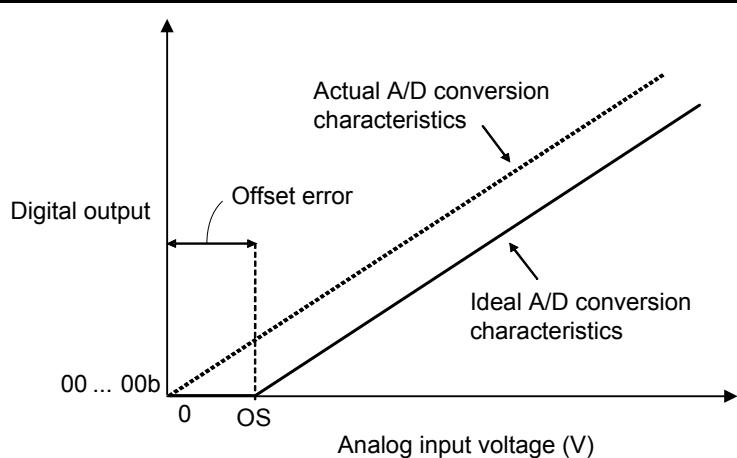
Figure 6.2 Offset Error of A/D Converter
