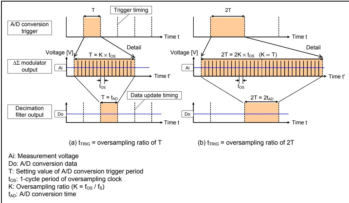
Figure 2.6 RX21A Group A/D Conversion Trigger Period and Oversampling Ratio
