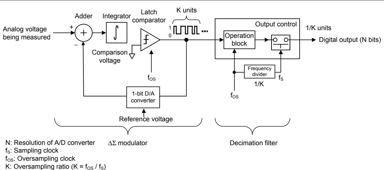
**Figure 1.2 Internal Structure of ΔΣ A/D Converter**
