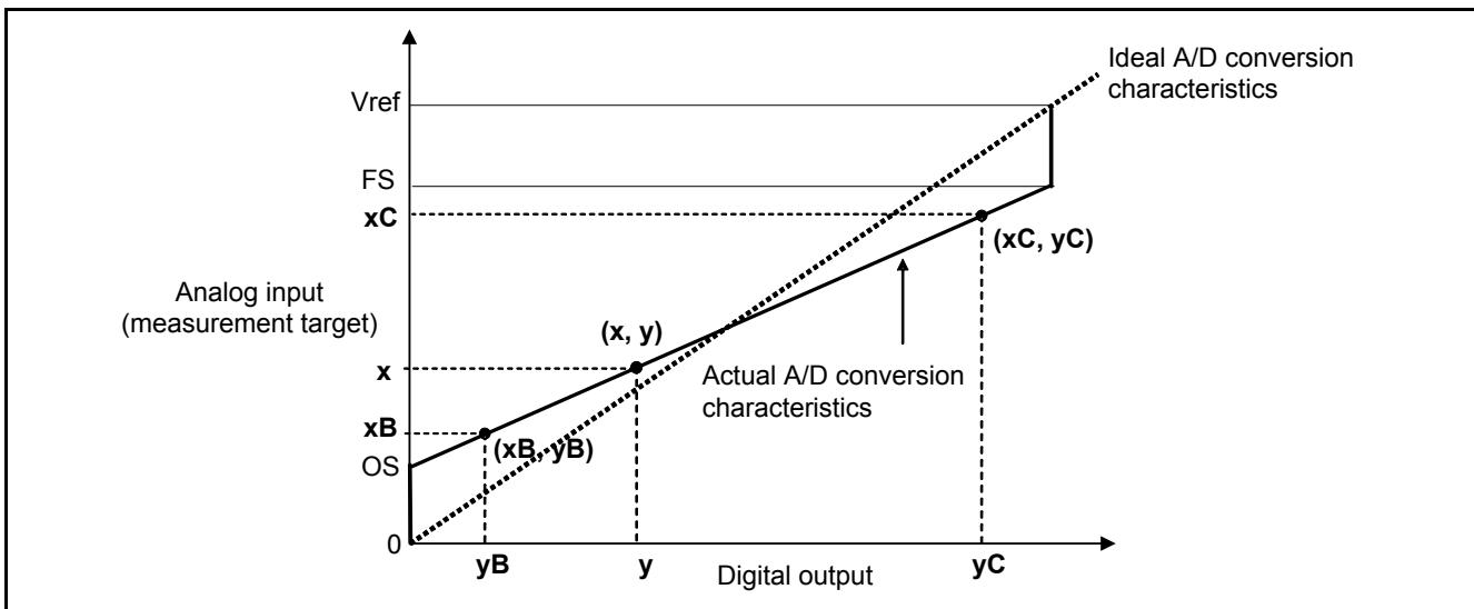
**Figure 4.2 Error Correction Concept**
