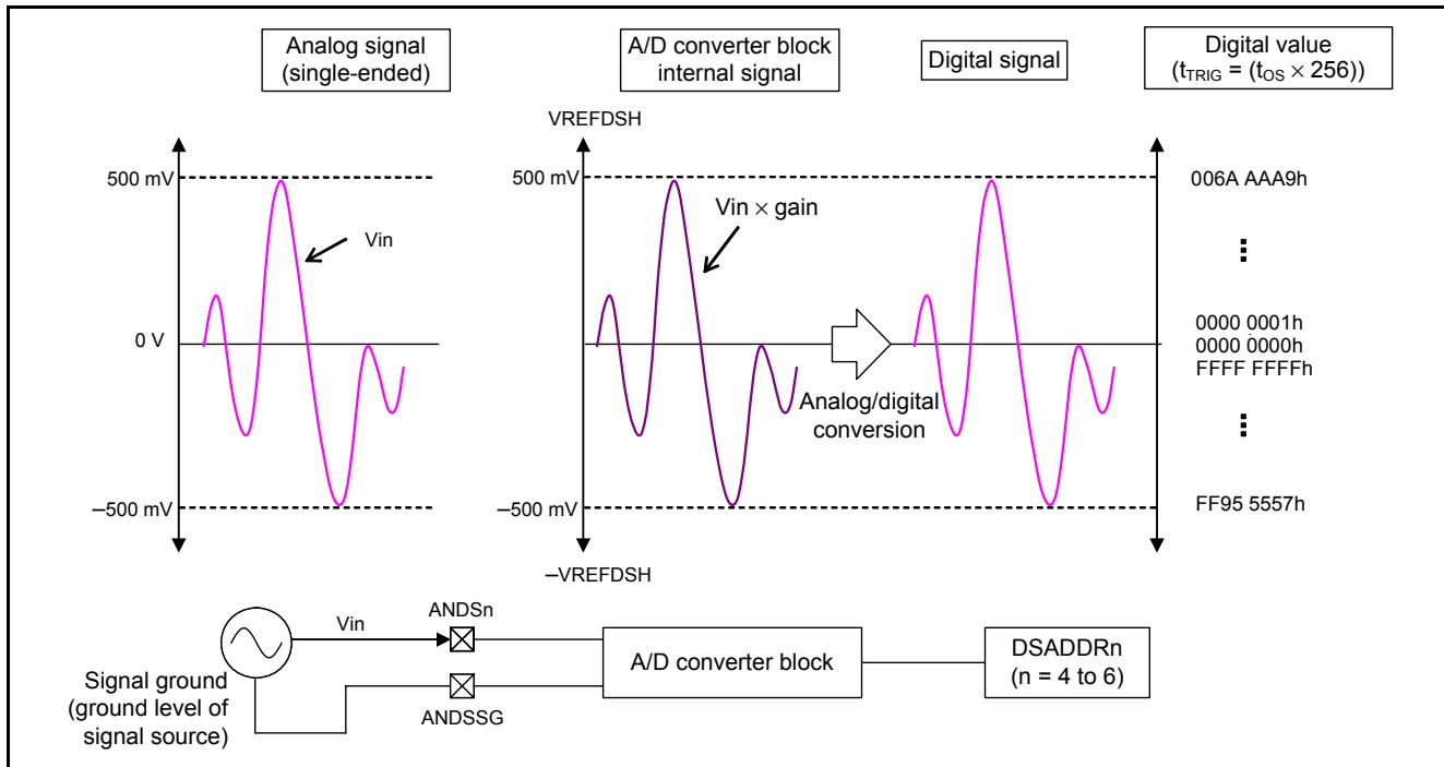
Figure 2.8 Example of Single-Ended Input
