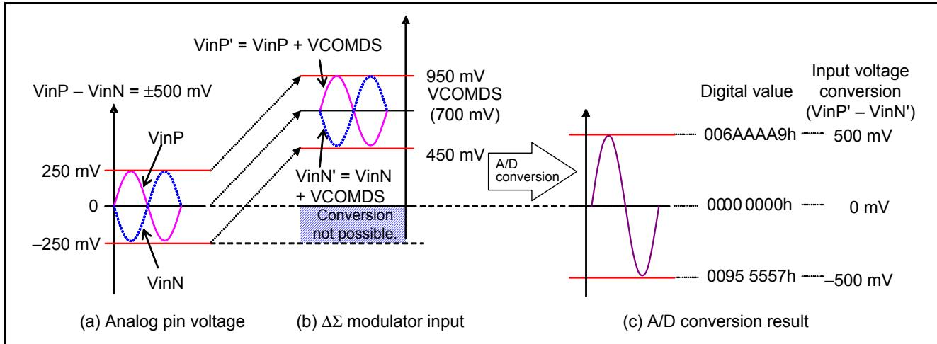
Figure 2.15 Internal Signal Processing by  $\Delta\Sigma$  A/D Converter
