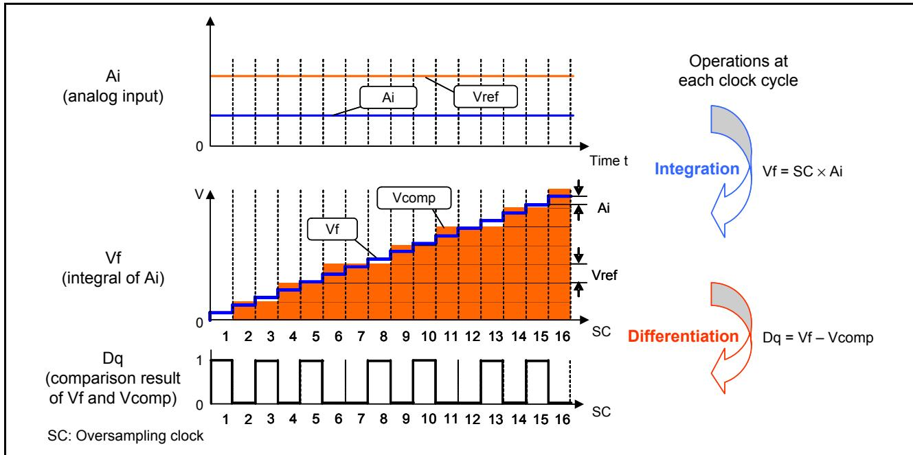
**Figure 1.5 A/D Conversion by  $\Delta\Sigma$  Modulator**
