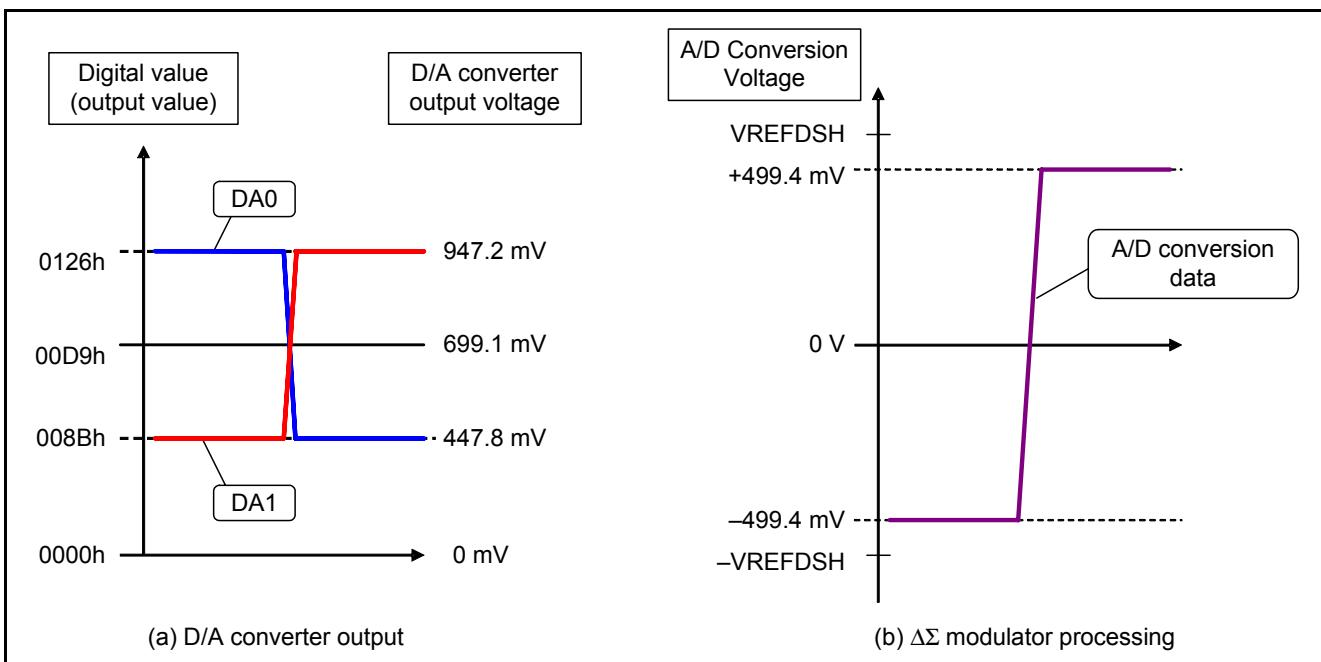
Figure 2.16 Differential Input Setting Example with  $\Delta\Sigma$  Modulator Gain of  $\times 1$
