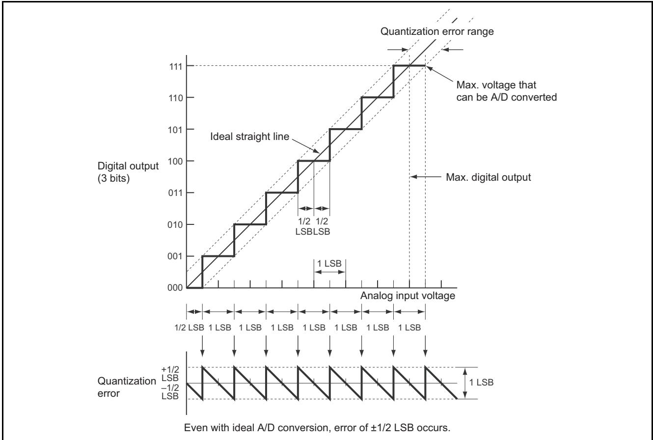
**Figure 6.3 Quantization Error**
