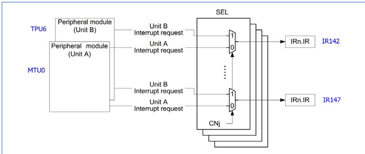
Figure 2 - Interrupt Unit Selection
