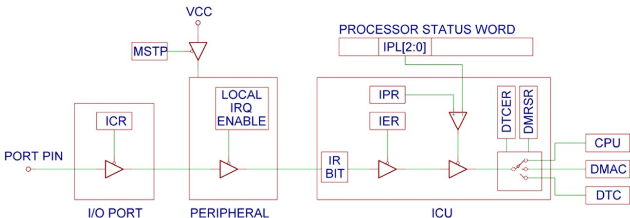
Figure 10.1 - RX Interrupt Flow
