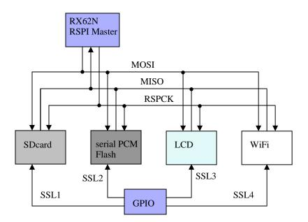
Figure 1: RSPI connected peripherals on the YRDKRX62N
