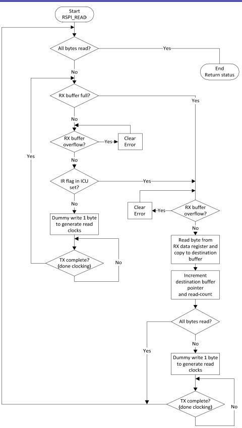
Figure 3 RSPI\_READ function flow diagram
