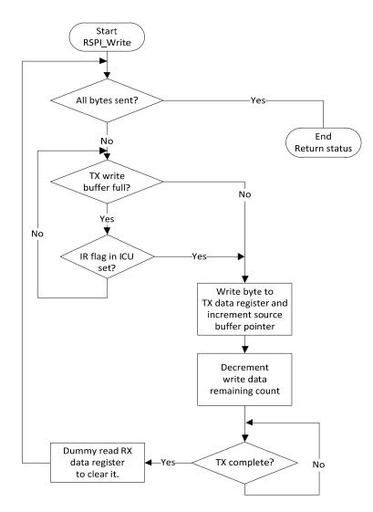
Figure 2: RSPI\_Write function flow diagram
