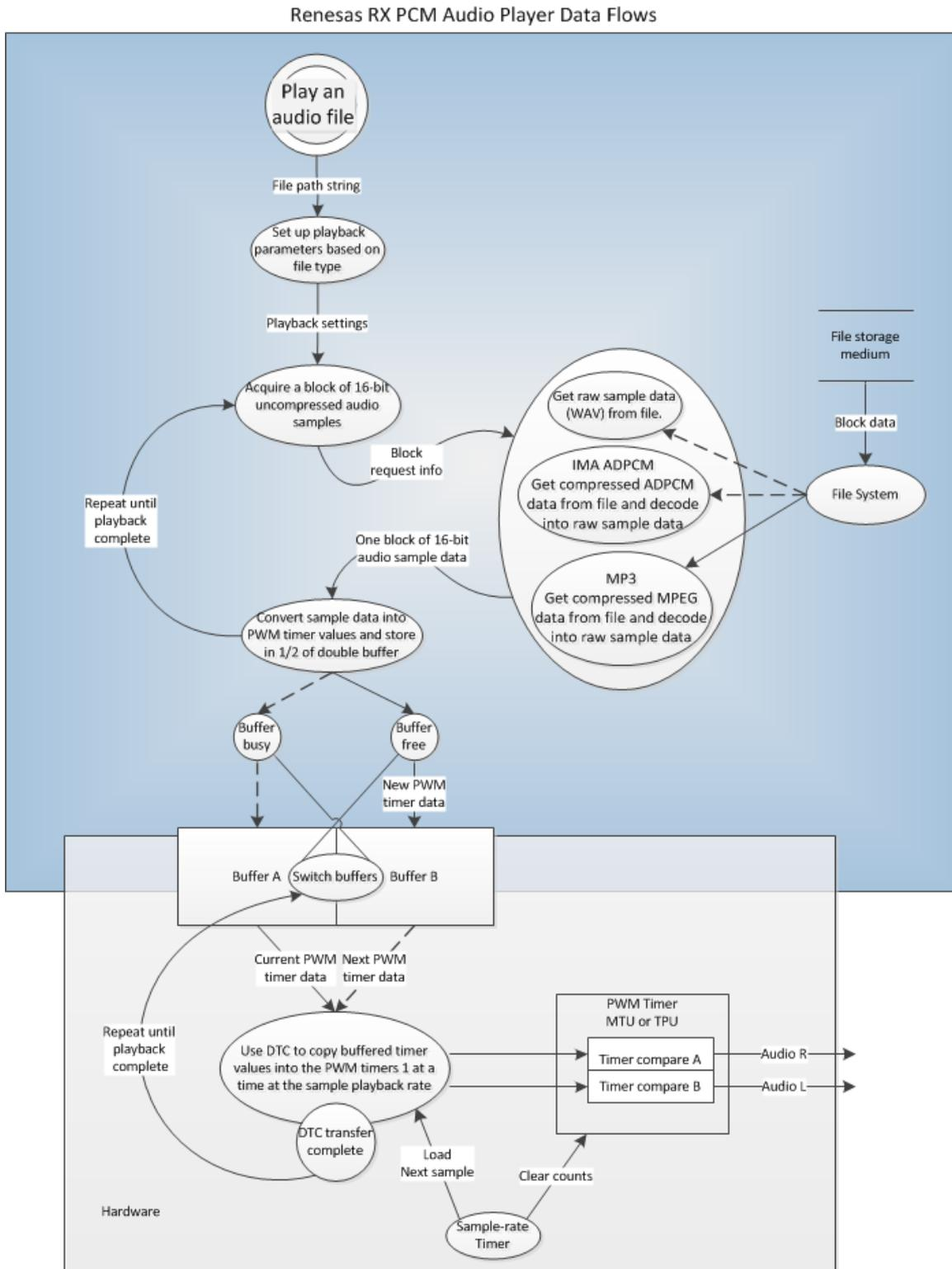
Figure 1 principle of operation
