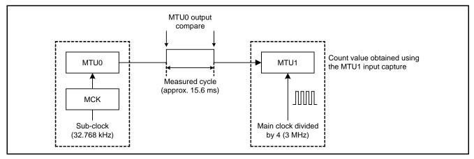
Figure 1.1 Block Diagram
