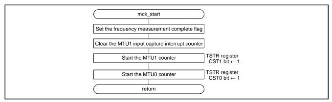
Figure 4.4 Start Frequency Measurement
