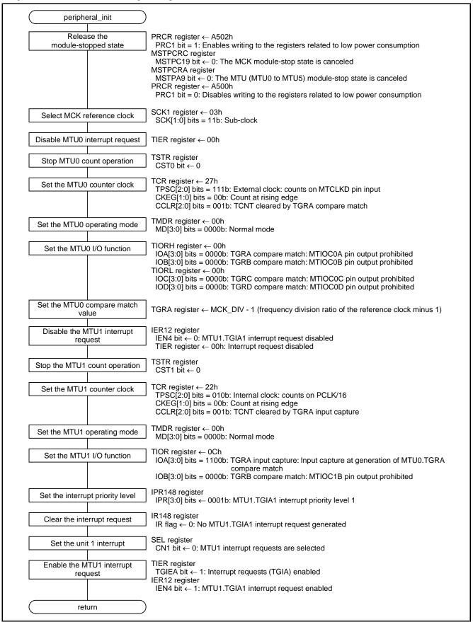
Figure 4.3 Initial Setting of Peripheral Functions
