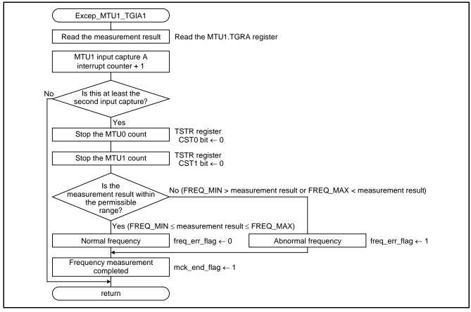
Figure 4.5 MTU1 Input Capture A Interrupt Handling
