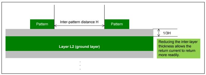
Figure 3 Return Current (Inter-layer Distance)
