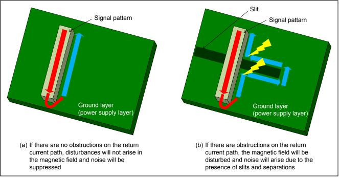
Figure 6 Return Current (Facilitated by Ground Layer)
