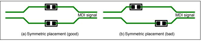
Figure 7 Layout of Components on Differential Signal Transmission Paths
