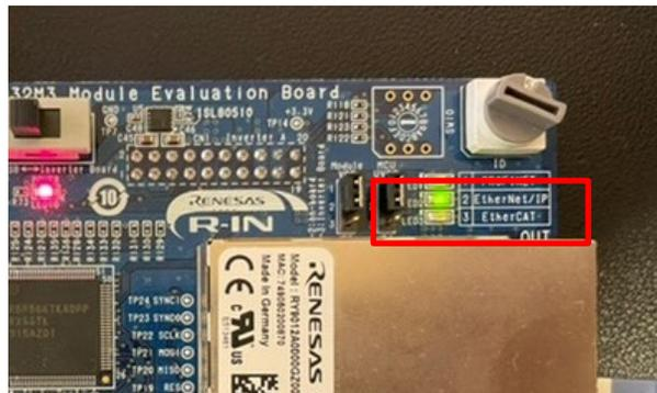
**Figure 3-41 Protocol LED: EtherNet/IP**
