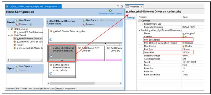
Figure 5-2 Ethernet Driver Configuration for VSC8531 (e.g. ETH0)
