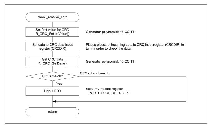
Figure 6.6 Serial Incoming Data Setting Processing
