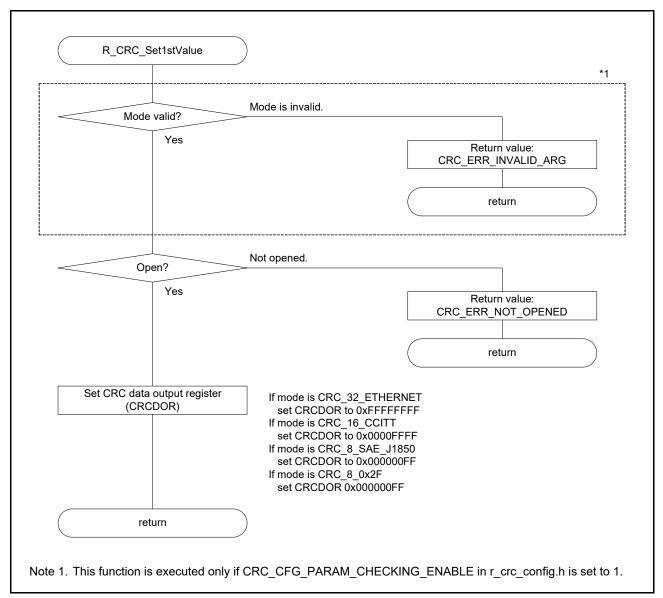
Figure 6.8 CRC Data Generation Register Starting Value Setting Function
