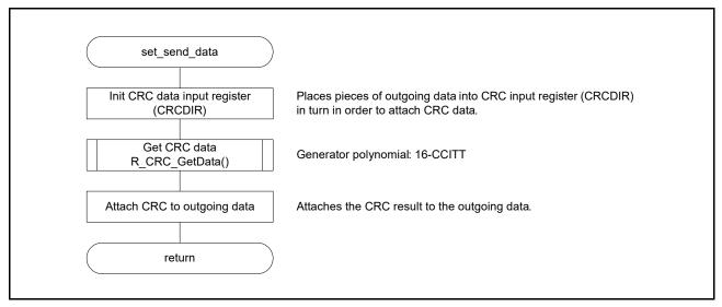
Figure 6.5 Serial Outgoing Data Setting Processing
