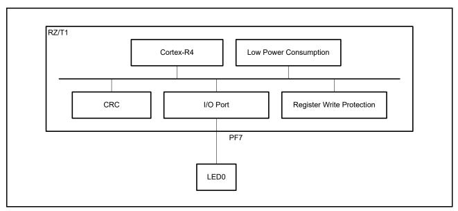
Figure 5.1 Hardware Configuration
