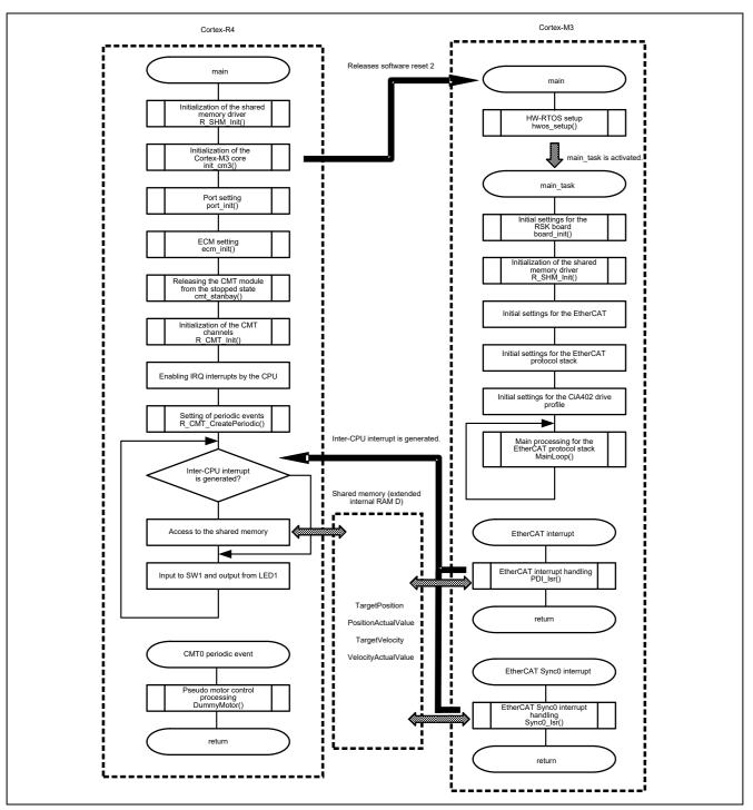
Figure 5.4 Simple Flowchart of the CiA402 Sample Program
