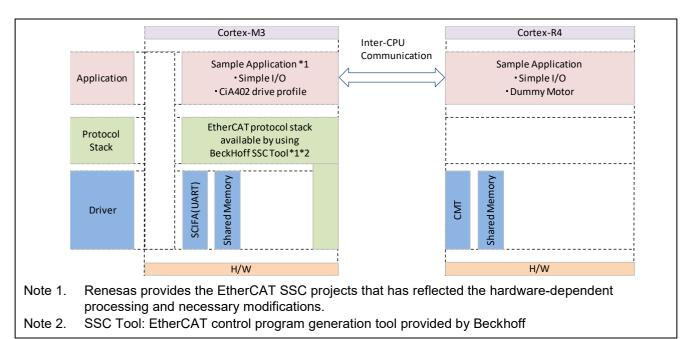
Figure 5.1 Software Structure Example
