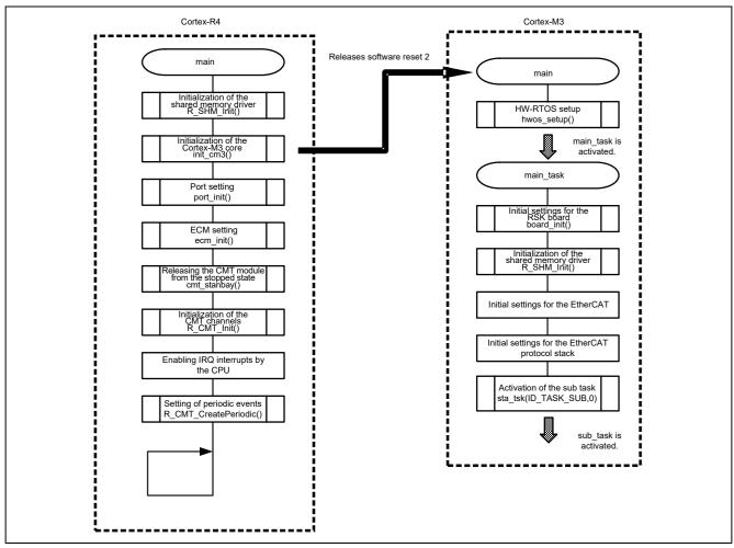
Figure 5.2 Simple Flowchart of the I/O Controller Sample Program (1)
