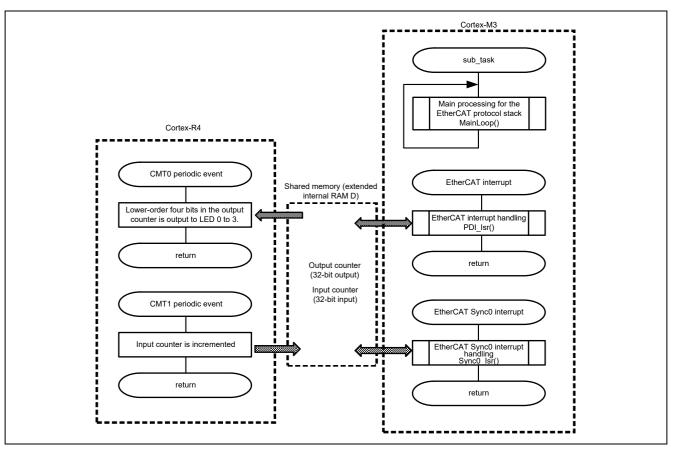
Figure 5.3 Simple Flowchart of the I/O Controller Sample Program (2)
