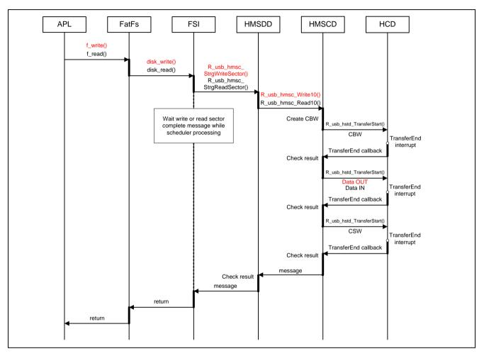
Figure 3-2 USB Storage Device Access Sequence
