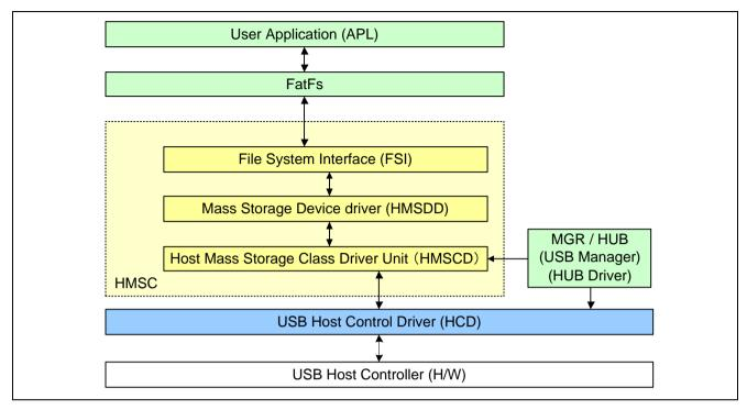
Figure 2-1 Software Block Diagram
