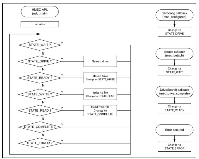
Figure 4-2 Main Loop flowchart
