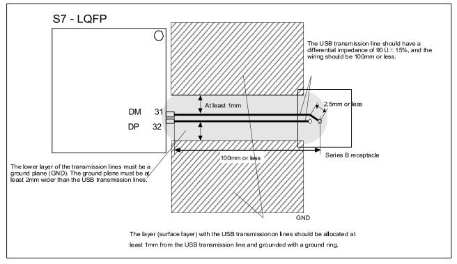
Figure 2 Design Example of a Device Controller USB Transmission Line Pattern
