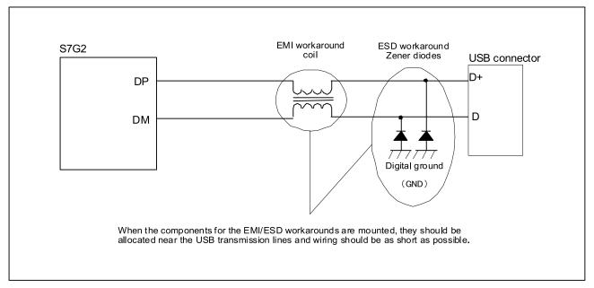
Figure 6 Connection Example When Components for EMI/ESD Workarounds are used
