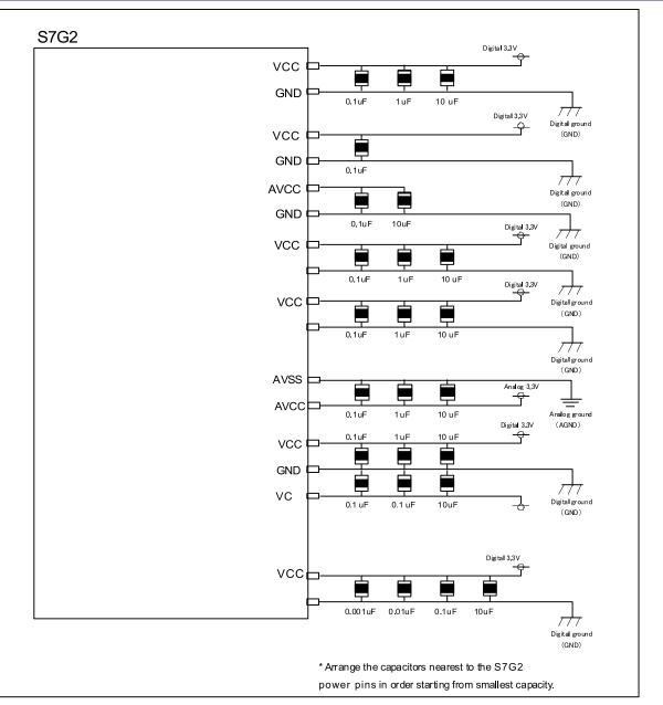
Figure 4 Example of Decoupling Capacitor Allocation
