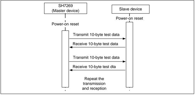
Figure 5.1 Communication Sequence with Salve Device
