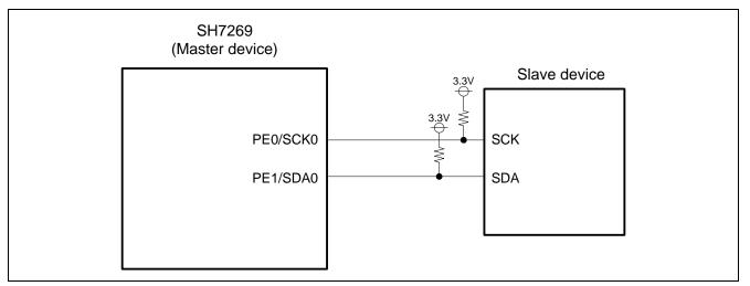
Figure 4.1 Configuration with Slave Device with IIC3
