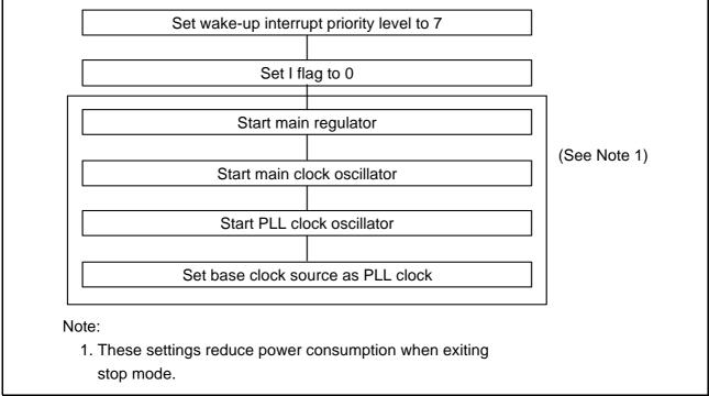
Figure 4.5 Procedure for Exiting Stop Mode
