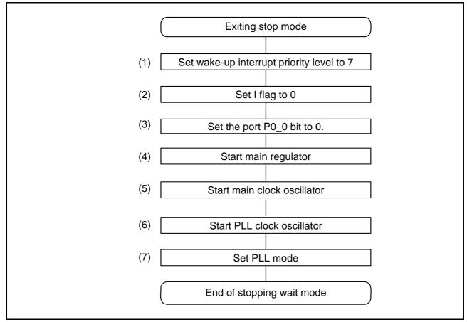
Figure 5.6 Exit Stop Mode Flowchart
