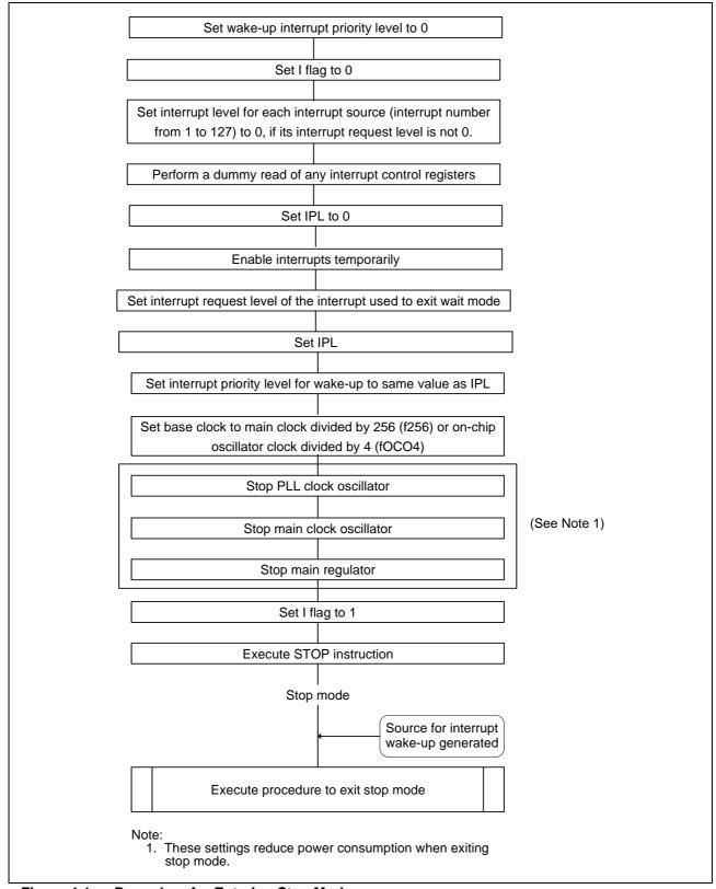
Figure 4.4 Procedure for Entering Stop Mode
