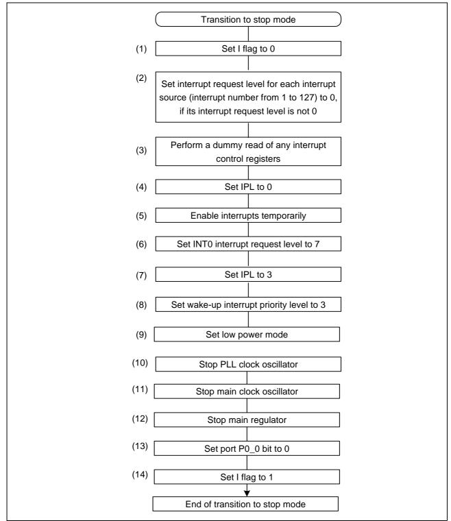
Figure 5.5 Stop Mode Transition Flowchart
