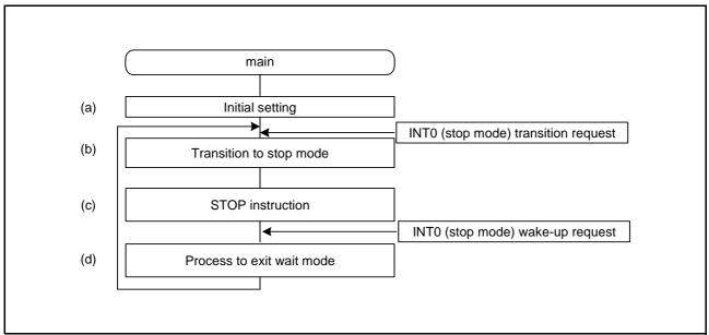
Figure 5.4 Main Function Flowchart
