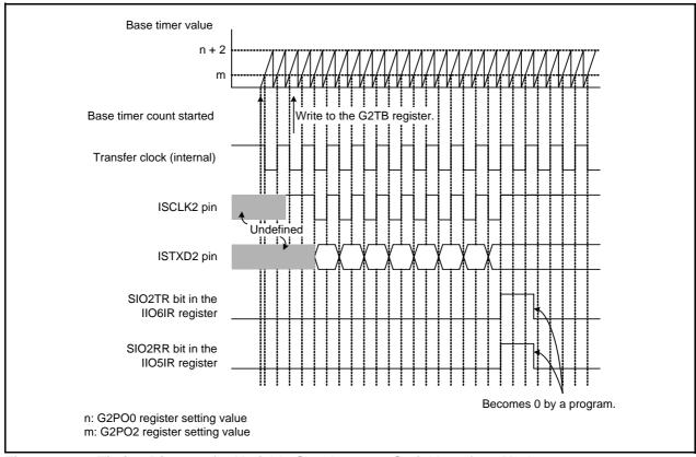
Figure 3.1 Timing Diagram for Variable Synchronous Serial Interface Mode
