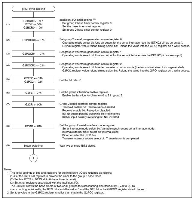
Figure 3.3 Intelligent I/O Initial Setting Function (1/2)
