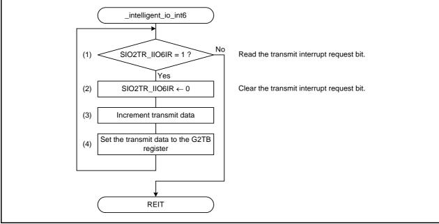
Figure 3.6 Intelligent I/O Interrupt 6
