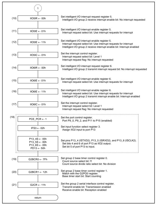
Figure 3.4 Intelligent I/O Initial Setting Function (2/2)
