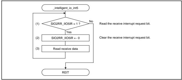
Figure 3.5 Intelligent I/O Interrupt 5
