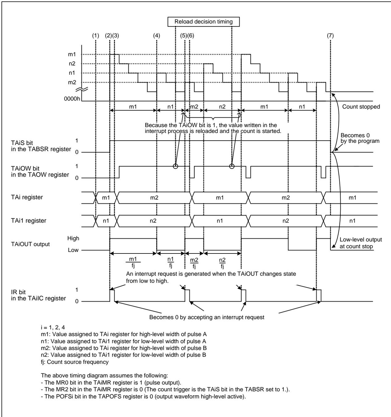
Figure 4.2 Operation Example in Programmable Output Mode
