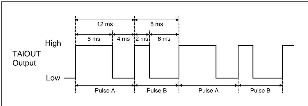
Figure 4.1 Output Waveform of the Sample Program
