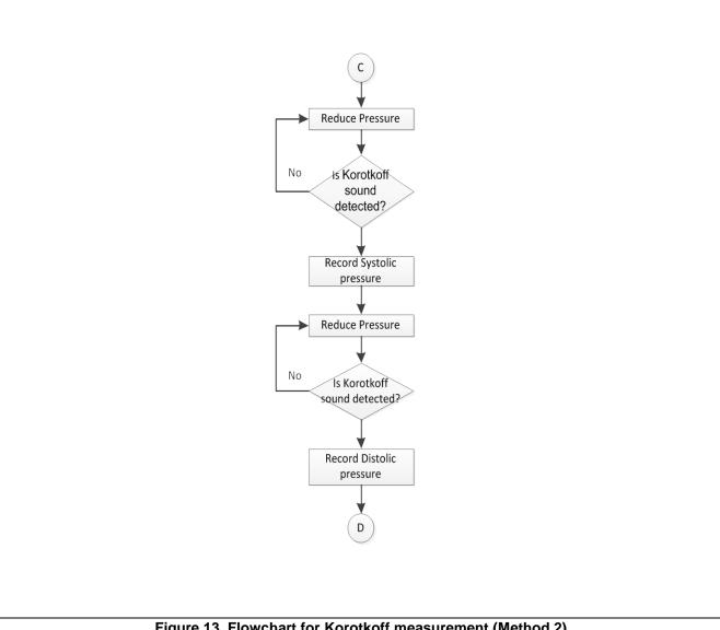
Figure 13 Flowchart for Korotkoff measurement (Method 2)
