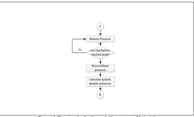
Figure 12 Flowchart for Oscillometric Measurement (Method 1)
