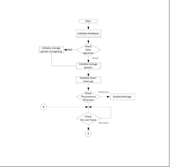
Figure 10 Flowchart for Initialization
