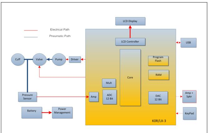
Figure 8 Low cost implementation using 78K0R/Lx3 device
