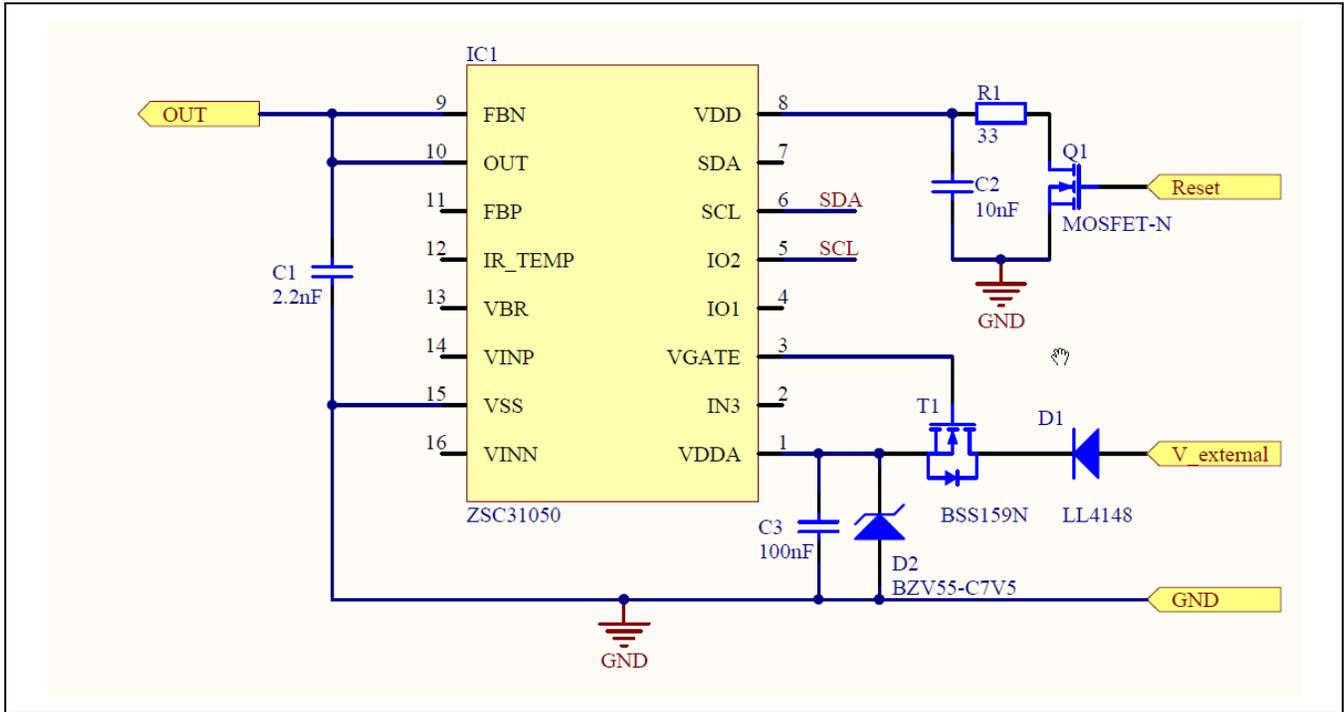
The registers shown in Table 2.1 can be used to set and fine-tune the regulation of the ZSC31050 supply voltage.
