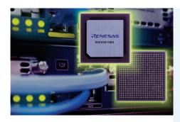
To create the platforms necessary to optimally manage large amounts of network traffic quickly and effectively, system designers are increasingly relying on advanced Ternary Content Addressable Memory (TCAM) devices for performing ultra-fast data packet searches.
