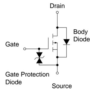
The diode connected between the gate and source of the transistor serves as a protector against ESD. When this device acutally used, an additional protection circiut is externally required if a voltage exceeding the rated voltage may be applied to this device.
