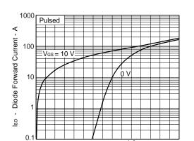
SOURCE TO DRAIN DIODE FORWARD VOLTAGE
