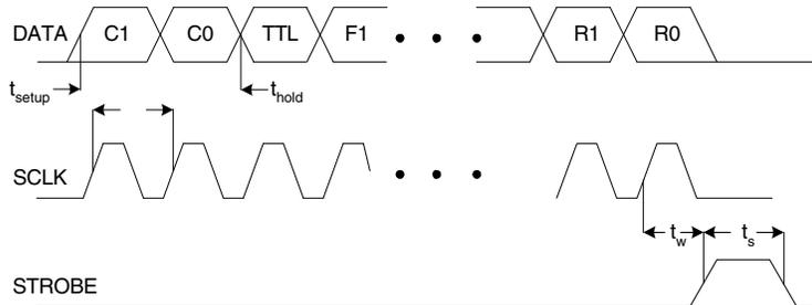
Figure 2. Timing Diagram for Programming the ICS307
