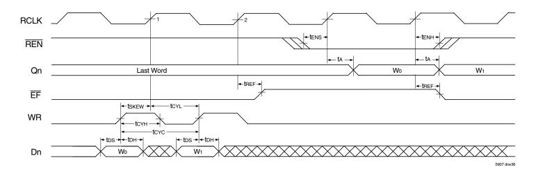
NOTE: 1.  $\overline{\text{OE}}$  = LOW,  $\overline{\text{WEN}}$  = LOW and  $\overline{\text{RCS}}$  = LOW.
