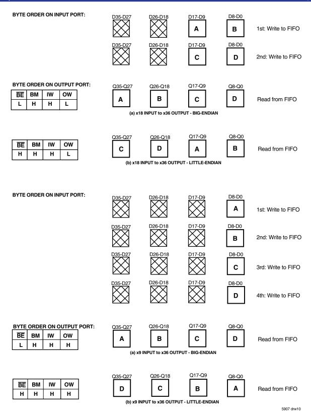
Figure 5. Bus-Matching Byte Arrangement (Continued)
