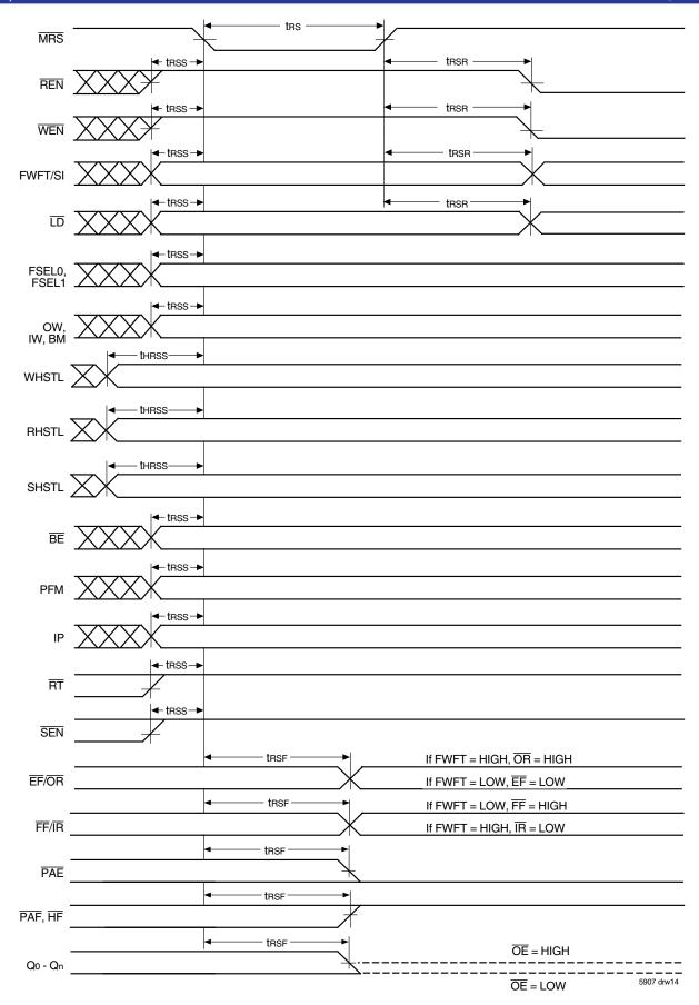
1. During Master Reset the High-Impedance control of the Qn data outputs is provided by  $\overline{\text{OE}}$  only,  $\overline{\text{RCS}}$  can be HIGH or LOW until the first rising edge of RCLK after Master Reset is complete.
