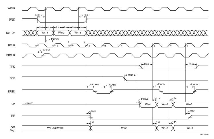
1. The O/P Register is the internal output register. Its contents are available on the Qn output bus only when RCS and OE are both active, LOW, that is the bus is not in High-Impedance state.
