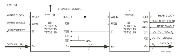
Figure 37. Block Diagram of 131,072 x 36, 262,144 x 36 and 524,288 x 36 Depth Expansion
