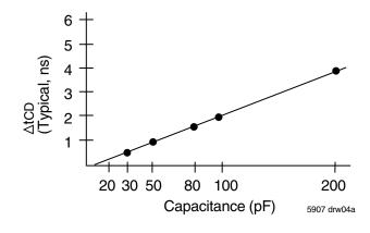
Figure 2b. Lumped Capacitive Load, Typical Derating
