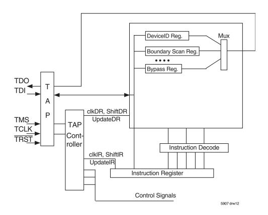
Figure 7. Boundary Scan Architecture
