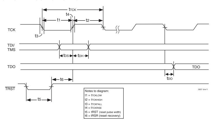
Figure 6. Standard JTAG Timing
