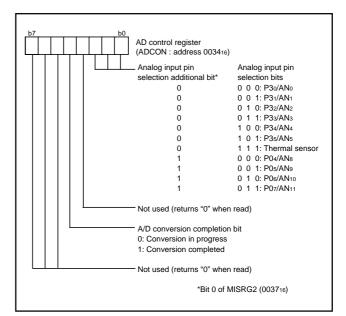
Fig. 44 Structure of AD control register
