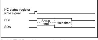
Fig. 33 START condition generating timing diagram
