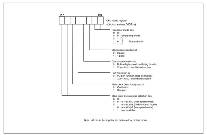
Fig. 6 Structure of CPU mode register
