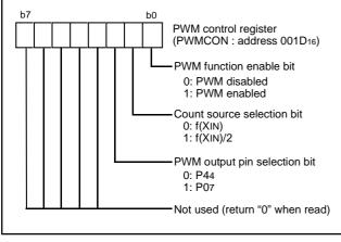
Fig. 42 Structure of PWM control register
