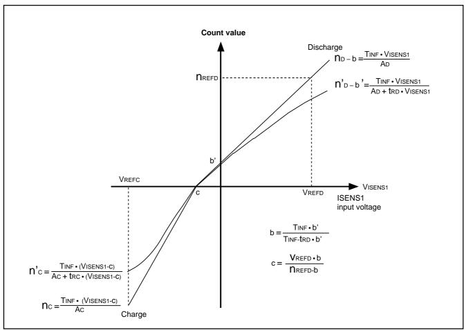
Fig. 80 VISENS1-Count value characteristics of current integrator
