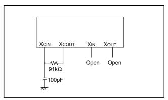
Fig. 64 High-speed RC oscillation circuit and 32kHz RC oscillation circuit
