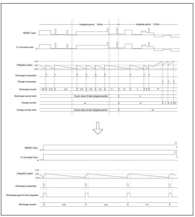
Fig. 48 Current integrator timing diagram
