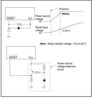
Fig. 56 Reset circuit example
