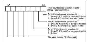
Fig. 15 Structure of timer count source selection register
