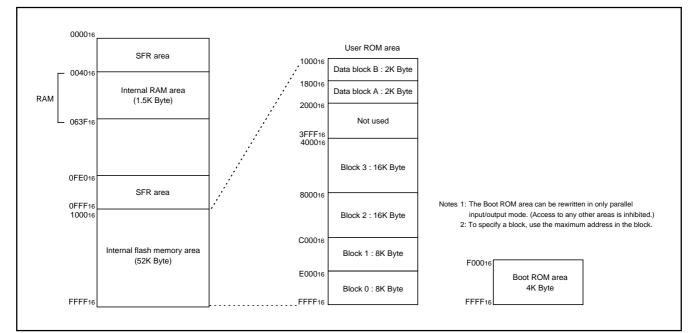
Fig. 68 Block diagram of built-in flash memory (M37512FCHP)
