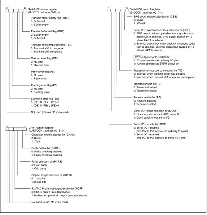
Fig. 21 Structure of serial I/O1 control registers
