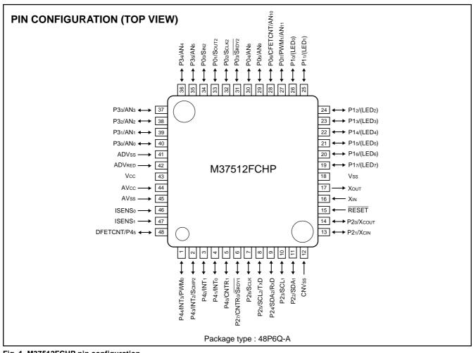
Fig. 1 M37512FCHP pin configuration
