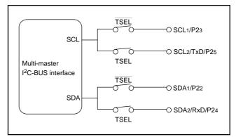
Fig. 29 SDA/SCL pin selection bit
