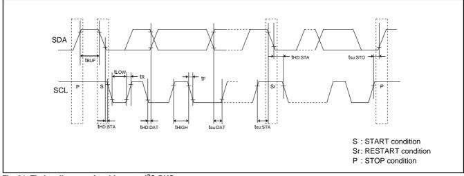
Fig. 81 Timing diagram of multi-master I<sup>2</sup>C-BUS
