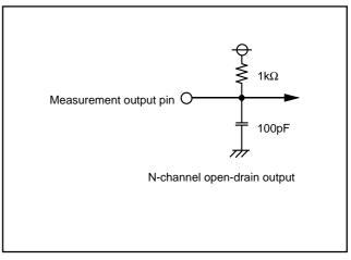
Fig. 82 Circuit for measuring output switching characteristics (1)
