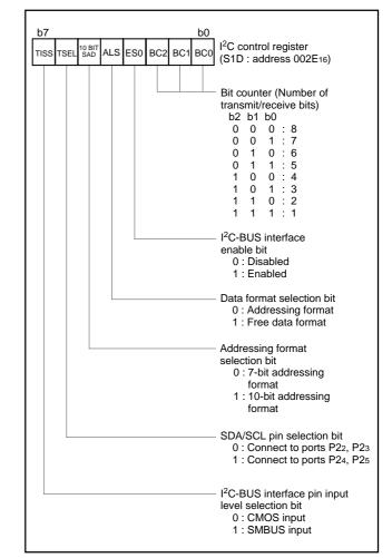
Fig. 30 Structure of I<sup>2</sup>C control register
