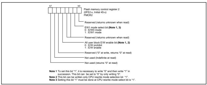
Fig. 71 Structure of flash memory control register 2
