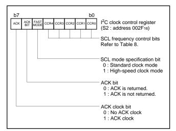
Fig. 28 Structure of I<sup>2</sup>C clock control register
