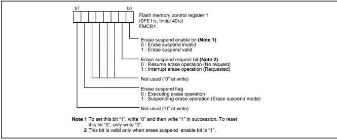
Fig. 70 Structure of flash memory control register 1
