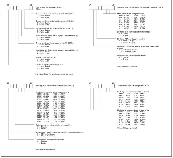
Fig. 52 Over current detector registers (1)
