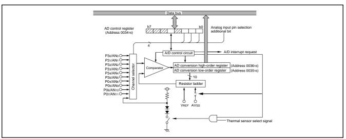
Fig. 46 Block diagram of A/D converter
