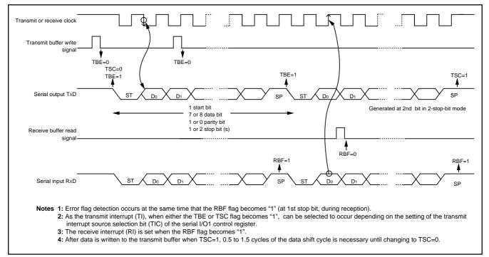
Fig. 20 Operation of UART serial I/O1 function
