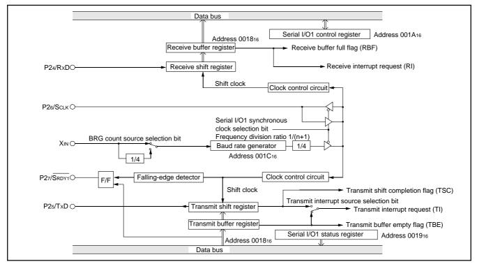
Fig. 17 Block diagram of clock synchronous serial I/O1
