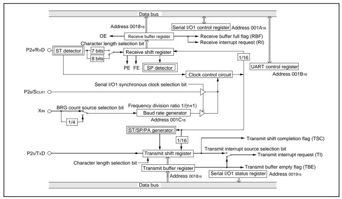
Fig. 19 Block diagram of UART serial I/O1
