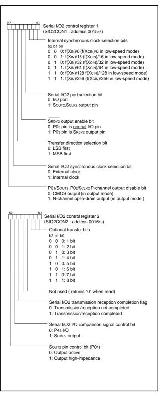
Fig. 22 Structure of Serial I/O2 control registers 1, 2
