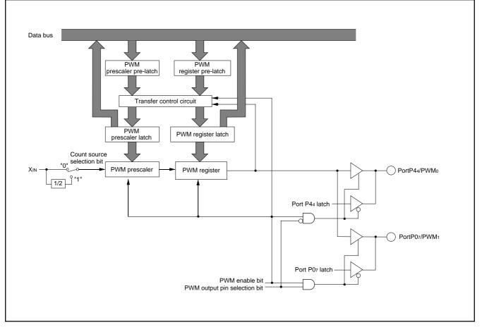
Fig. 41 Block diagram of PWM function
