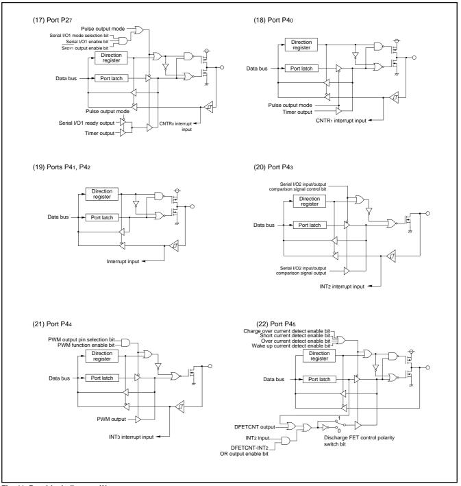
Fig. 11 Port block diagram (3)
