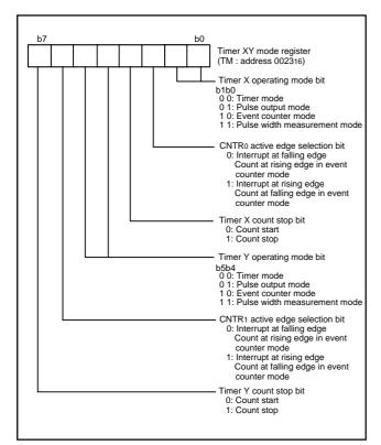
Fig. 14 Structure of timer XY mode register
