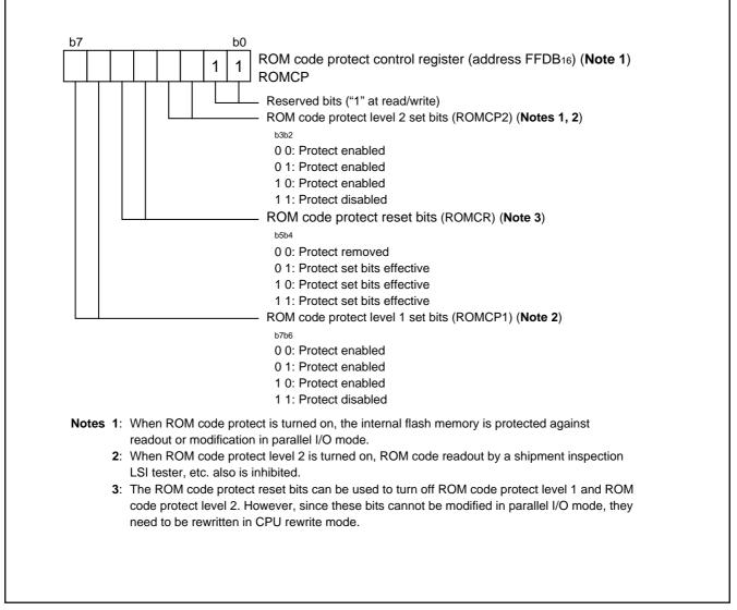
Fig. 76 Structure of ROM code protect control
