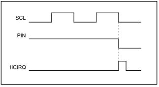
Fig. 32 Interrupt request signal generating timing
