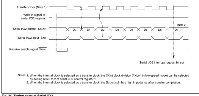
Fig. 24 Timing chart of Serial I/O2
