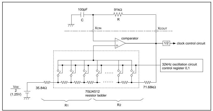
Fig. 59 Block diagram of 32kHz RC oscillation circuit
