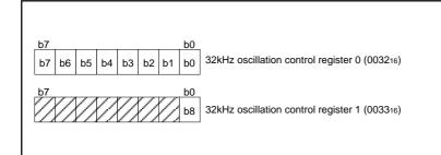
Fig. 60 32kHz oscillation control register
