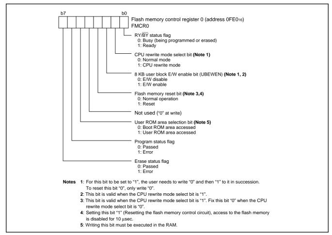
Fig. 69 Structure of flash memory control register
