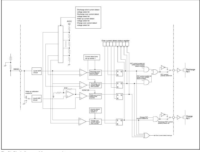
Fig. 51 Block diagram of Over current detector
