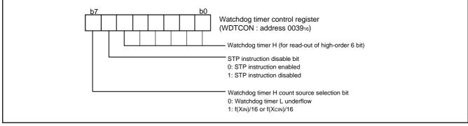
Fig. 55 Structure of Watchdog timer control register
