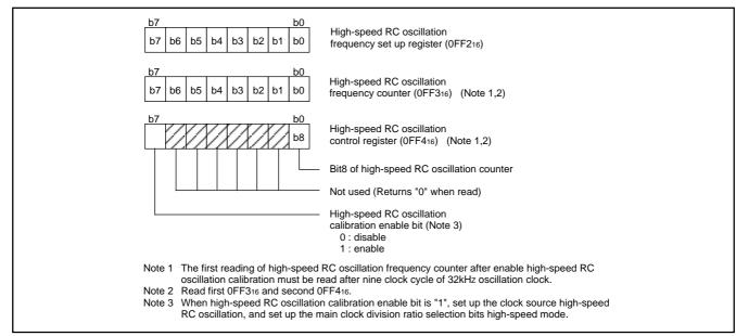
Fig. 61 High-speed RC oscillation register
