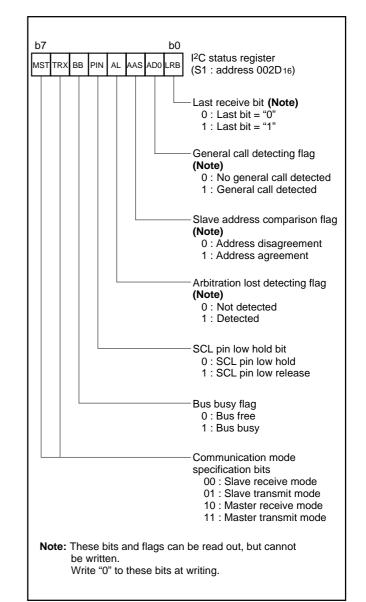
Fig. 31 Structure of I<sup>2</sup>C status register
