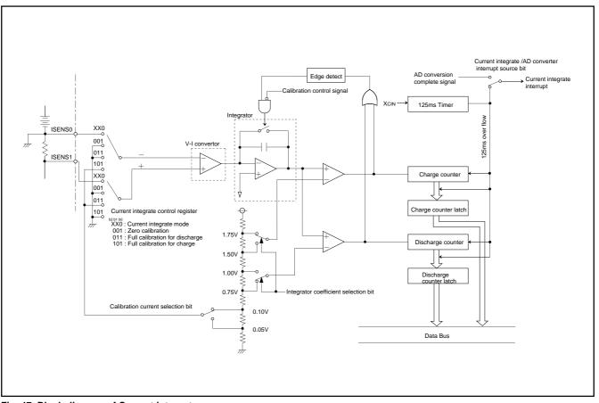
Fig. 47 Block diagram of Current integrator
