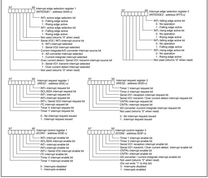
Fig. 13 Structure of interrupt-related registers
