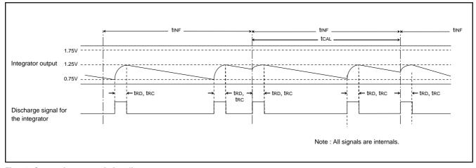
Fig. 79 Current integrator timing diagram
