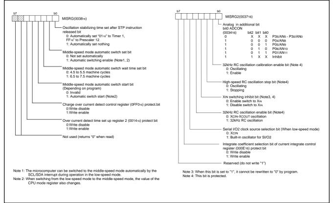
Fig. 66 Structure of MISRG1, MISRG2
