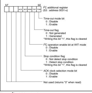
Fig. 38 I<sup>2</sup>C additional register
