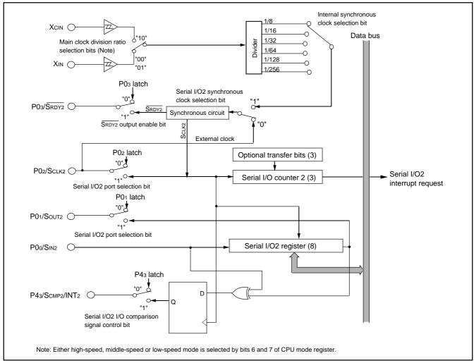
Fig. 23 Block diagram of Serial I/O2
