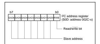
Fig. 27 Structure of I<sup>2</sup>C address register
