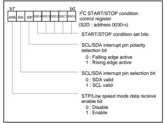
Fig. 37 Structure of I<sup>2</sup>C START/STOP condition control register
