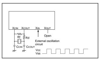
Fig. 63 External clock input circuit
