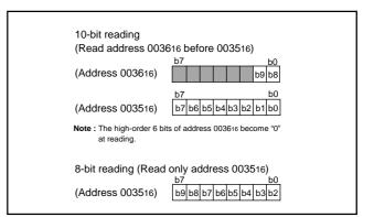
Fig. 45 Structure of AD conversion registers
