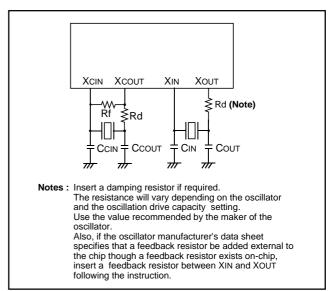
Fig. 62 Ceramic resonator circuit
