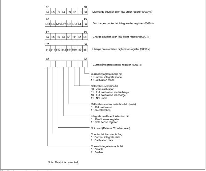
Fig. 50 Current integrator registers
