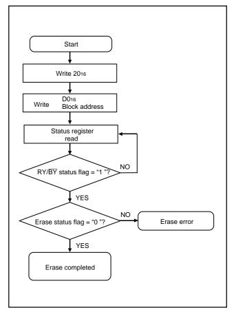
Fig. 74 Erase flowchart in no erase suspend
