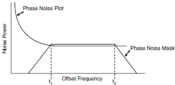
$$RMS\ Jitter = \sqrt{\text{Area Under the Masked Phase Noise Plot}}$$
