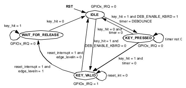
Figure 63: GPIO Interrupt Generator State Machine
