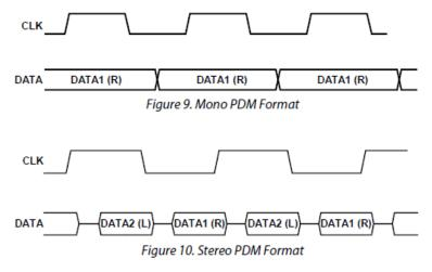
Figure 72: PDM Mono/Stereo Formats
