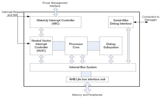
Figure 16: ARM Cortex-M0 Block Diagram
