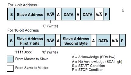
Figure 34: Master-Transmitter Protocol
