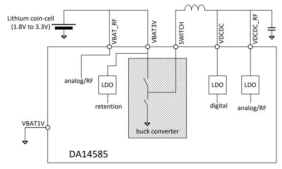
Figure 75: Supply Overview, Coin-Cell Application
