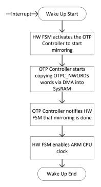
Figure 11: Wake-Up OTP Mirroring
