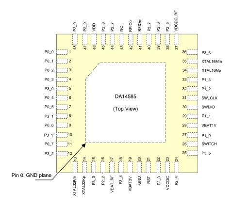
Figure 5: QFN48 Pin Assignment
