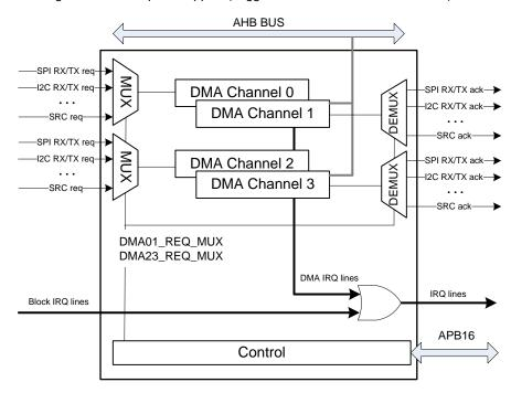
Figure 26: DMA Controller Block Diagram
