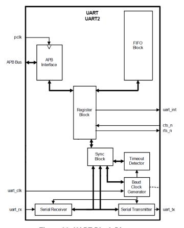
Figure 39: UART Block Diagram
