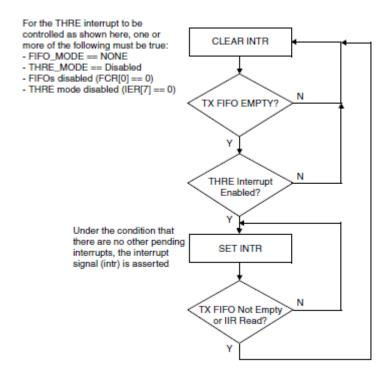
Figure 44: Flowchart of Interrupt Generation when not in Programmable THRE Interrupt Mode
