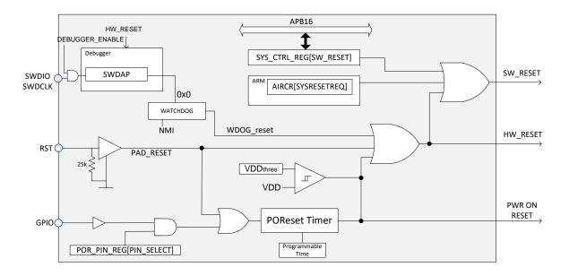
Figure 14: Reset Block Diagram
