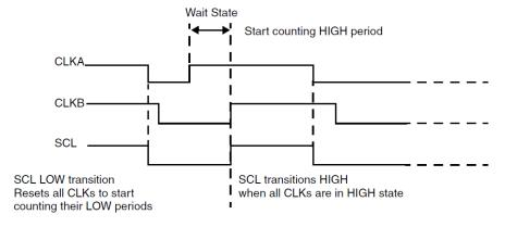
Figure 38: Multiple Master Clock Synchronization
