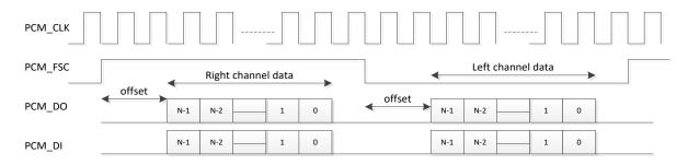
Figure 70: I2S TDM Mode (Left Justified Mode)
