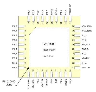
Figure 4: QFN40 Pin Assignment
