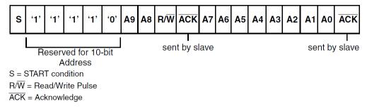
Figure 33: 10-bit Address Format
