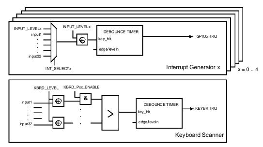
Figure 61: Keyboard Controller Block Diagram
