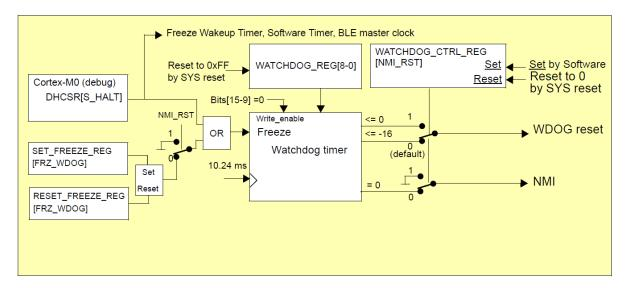
Figure 60: Watchdog Timer Block Diagram
