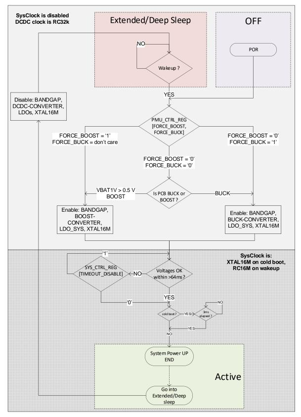
Figure 10: Power/Wake-Up Sequence
