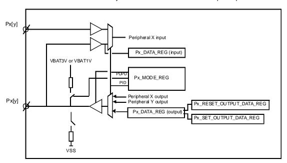
Figure 64: Port P0, P1, P2, and P3 with Programmable Pin Assignment
