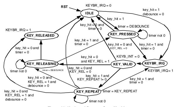
Figure 62: Keyboard Scanner State Machine
