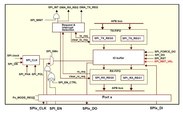
Figure 45: SPI Block Diagram
