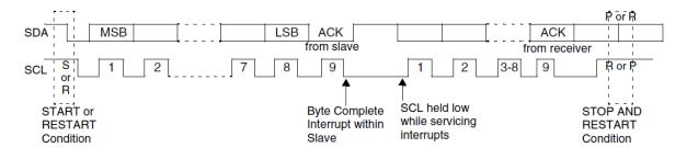
Figure 30: Data Transfer on the I2C Bus
