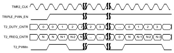
Figure 59: Timer 2 PWM Timing Diagram
