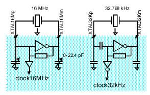
Figure 21: Crystal Oscillator Circuits
