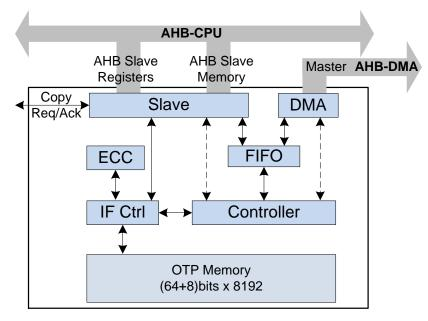
Figure 24: OTP Controller Block Diagram
