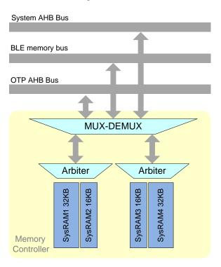
Figure 19: Memory Controller Block Diagram
