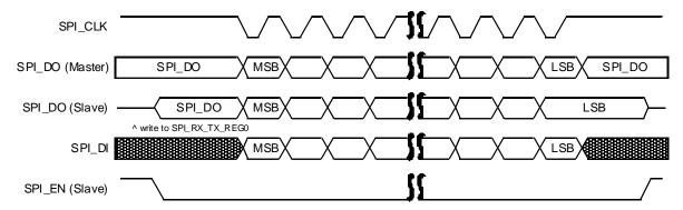
Figure 49: SPI Master/slave, Mode 3: SPI\_POL=1 and SPI\_PHA=1
