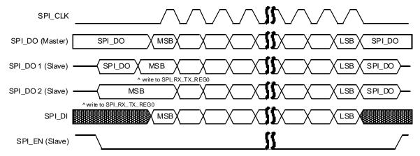
Figure 46: SPI Master/Slave, Mode 0: SPI\_POL=0 and SPI\_PHA=0
