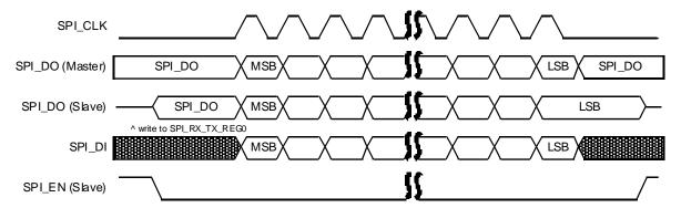
Figure 47: SPI Master/Slave, Mode 1: SPI POL=0 and SPI PHA=1
