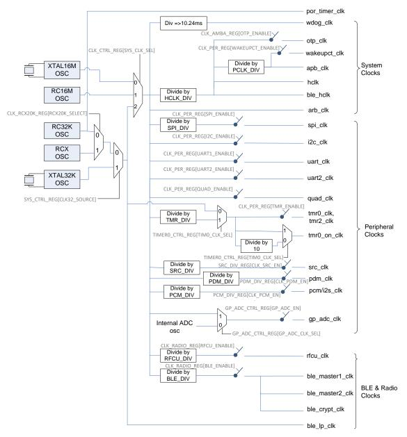
Figure 23: Clock Generation Block Diagram
