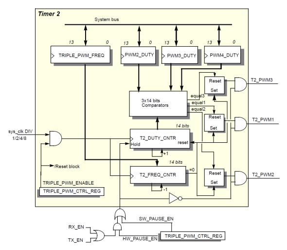
Figure 58: Timer 2 PWM Block Diagram
