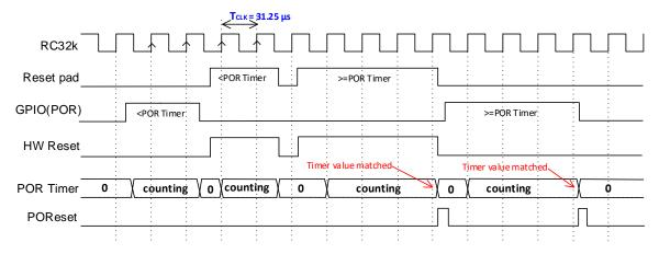
Figure 15: Power-On Reset Timing Diagram
