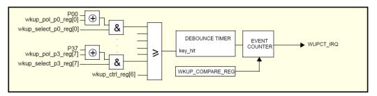
Figure 54: Wake-Up Timer Block Diagram
