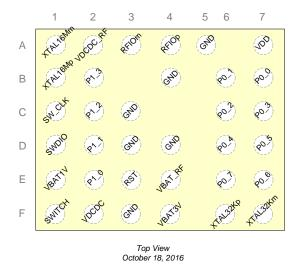
Figure 3: WLCSP34 Ball Assignment (Top View)
