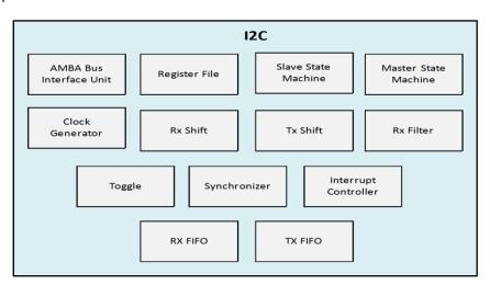
Figure 28: I2C Controller Block Diagram
