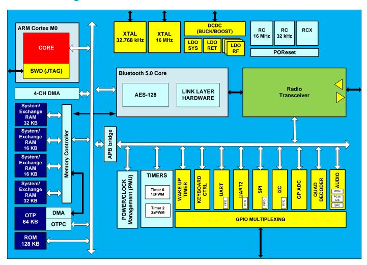
Figure 2: DA14585 Block Diagram
