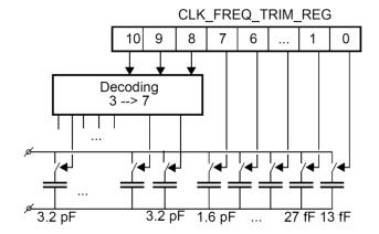
Figure 22: 16 MHz Crystal Oscillator Frequency Trimming
