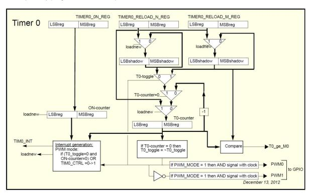
Figure 56: Timer 0 Block Diagram
