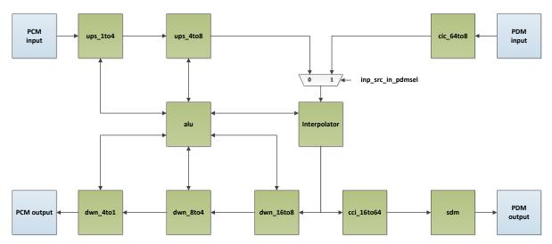
Figure 67: Audio Unit Up/Down Sampler Block Diagram
