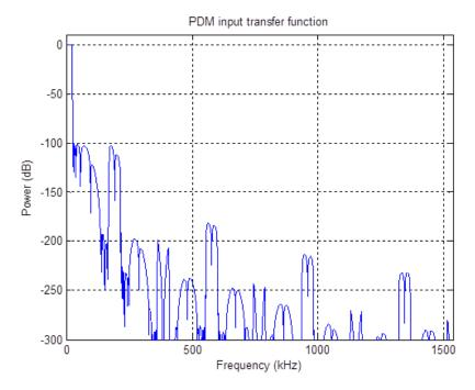
Figure 73: SRC PDM Input Transfer Function
