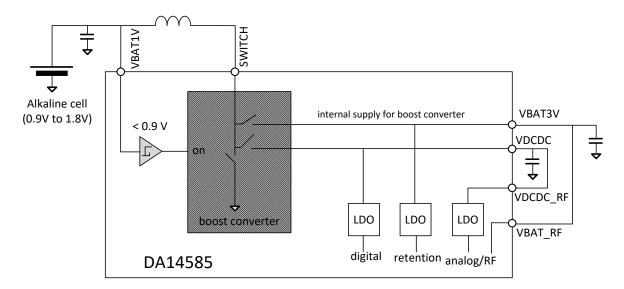
Figure 76: Supply Overview, Alkaline-Cell Application
