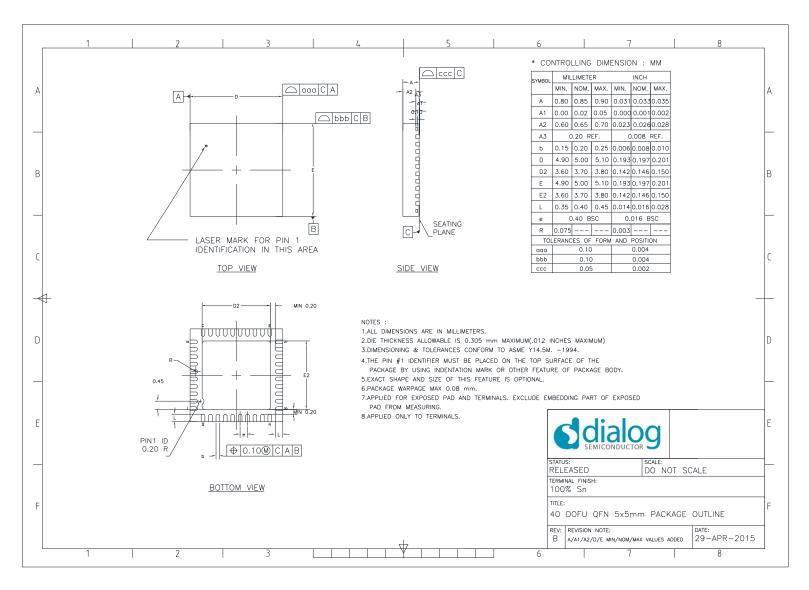
Figure 86: QFN40 Package Outline Drawing
