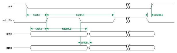
Figure 50: SPI Slave Mode Timing (CPOL = 0, CPHA = 0)
