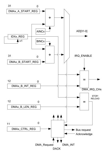
Figure 27: DMA Channel Diagram
