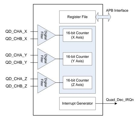
Figure 51: Quadrature Decoder Block Diagram
