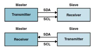
Figure 29: Master/Slave and Transmitter/Receiver Relationships
