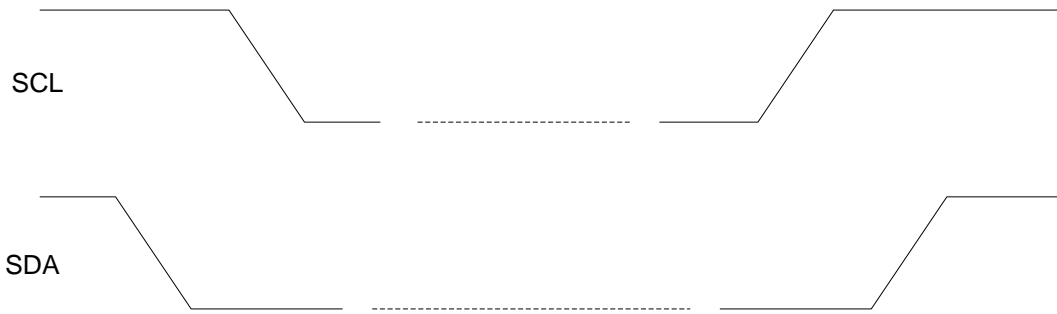
Figure 16: I 2 C START and STOP Condition Timing
