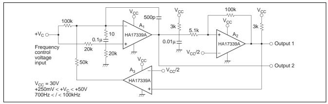
Figure 5 Voltage Controlled Oscillator
