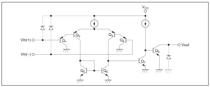
Note: If Input/Output terminals voltage over the absolute maximum ratings, there is possibility of mis-operation, characteristics deterioration and destruction, because of the current's flowing to parasitic diode in IC. The Input/Output terminals are recommended to be protected with the clamp circuit which using the diode with low forward voltage (like schottky barrier diode) when there is a possibility for the Input/Output terminals voltage exceeds the absolute maximum ratings.
