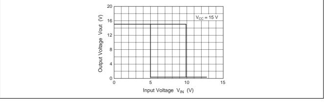
Figure 10 Inverting Comparator I/O Transfer Characteristics
