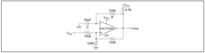
Figure 1 Square-Wave Oscillator
