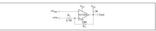
Figure 7 Noninverting Comparator
