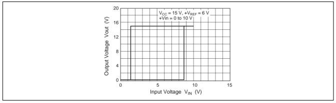
Figure 8 Noninverting Comparator I/O Transfer Characteristics
