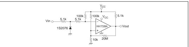
Figure 11 Zero-Cross Detector
