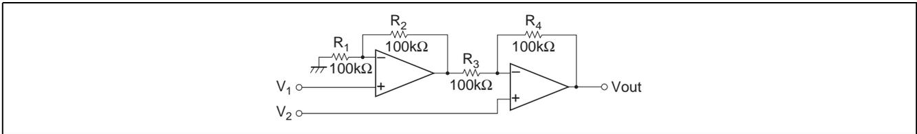
Figure 3 High Input Impedance DC Differential Amplifier
