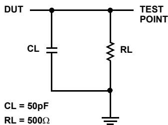
**Three-State Low Timing Diagram**
