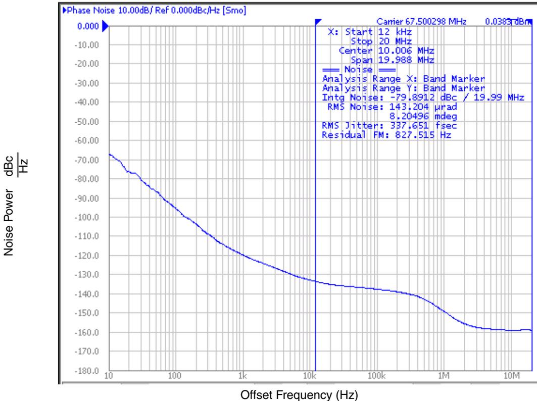
Typical Phase Noise at 74.25MHz @ (3.3V core, 3.3V output)
