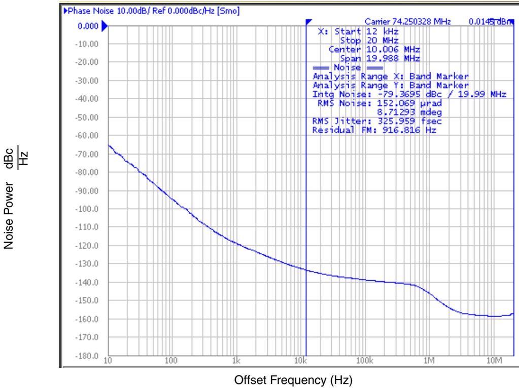
Typical Phase Noise at 148.5MHz (3.3V core, 3.3V output)
