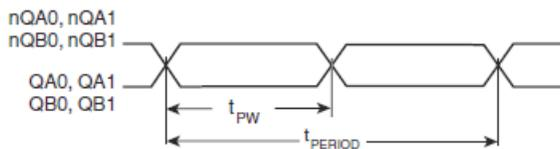
$$\text{odc} = \frac{t_{PW}}{t_{PERIOD}} \times 100\%$$
