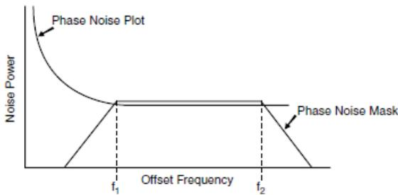
$$\text{RMS Jitter} = \sqrt{\text{Area Under the Masked Phase Noise Plot}}$$
