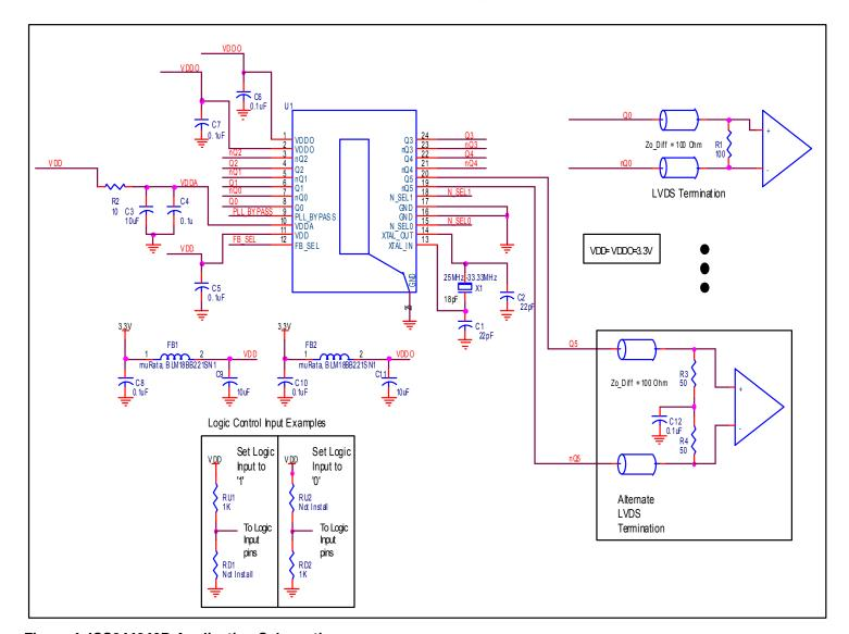
Figure 4. ICS844246D Application Schematic
