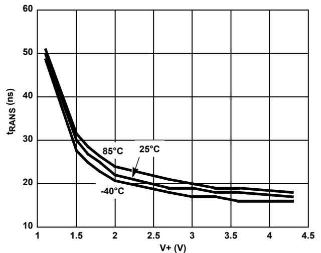
FIGURE 14. ADDRESS TRANS TIME vs SUPPLY VOLTAGE
