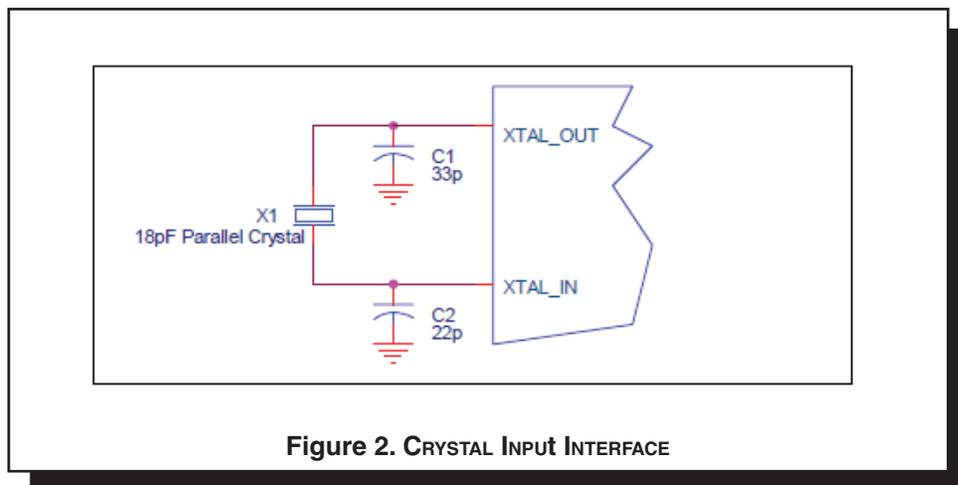
Figure 2. CRYSTAL INPUT INTERFACE
