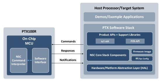
Figure 9: PTX100R SW Stack Integration View
