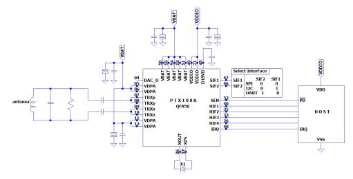
Figure 10: Exemplary Reference Schematic
