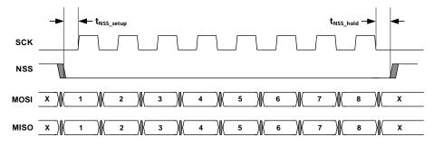
Figure 8: SPI mode 0 (CPOL, CPHA = 0)
