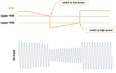
Figure 7: Dynamic Digital Power Control (DDPC)
