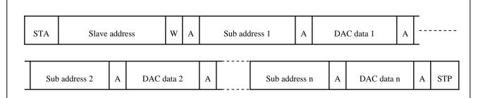
Note: After START condition, the master IC (MCU etc.) accesses the slave IC by slave address, and transmits the data to each channel by two bytes (sub address and DAC data).
