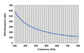
Figure 24. Switching Frequency versus FS Resistance
