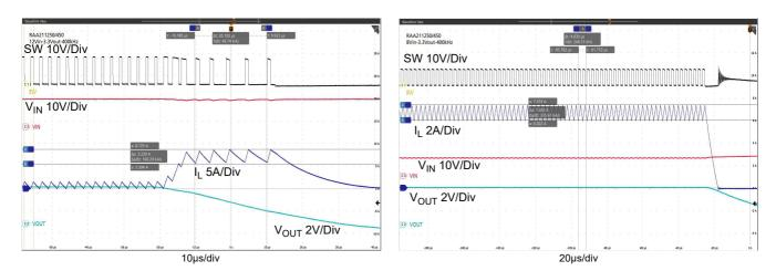
Figure 25. Short Output Protection, High-Side OC Protection
