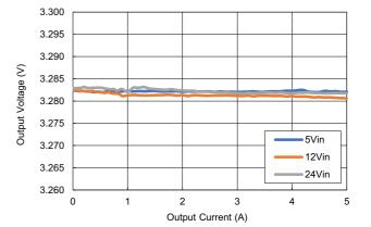
Figure 5. Load Regulation, 3.3V  $V_{OUT}$ , 400kHz, QFN
