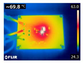
Figure 22. Thermal Image, 12V $_{\rm IN}$ , 3.3V $_{\rm OUT}$ , 400kHz, 5A, HTSSOP, T $_{\rm J}$  = 69.8°C
