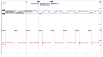
Figure 9. External SS,  $12V_{IN}$ ,  $3.3V_{OUT}$ ,  $0.65\Omega$  Load,  $C_{SS}$  = 39nF, HTSSOP
