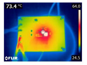
Figure 21. Thermal Image,  $24V_{IN}$ ,  $3.3V_{OUT}$ , 400kHz, 5A, QFN,  $T_J$  =  $73.4^{\circ}C$
