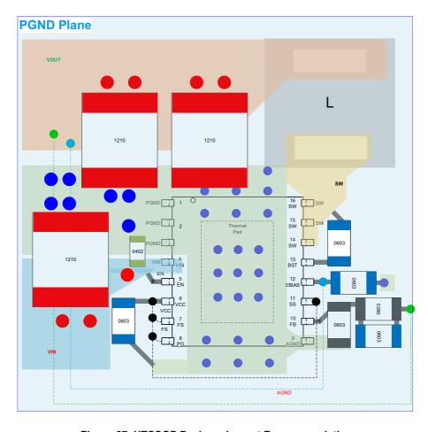
Figure 27. HTSSOP Package Layout Recommendation
