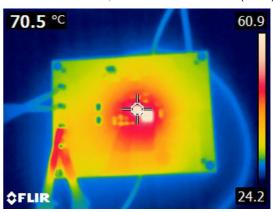
Figure 20. Thermal Image, 12V  $_{\mbox{IN}},\,3.3V_{\mbox{OUT}},\,400\mbox{kHz},\,5\mbox{A},\\ \mbox{QFN},\,T_{\mbox{J}}=70.5^{\circ}\mbox{C}$
