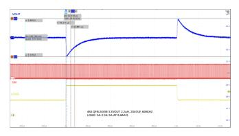
Figure 13. Load Transient,  $24V_{IN}$ ,  $3.3V_{OUT}$ , 600kHz, 2.5A to 5A, QFN
