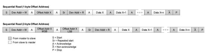
Figure 21. I<sup>2</sup>C Master Sequencing
