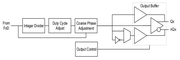
Figure 15. Single Output Stage
