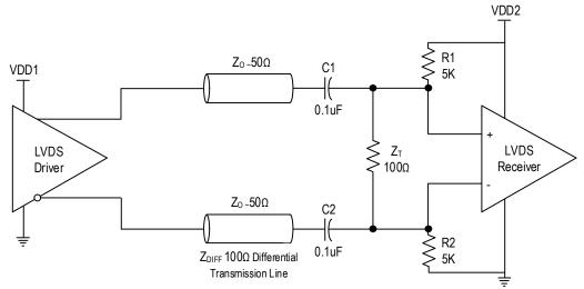
Figure 43. AC Coupled LVDS Termination
