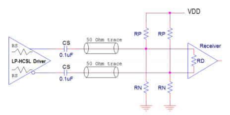
Figure 46. AC-Coupling Termination
