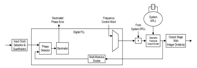
Figure 26. Jitter Attenuator Operation with External Digital Loop Filter
