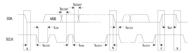
Figure 20. I<sup>2</sup>C Slave Timing Diagram
