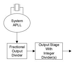
Figure 22. Free-Running Synthesizer Operation
