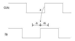
a = Trace delay from Qy to the CLK input used for external feedback
