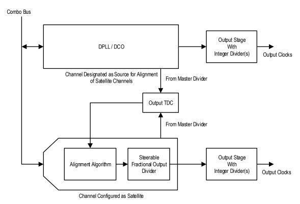
Figure 32. Satellite Channel and Source Channel
