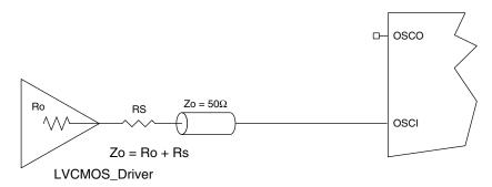
Figure 39. 1.8V LVCMOS Driver to XTAL Input Interface
