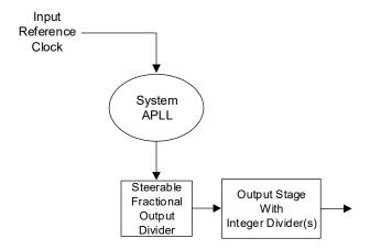
Figure 23. Clock Generator Operation
