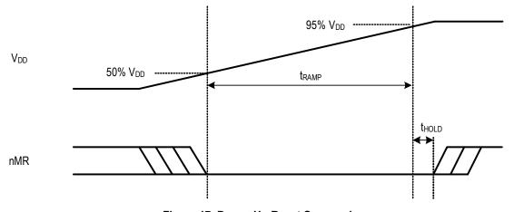
Figure 17. Power-Up Reset Sequencing
