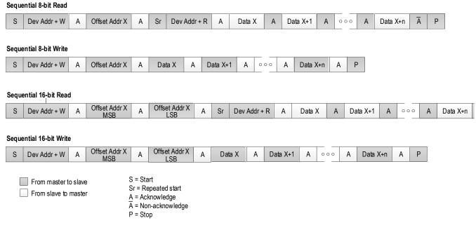
Figure 19. I<sup>2</sup>C Slave Sequencing
