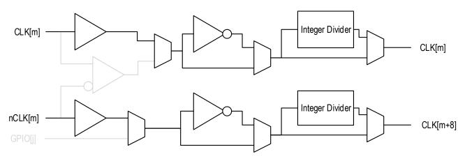
Figure 7. Input Stage Configured as Dual Single-Ended
