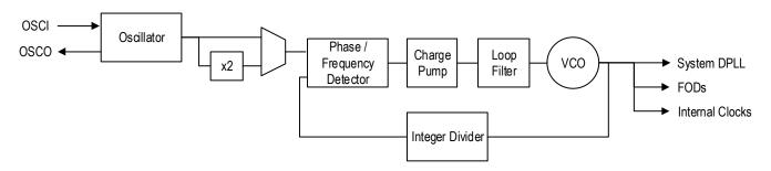
Figure 5. System Analog PLL Channel
