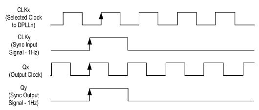
Figure 10. Sync Pulse Operation
