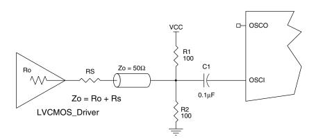
Figure 40. LVCMOS Driver to XTAL Input Interface
