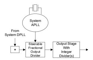
Figure 24. Synthesizer Disciplined with Oscillator Operation
