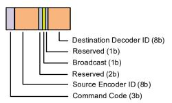
Figure 37. PWM Frame Header
