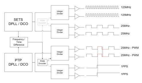
Figure 35. PWM Signature - 1PPS Encoding Example
