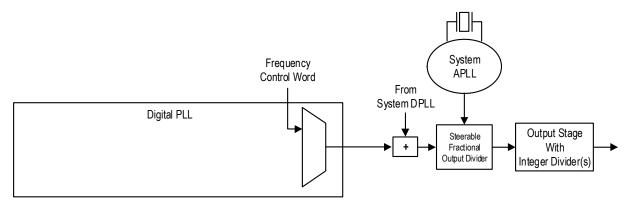
Figure 28. External DCO Control via Frequency Control Word
