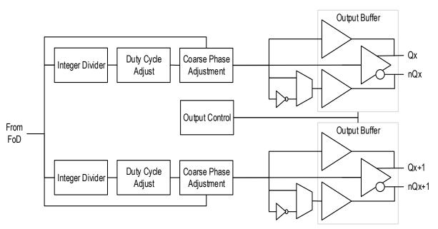
Figure 16. Dual Output Stage
