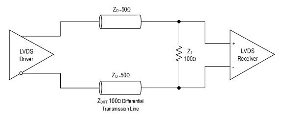
Figure 42. Standard LVDS Termination
