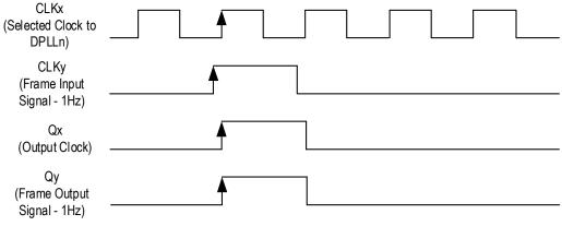
Figure 9. Frame Pulse Operation
