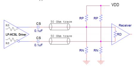
Figure 45. AC-Coupling Termination
