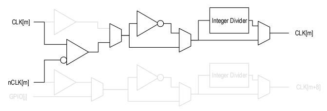
Figure 6. Input Stage Configured as Differential Only
