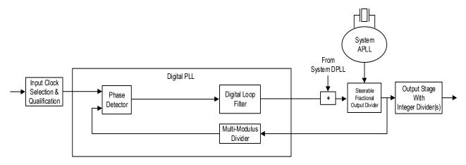
Figure 27. Jitter Attenuator Disciplined with Oscillator Operation
