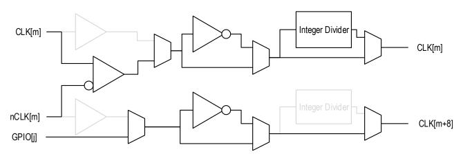
Figure 8. Input Stage Configured as Differential Plus Single Single-Ended
