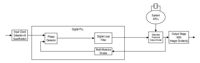
Figure 25. Jitter Attenuator Operation
