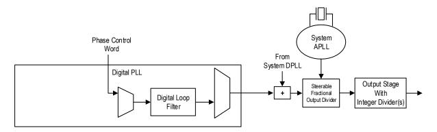
Figure 29. External DCO Control via Phase Control Word
