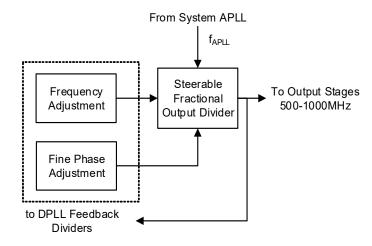
Figure 14. Steerable Fractional Output Divider Block
