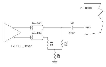
Figure 41. LVPECL Driver to XTAL Input Interface
