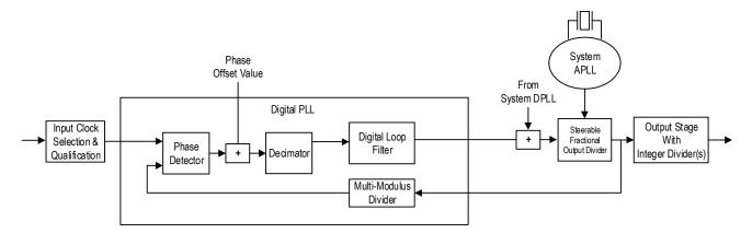
Figure 30. Phase Control in Closed Loop Operation
