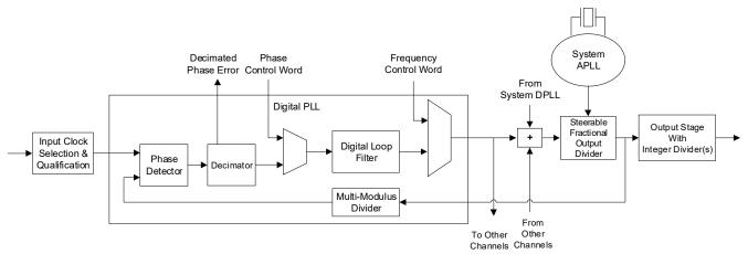
Figure 2. Single PLL Channel
