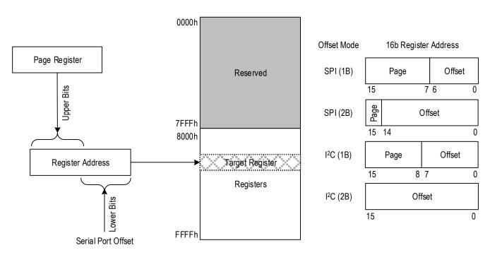
Figure 18. Register Addressing Modes via Serial Port
