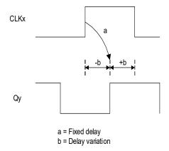
Figure 3. Input-Output Delay with Internal Feedback
