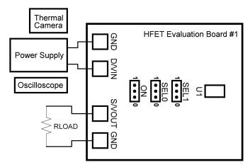
Figure 11. SLG59H1009V Evaluation Board Connection Circuit
