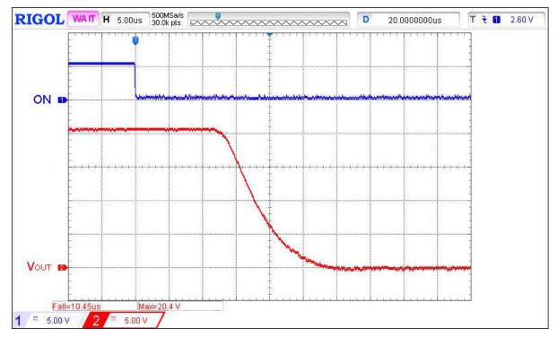
Figure 4. Typical Turn OFF operation waveform for V<sub>IN</sub> = 20 V, C<sub>SLEW</sub> = 10 nF, no C<sub>LOAD</sub> , R<sub>LOAD</sub> = 100  $\Omega$
