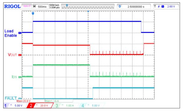
Figure 6. Thermally induced SOA shutdown for  $V_{IN}$  = 20 V,  $C_{LOAD}$  = 10  $\mu$ F,  $I_{ACL}$  = 1 A,  $R_{SET}$  = 91  $k\Omega$
