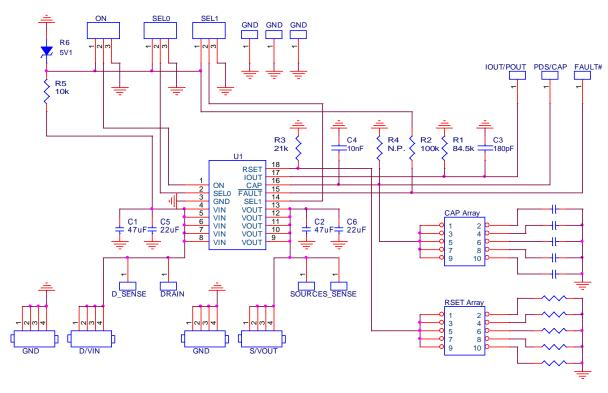
Figure 10. SLG59H1009V Evaluation Board Connection Circuit
