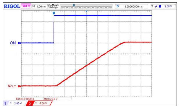
Figure 2. Typical Turn ON operation waveform for V<sub>IN</sub> = 20 V,  $C_{SLEW}$  = 10 nF,  $C_{LOAD}$  = 10  $\mu$ F,  $R_{LOAD}$  = 100  $\Omega$
