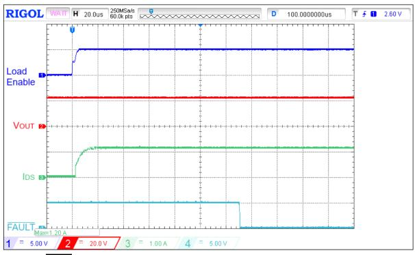
Figure 7. Typical  $\overline{FAULT}$  assertion waveform for  $V_{IN}$  = 20 V,  $C_{LOAD}$  = 10  $\mu$ F,  $I_{ACL}$  = 1 A,  $R_{SET}$  = 91  $k\Omega$ , switch in 20  $\Omega$  load
