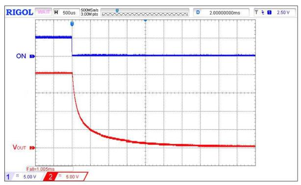
Figure 5. Typical Turn OFF operation waveform for  $V_{IN}$  = 20 V,  $C_{SLEW}$  = 10 nF,  $C_{LOAD}$  = 10  $\mu$ F,  $R_{LOAD}$  = 100  $\Omega$  Typical SOA Waveforms
