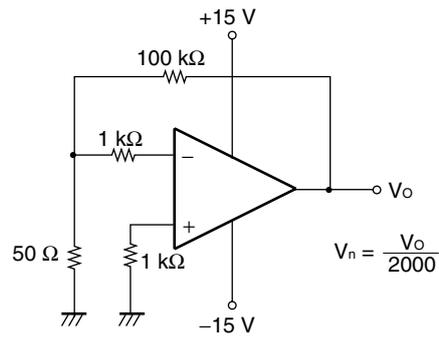
Figure2 Channel Separation Measurement Circuit
