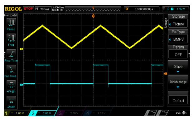
Figure 7: ACMP Output during Glitching
