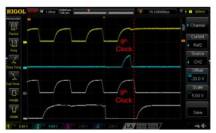
Figure 3: Non-I<sup>2</sup>C Compliant Behavior Oscillogram
