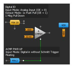
Figure 4: GreenPAK Input Structure Test Schematic
