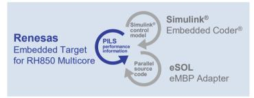
Embedded Target for RH850 Multicore is a MATLAB® collaborative environment that automatically generates parallel codes and a Processor In the Loop Simulation (PILS) environment from a Simulink® model. This development environment also supports automatic multicore allocation in corporation with the model based parallelizer of eSOL Co., Ltd.
