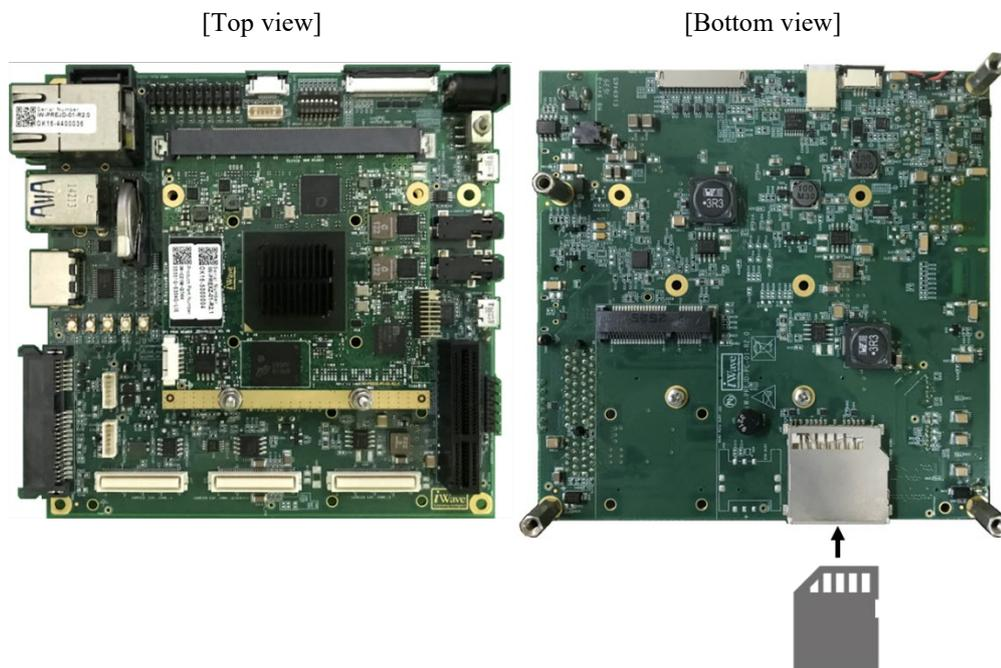
Figure 6. Set SD card to carry board
