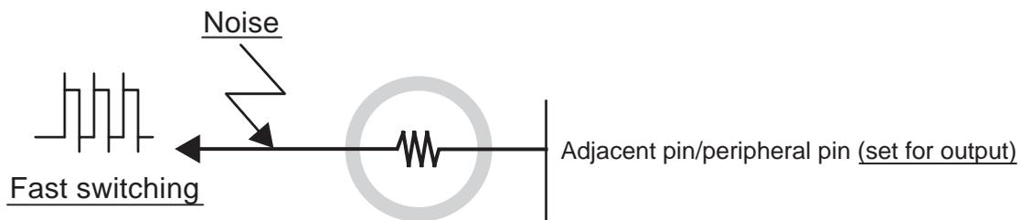
Method for limiting switching noise with a resistor
