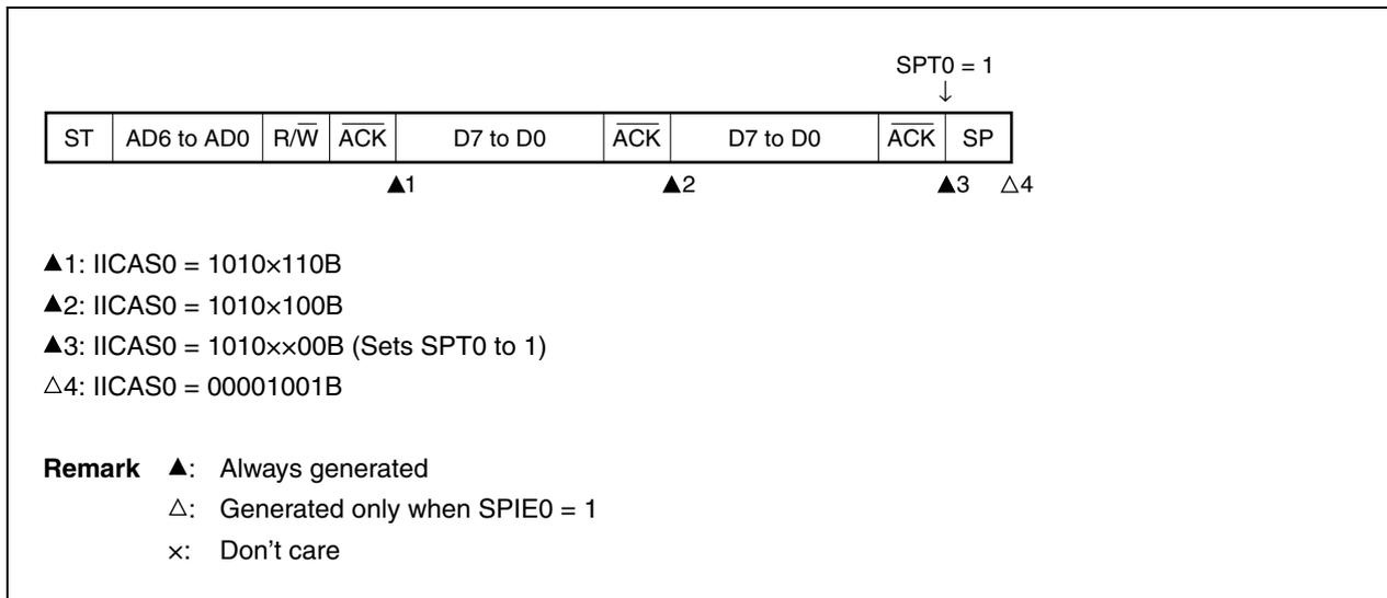
**(2) Slave device operation (slave address data reception)****(a) Start ~ Address ~ Data ~ Data ~ Stop****(i) When WTIM0 = 0**
