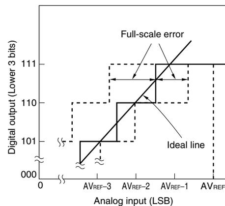
**Figure 12-20. Integral Linearity Error**
