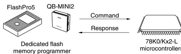
The flash memory control commands of the 78K0/Kx2-L microcontrollers are listed in the table below. All these commands are issued from the programmer and the 78K0/Kx2-L microcontrollers perform processing corresponding to the respective commands.
