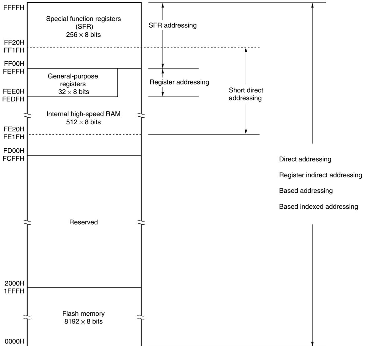
**Figure 3-7. Correspondence Between Data Memory and Addressing**
