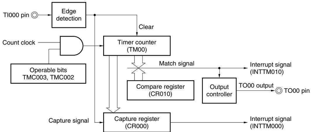
**Figure 6-28. Timing Example of Clear & Start Mode Entered by TI000 Pin Valid Edge Input
