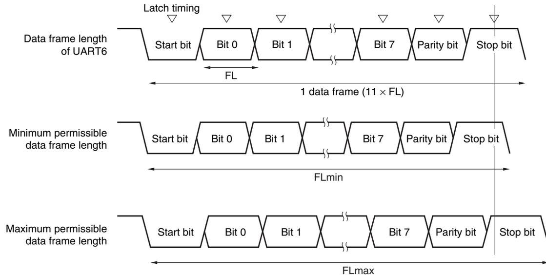
As shown in Figure 14-27, the latch timing of the receive data is determined by the counter set by baud rate generator control register 6 (BRGC6) after the start bit has been detected. If the last data (stop bit) meets this latch timing, the data can be correctly received.
