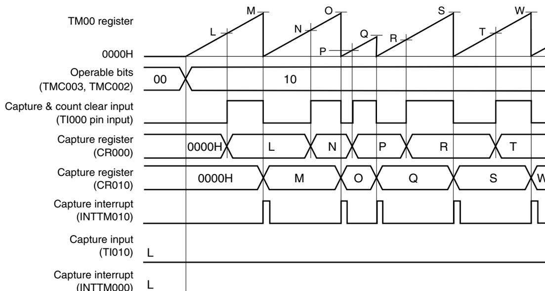
This is an application example where the pulse width of the signal input to the TI000 pin is measured. By setting CRC00, the count value can be captured to CR000 in the phase reverse to the falling edge of the TI000 pin (i.e., rising edge) and to CR010 at the falling edge of the TI000 pin. The high- and low-level widths of the input pulse can be calculated by the following expressions.
