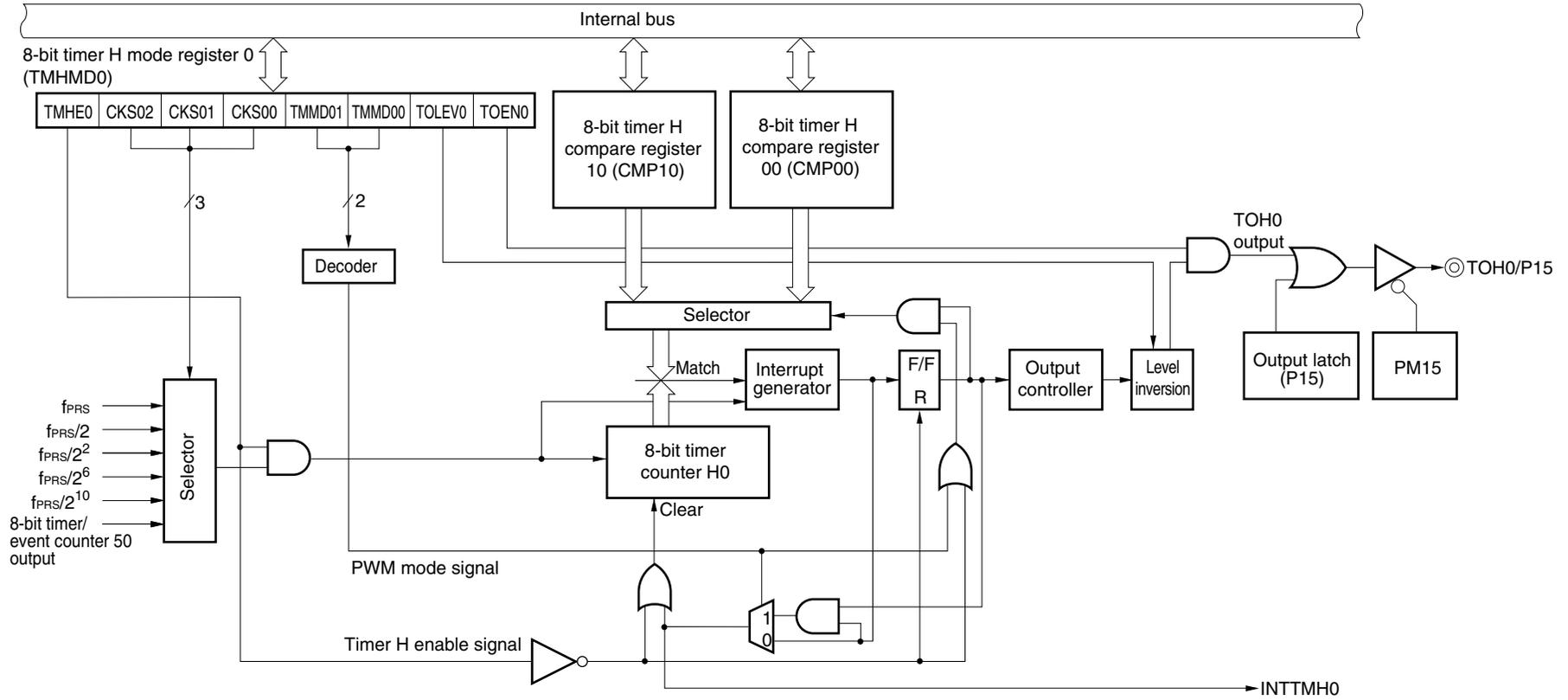
Figure 8-2. Block Diagram of 8-Bit Timer H1
