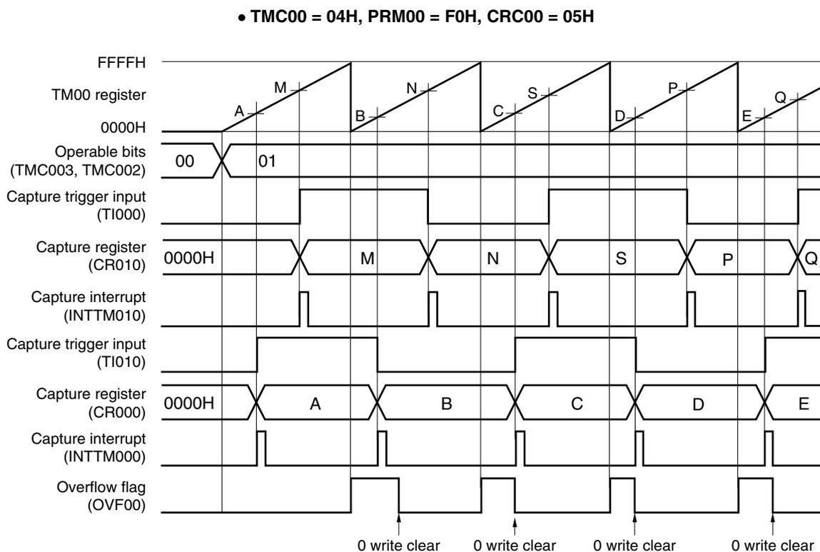
**(2) Measuring the pulse width by using one input signal of the TI000 pin (free-running timer mode)**
