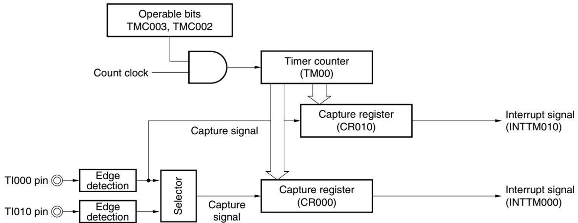
**Remark** If both CR000 and CR010 are used as capture registers in the free-running timer mode, the TO00 output level is not inverted.
