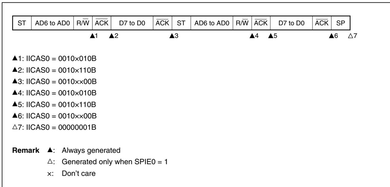
**(d) Start ~ Code ~ Data ~ Start ~ Address ~ Data ~ Stop****(i) When WTIM0 = 0 (after restart, does not match address (= not extension code))**
