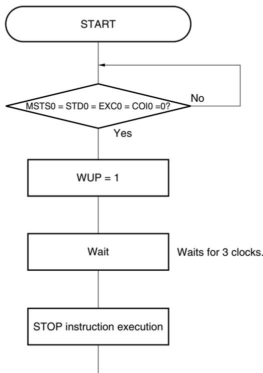
Figure 15-24. Flow When Setting WUP = 0 upon Address Match (Including Extension Code Reception)
