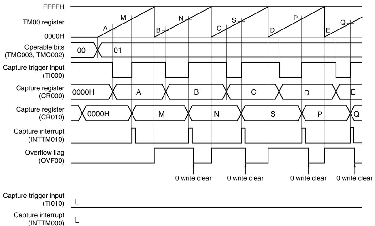
**(3) Measuring the pulse width by using one input signal of the TI000 pin (clear & start mode entered by the TI000 pin valid edge input)**
