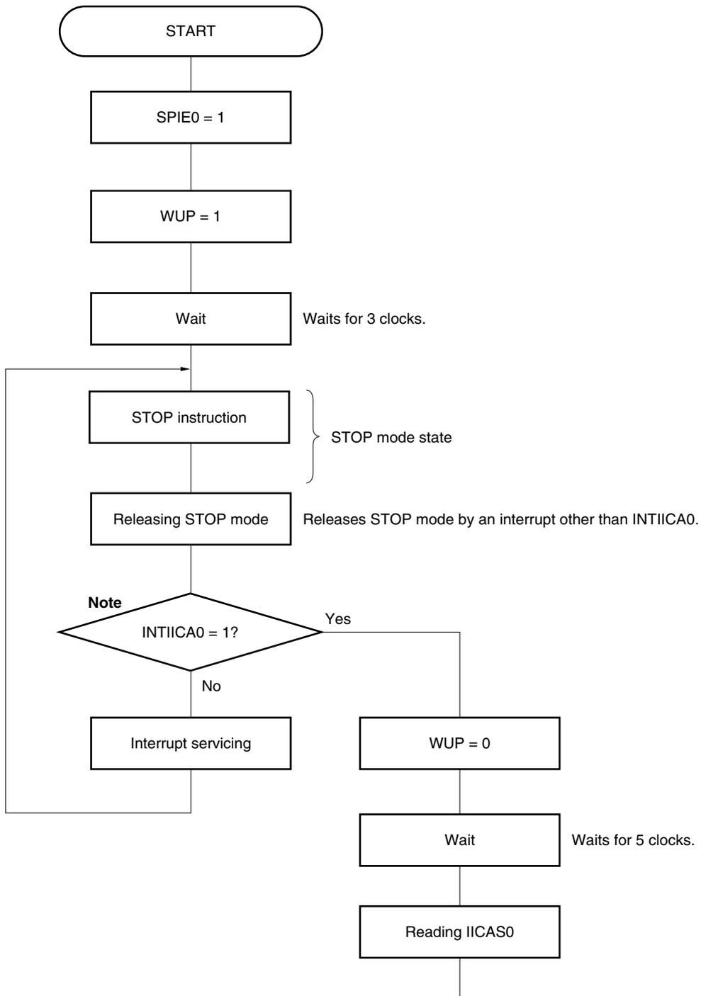
Executes processing corresponding to the operation to be executed after checking the operation state of serial interface IICA.
