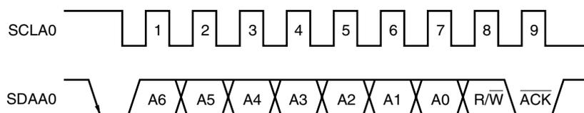
When the local address is received,  $\overline{ACK}$  is automatically generated, regardless of the value of the ACKE0 bit. When an address other than that of the local address is received,  $\overline{ACK}$  is not generated (NACK).
