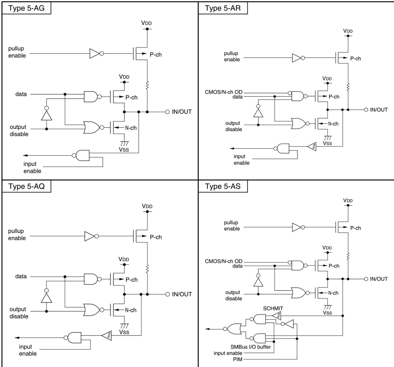
Figure 2-1. Pin I/O Circuit List (2/4)
