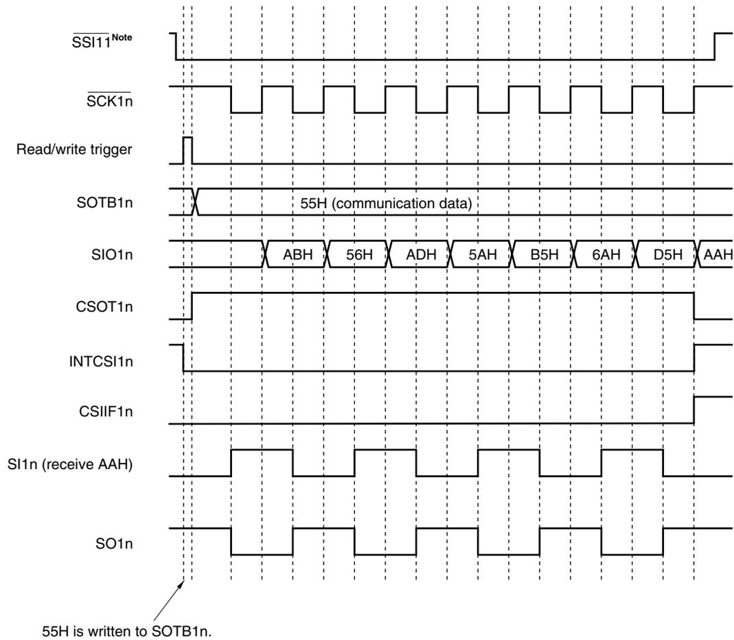
**Note** The SSE11 flag and  $\overline{\text{SSI11}}$  pin are available only for serial interface CSI11 of 78K0/KA2-L (25, 32-pin products) and 78K0/KC2-L (48-pin products), and are used in the slave mode.
