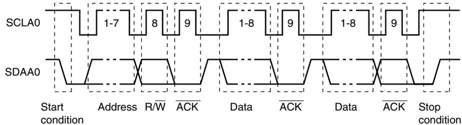
The master device generates the start condition, slave address, and stop condition. The acknowledge ( $\overline{\text{ACK}}$ ) can be generated by either the master or slave device (normally, it is output by the device that receives 8-bit data).
