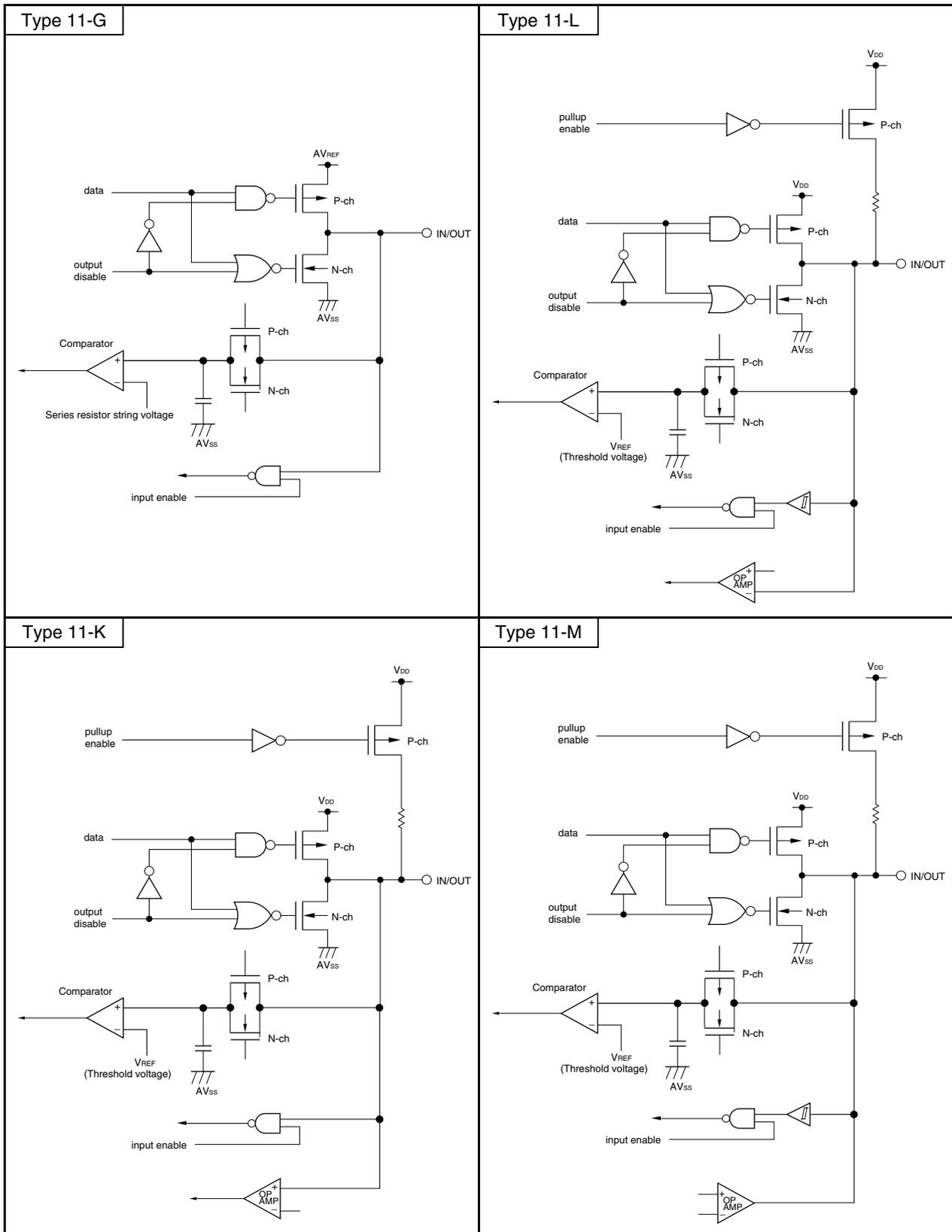
Figure 2-1. Pin I/O Circuit List (3/4)
