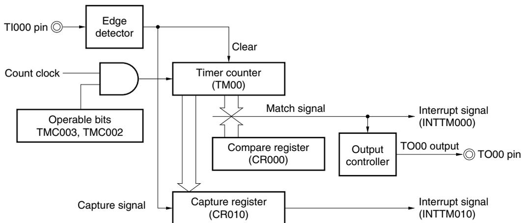
Figure 6-26. Timing Example of Clear & Start Mode Entered by TI000 Pin Valid Edge Input
