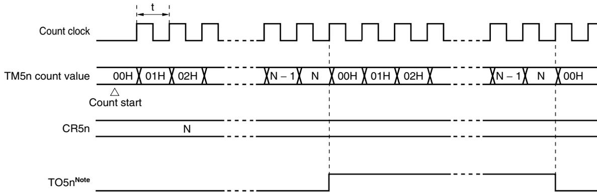
**Note** The initial value of TO5n output can be set by bits 2 and 3 (LVR5n, LVS5n) of 8-bit timer mode control register 5n (TMC5n).
