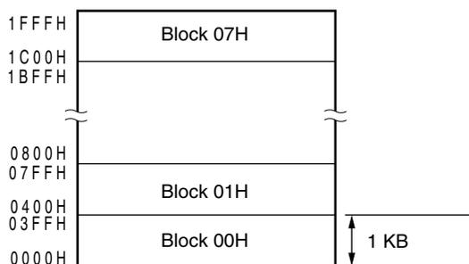
Figure 3-4. Memory Map ( $\mu$ PD78F0573, 78F0578, 78F0583, 78F0588)
