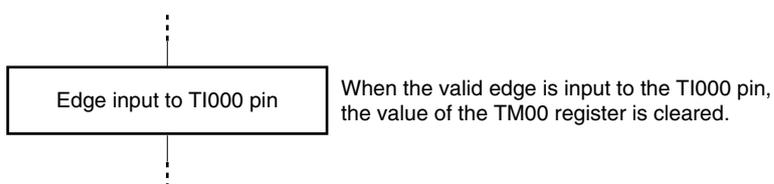
**Note** Care must be exercised when setting TOC00. For details, refer to 6.3 (3) 16-bit timer output control register 00 (TOC00).
