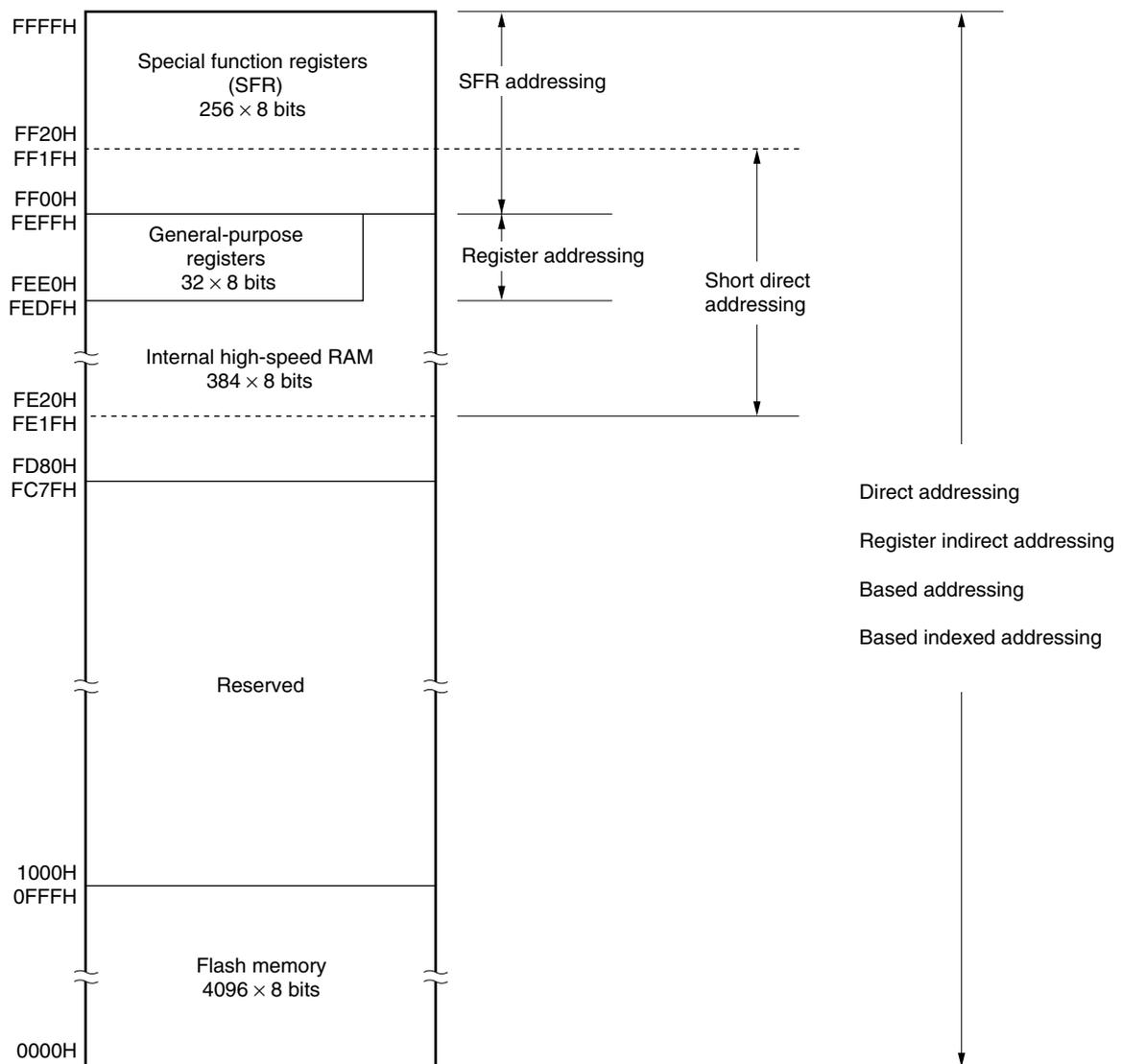
**Figure 3-6. Correspondence Between Data Memory and Addressing**
