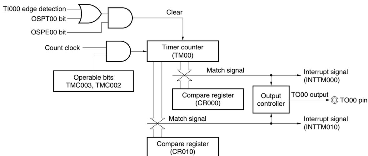
Figure 6-45. Example of Register Settings for One-Shot Pulse Output Operation (1/2)
