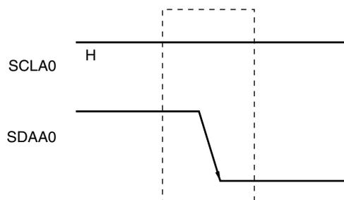
A start condition is output when bit 1 (STT0) of IICA control register 0 (IICACTL0) is set (1) after a stop condition has been detected (SPD0: Bit 0 of the IICA status register 0 (IICAS0) = 1). When a start condition is detected, bit 1 (STD0) of the IICAS0 register is set (1).
