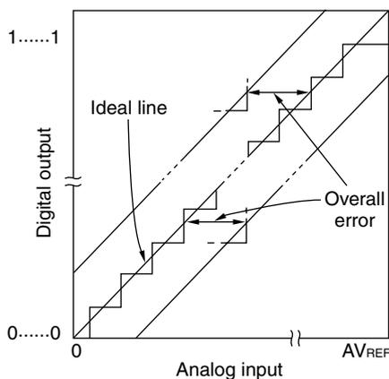
Figure 12-17. Quantization Error
