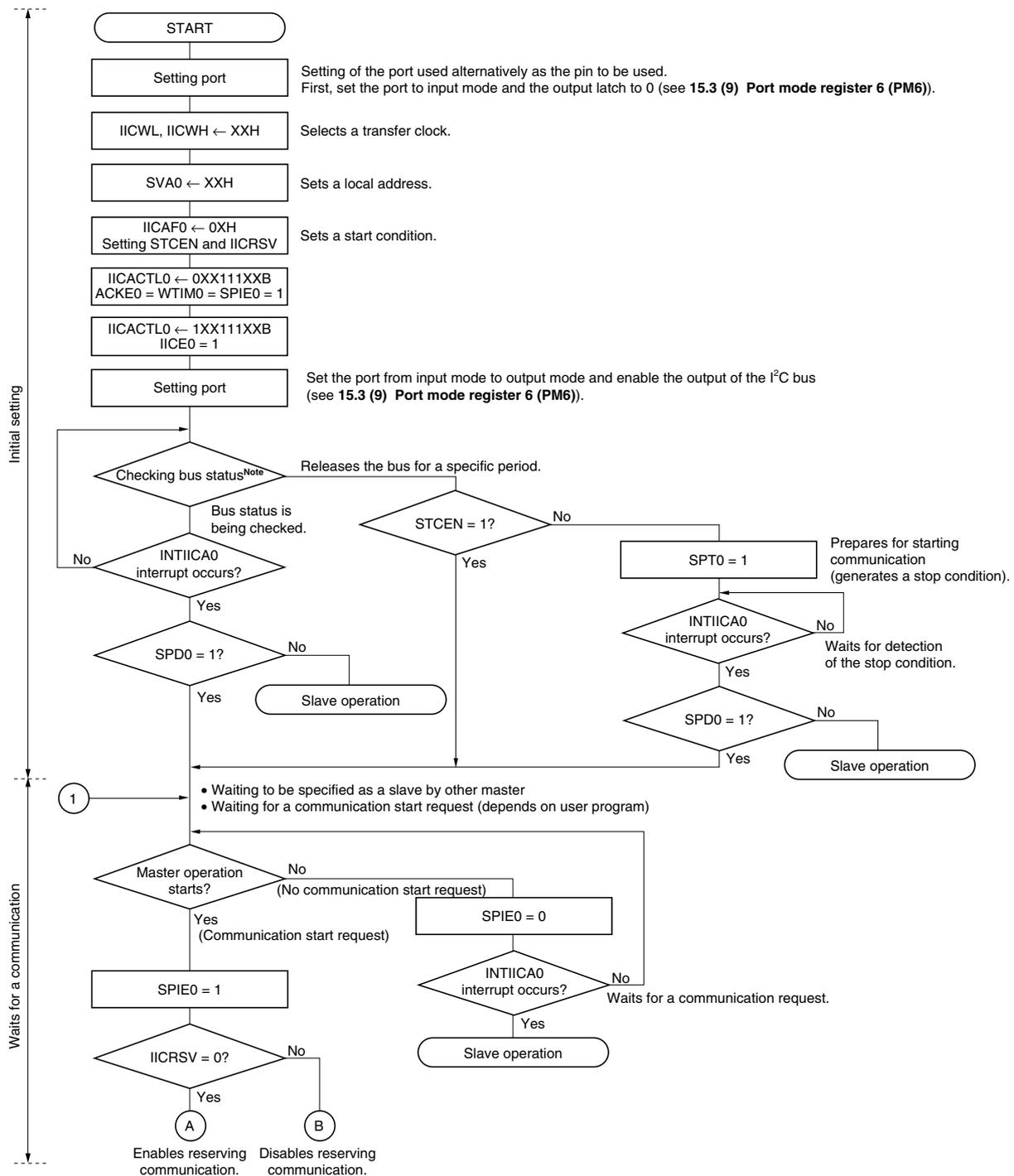
**Note** Confirm that the bus is released (CLD0 bit = 1, DAD0 bit = 1) for a specific period (for example, for a period of one frame). If the SDAA0 pin is constantly at low level, decide whether to release the I<sup>2</sup>C bus (SCLA0 and SDAA0 pins = high level) in conformance with the specifications of the product that is communicating.
