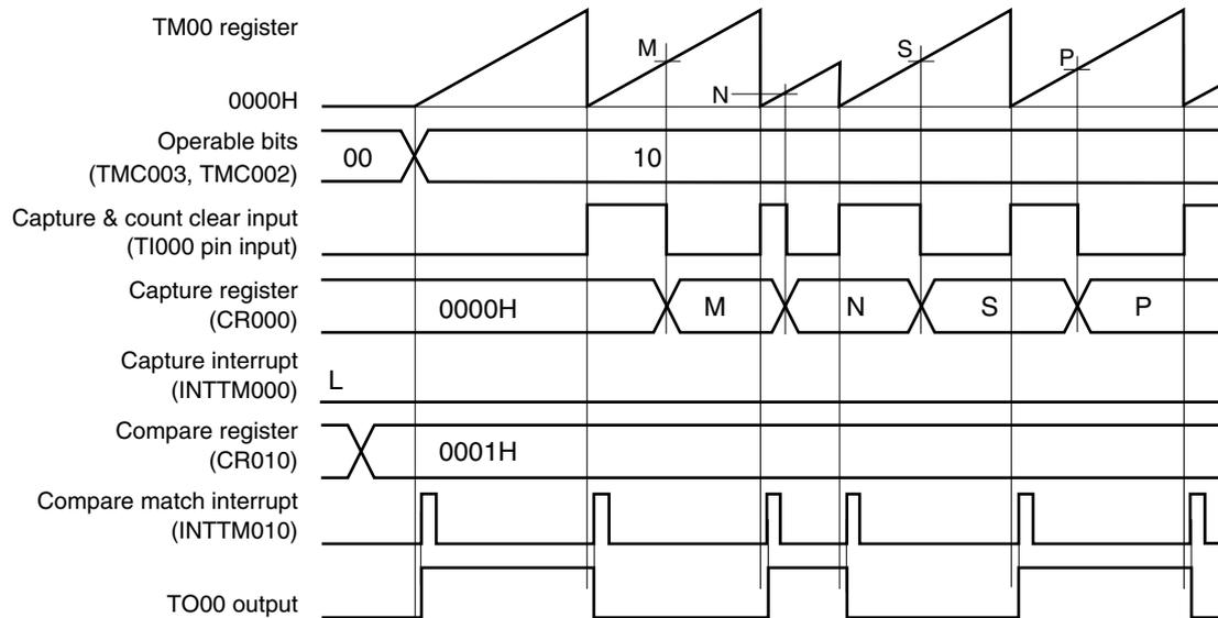
This is an application example where the TO00 output level is to be inverted when the count value has been captured & cleared.
