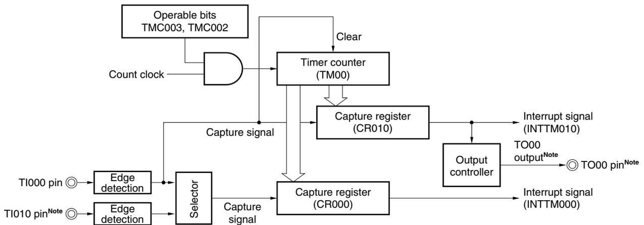
**Note** The timer output (TO00) cannot be used when detecting the valid edge of the TI010 pin is used.
