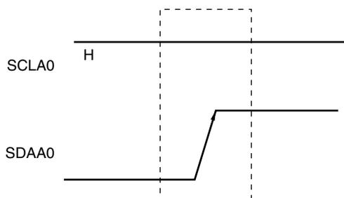
A stop condition is generated when bit 0 (SPT0) of the IICA control register 0 (IICACTL0) is set to 1. When the stop condition is detected, bit 0 (SPD0) of the IICA status register 0 (IICAS0) is set to 1 and INTIICA0 is generated when bit 4 (SPIE0) of the IICACTL0 register is set to 1.
