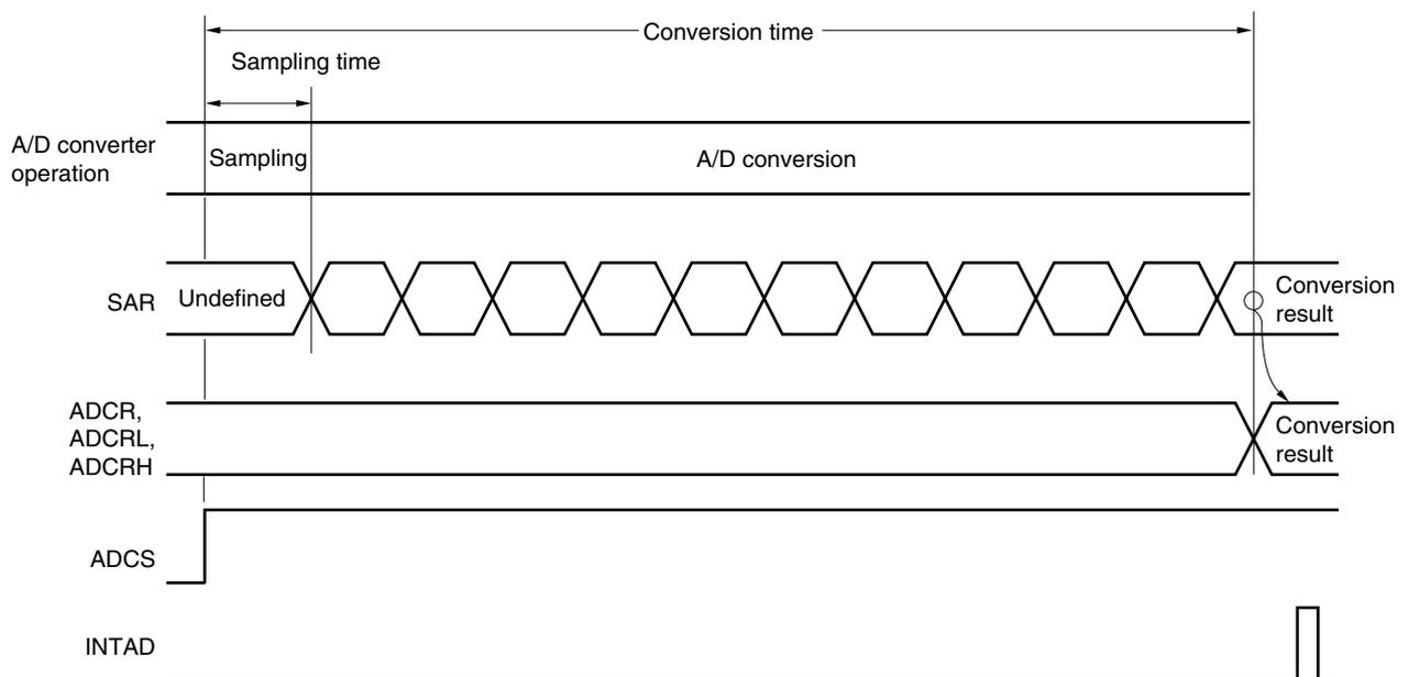
A/D conversion operations are performed continuously until bit 7 (ADCS) of the A/D converter mode register 0 (ADM0) is reset (0) by software.
