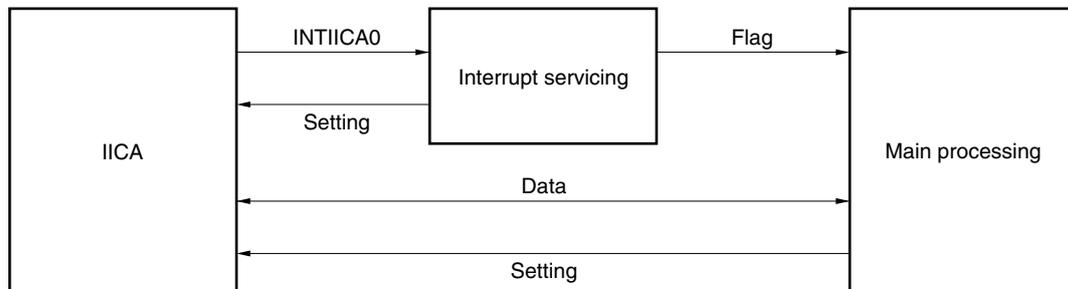
Therefore, data communication processing is performed by preparing the following three flags and passing them to the main processing instead of INTIICA0.
