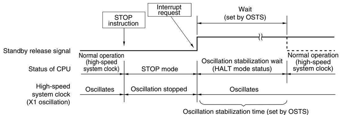
**(2) When high-speed system clock (external clock input) is used as CPU clock**
