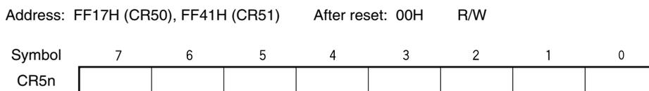
**Cautions 1. In the mode in which clear & start occurs on a match of TM5n and CR5n (TMC5n6 = 0), do not write other values to CR5n during operation.**
