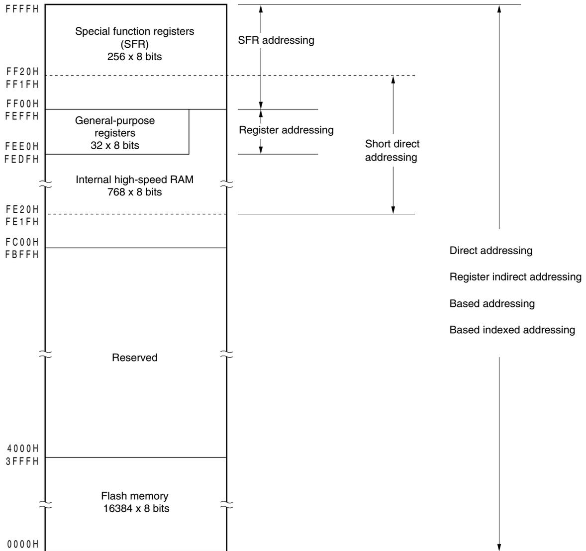
**Figure 3-8. Correspondence Between Data Memory and Addressing**
