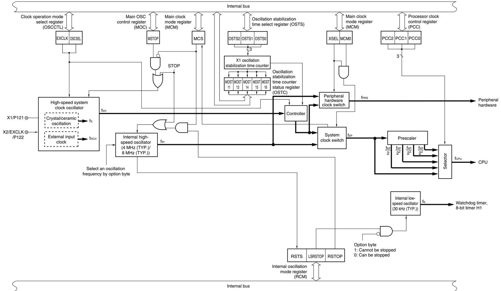
Figure 5-2. Block Diagram of Clock Generator (78K0/KC2-L)
