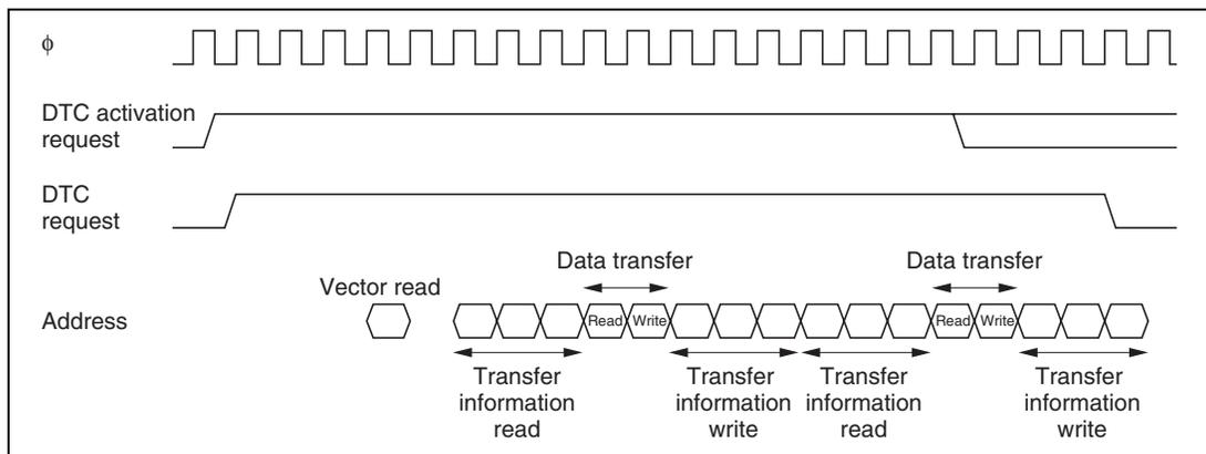
**Figure 7.12 DTC Operation Timing (Example of Chain Transfer)**
