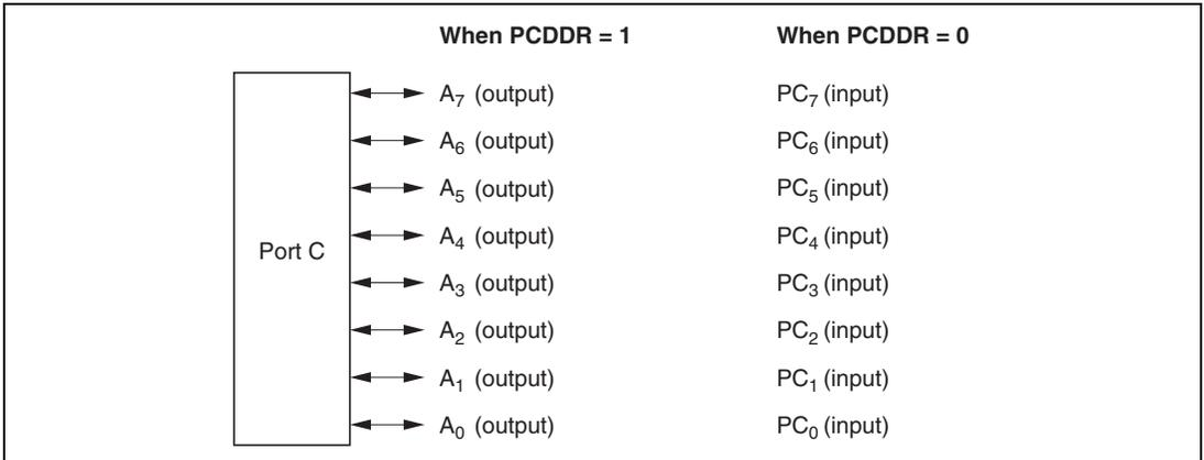
**Figure 8.17 Port C Pin Functions (Modes 2 and 6)**
