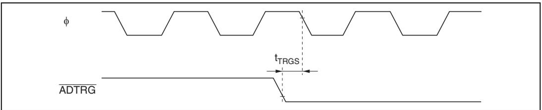
**Figure 20.23 A/D Converter External Trigger Input Timing**
