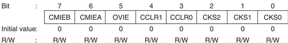
TCR0 and TCR1 are 8-bit readable/writable registers that select the clock source and the time at which TCNT is cleared, and enable interrupts.
