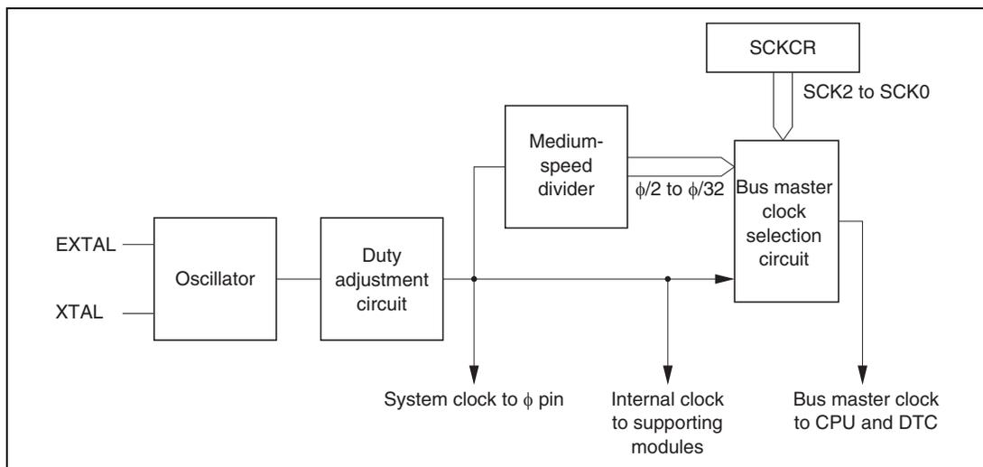
**Figure 18.1 Block Diagram of Clock Pulse Generator**
