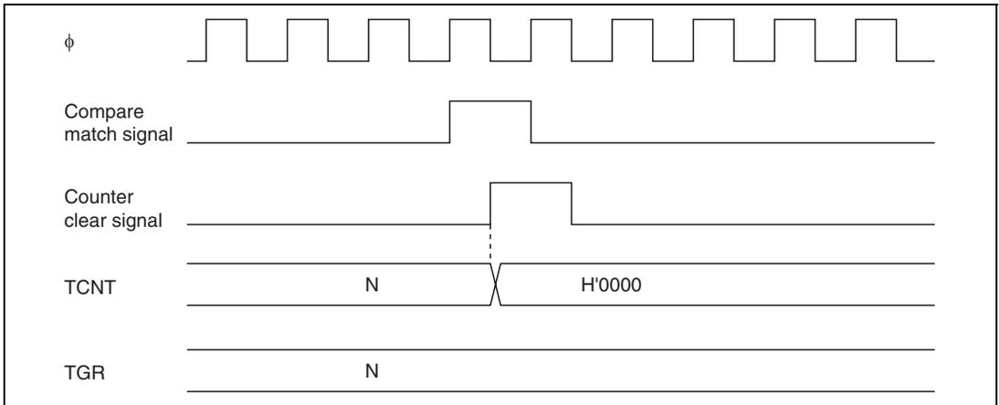
**Figure 9.38 Counter Clear Timing (Compare Match)**
