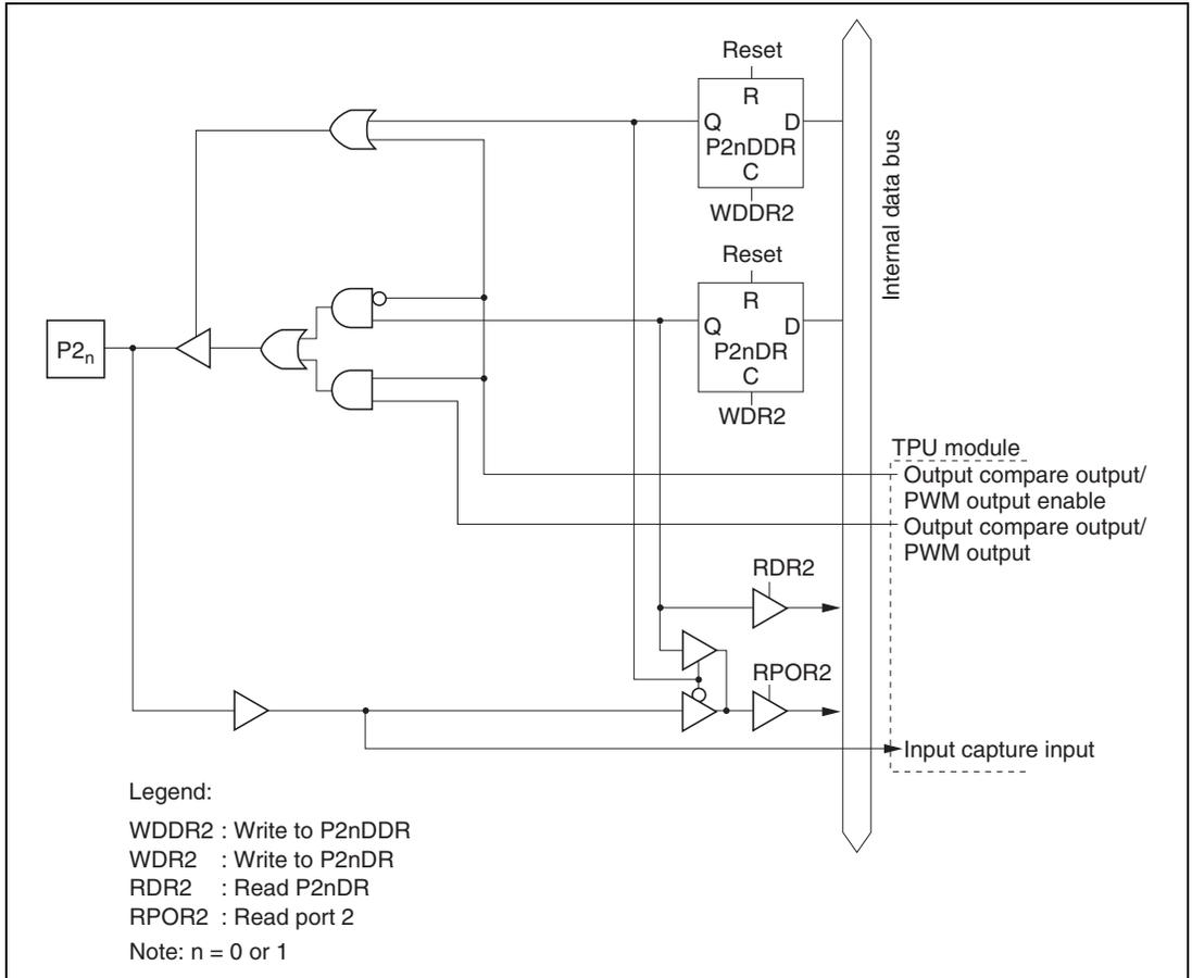
Figure C.2 (a) Port 2 Block Diagram (Pins P2<sub>0</sub> and P2<sub>1</sub>)
