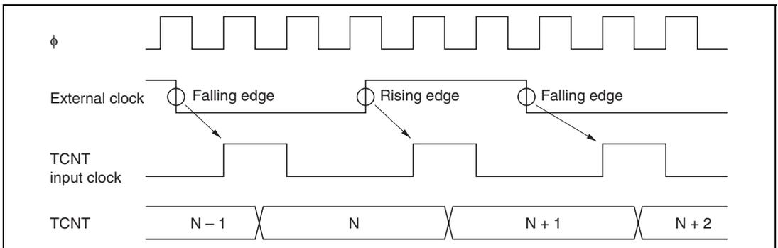
**Figure 9.35 Count Timing in External Clock Operation**
