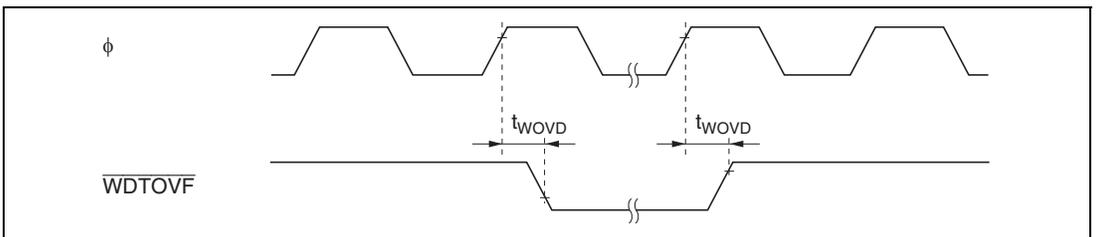
**Figure 20.20 WDT Output Timing**
