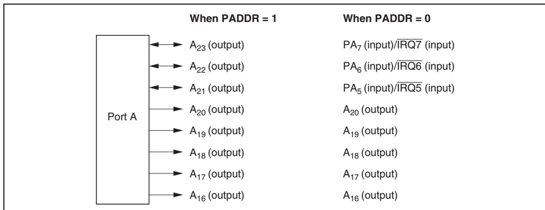
**Figure 8.9 Port A Pin Functions (Modes 4 and 5)**
