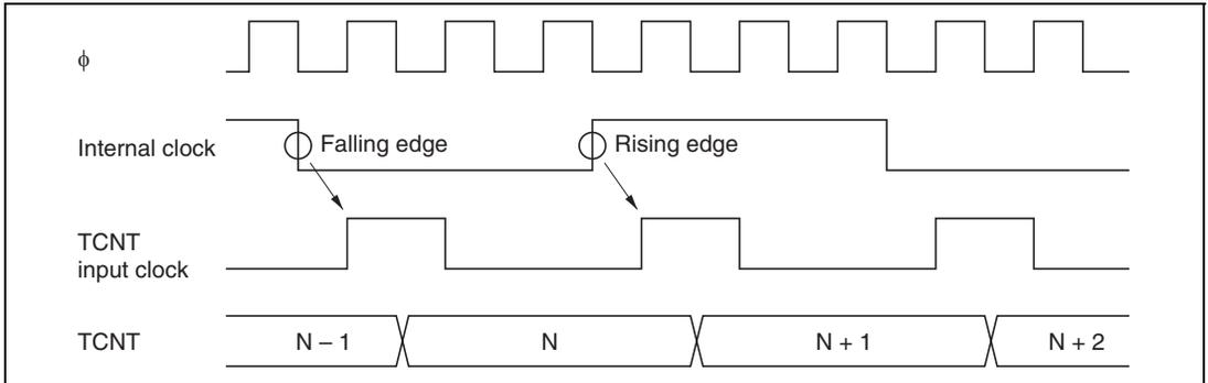
**Figure 9.34 Count Timing in Internal Clock Operation**
