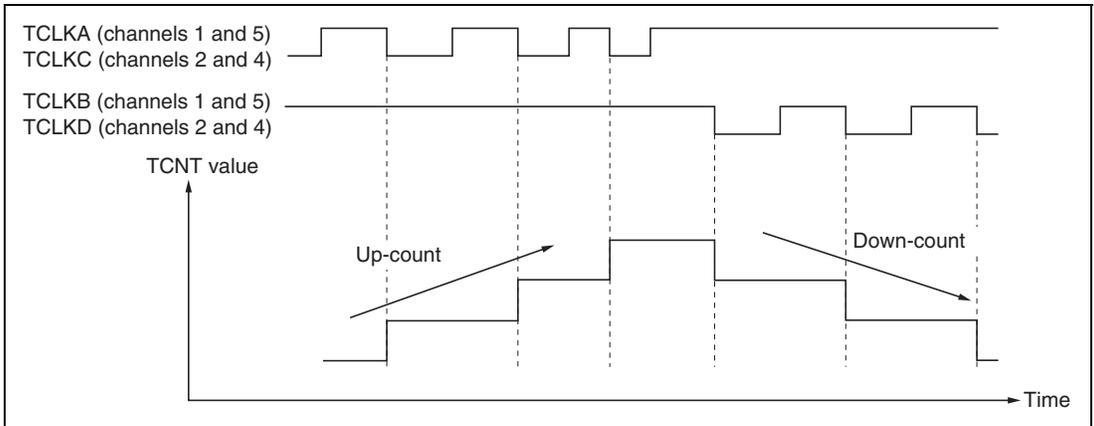
**Figure 9.31 Example of Phase Counting Mode 3 Operation**
