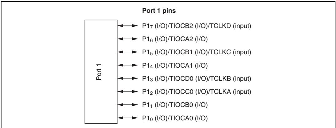
**Figure 8.1 Port 1 Pin Functions**
