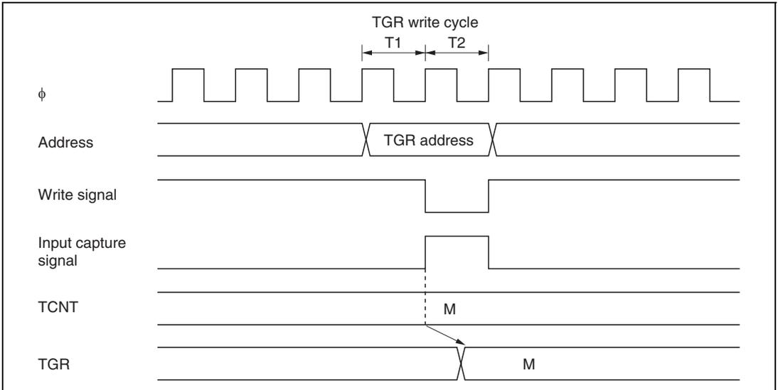
**Figure 9.54** Contention between TGR Write and Input Capture
