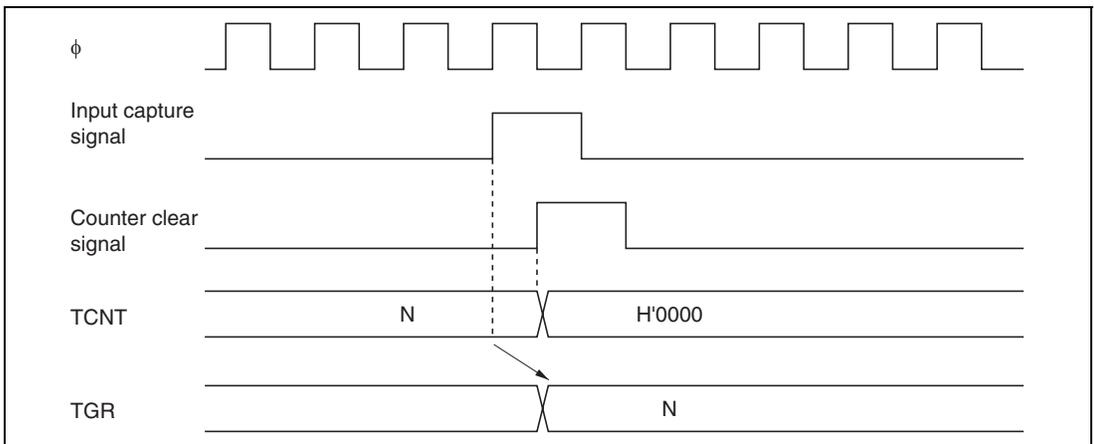
**Figure 9.39 Counter Clear Timing (Input Capture)**
