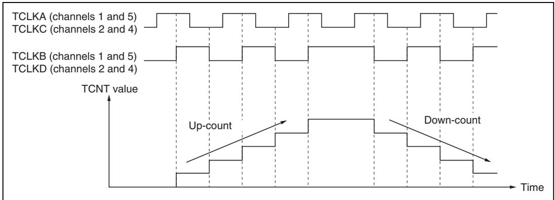
**Figure 9.32 Example of Phase Counting Mode 4 Operation**
