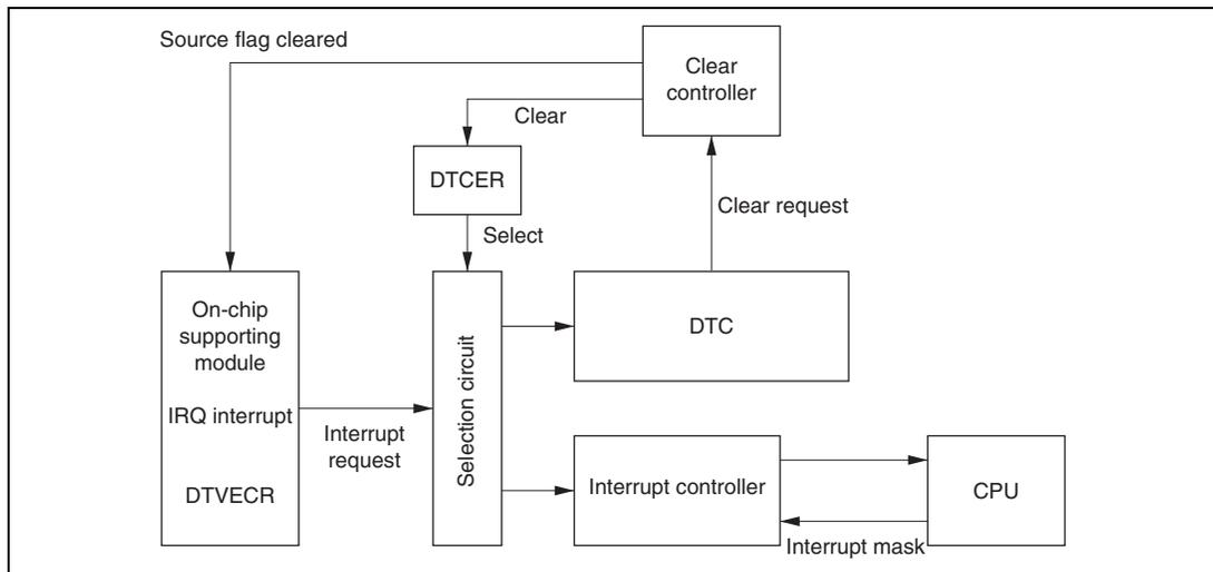
**Figure 7.3 Block Diagram of DTC Activation Source Control**
