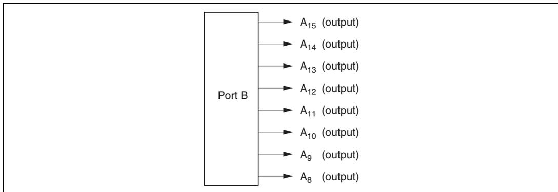
**Figure 8.12 Port B Pin Functions (Modes 1, 4, and 5)**
