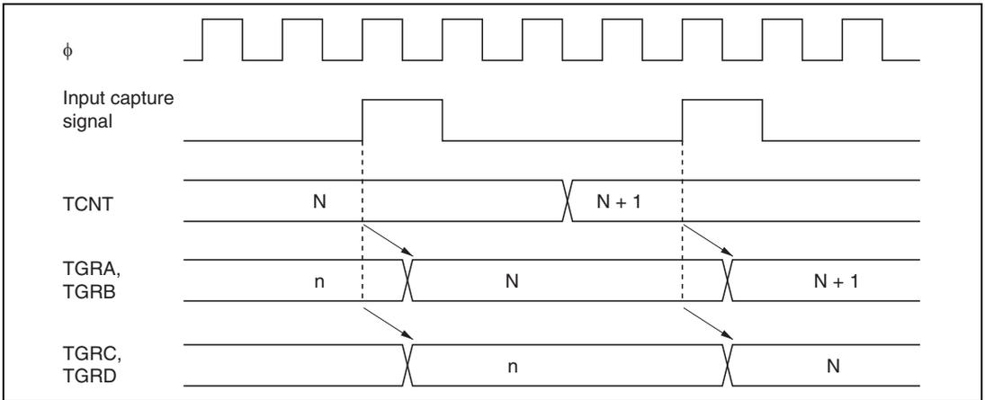
**Figure 9.41 Buffer Operation Timing (Input Capture)**
