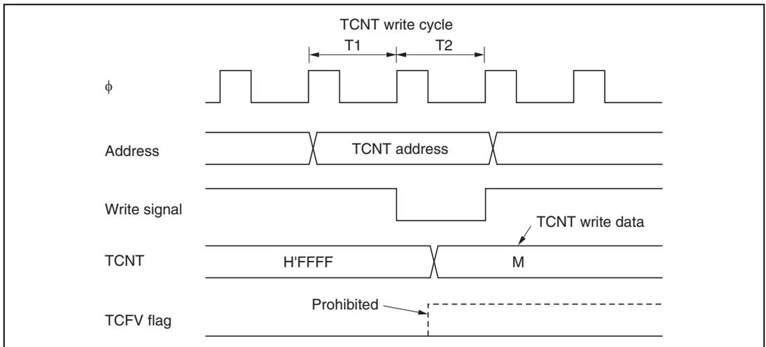
**Figure 9.57 Contention between TCNT Write and Overflow**
