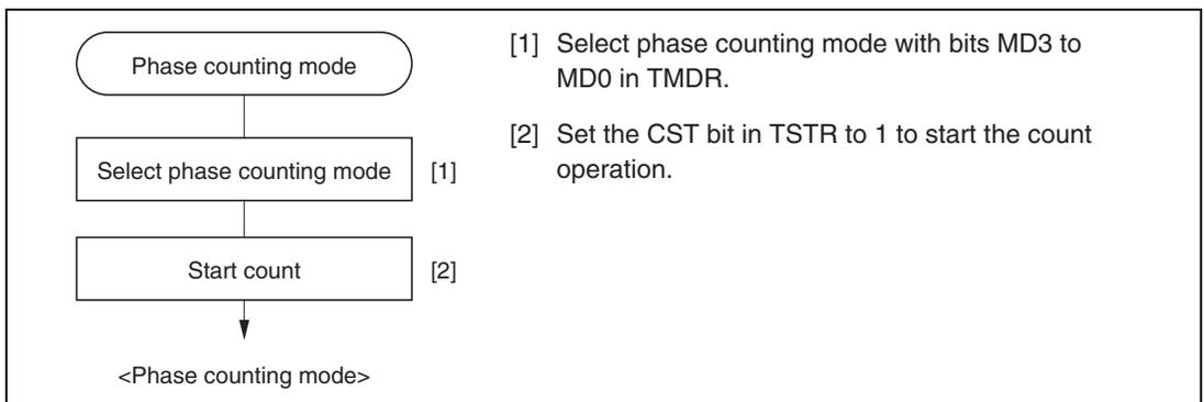
**Figure 9.28 Example of Phase Counting Mode Setting Procedure**
