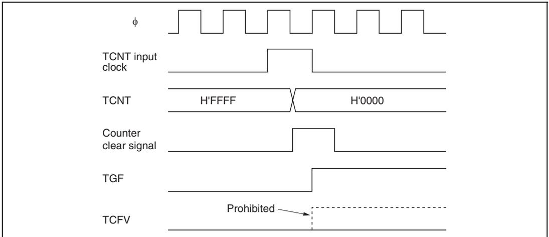
**Figure 9.56** Contention between Overflow and Counter Clearing
