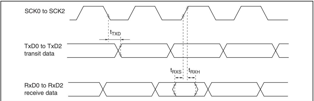
**Figure 20.22 SCI Input/Output Timing (Clock Synchronous Mode)**
