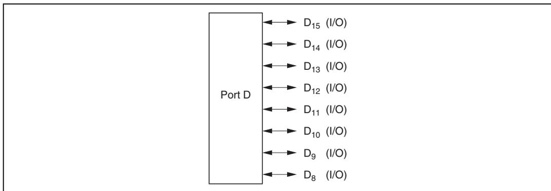
**Figure 8.20 Port D Pin Functions (Modes 1, 2, 4, 5, and 6)**
