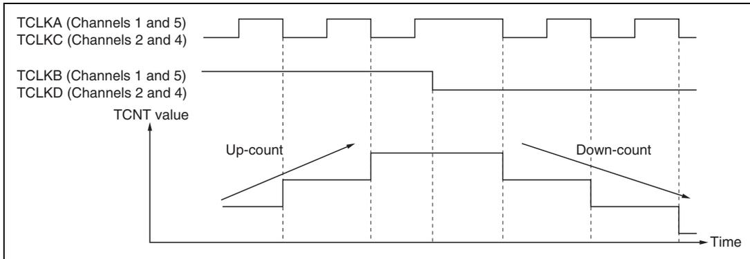
**Figure 9.30 Example of Phase Counting Mode 2 Operation**
