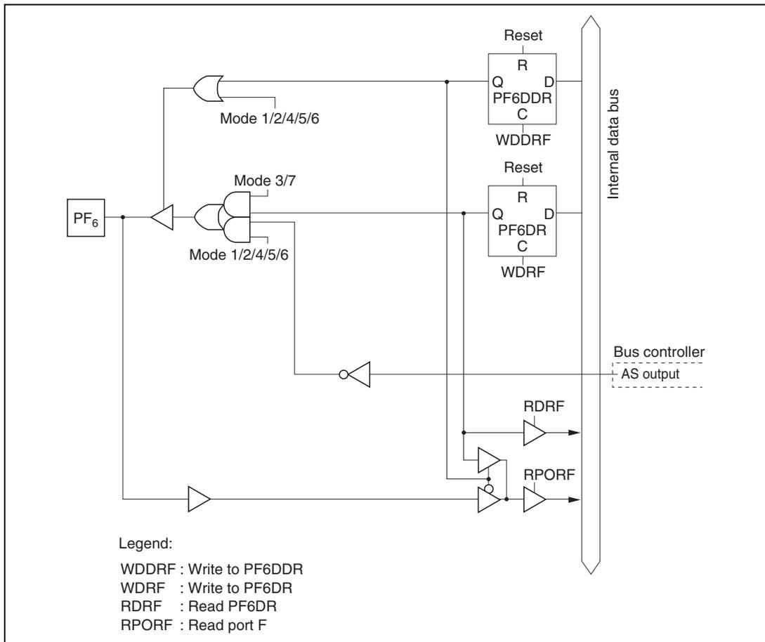
**Figure C.12 (g) Port F Block Diagram (Pin PF<sub>6</sub>)**
