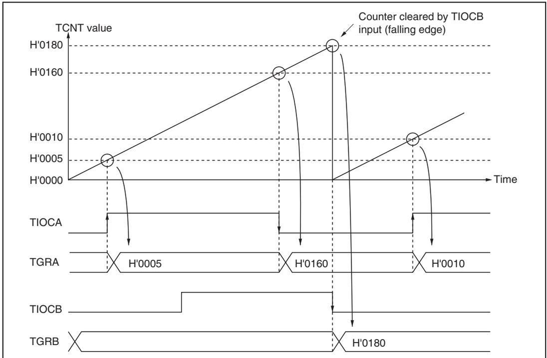
**Figure 9.13 Example of Input Capture Operation**
