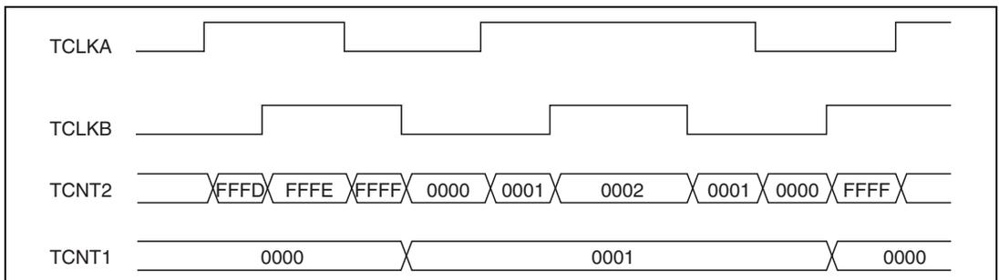
**Figure 9.23 Example of Cascaded Operation (2)**
