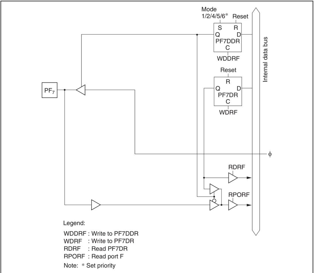
Figure C.12 (h) Port F Block Diagram (Pin PF<sub>7</sub>)
