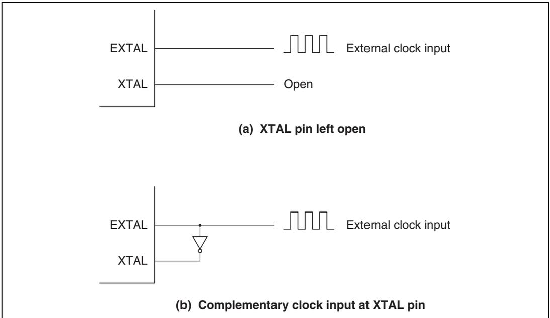
**Figure 18.5 External Clock Input (Examples)**
