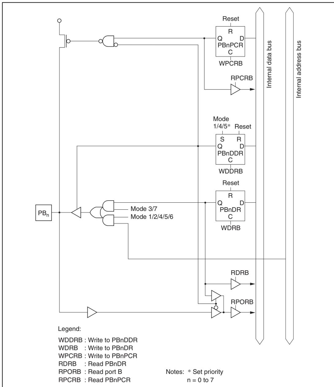
**Figure C.8 Port B Block Diagram (Pin  $PB_n$ )**
