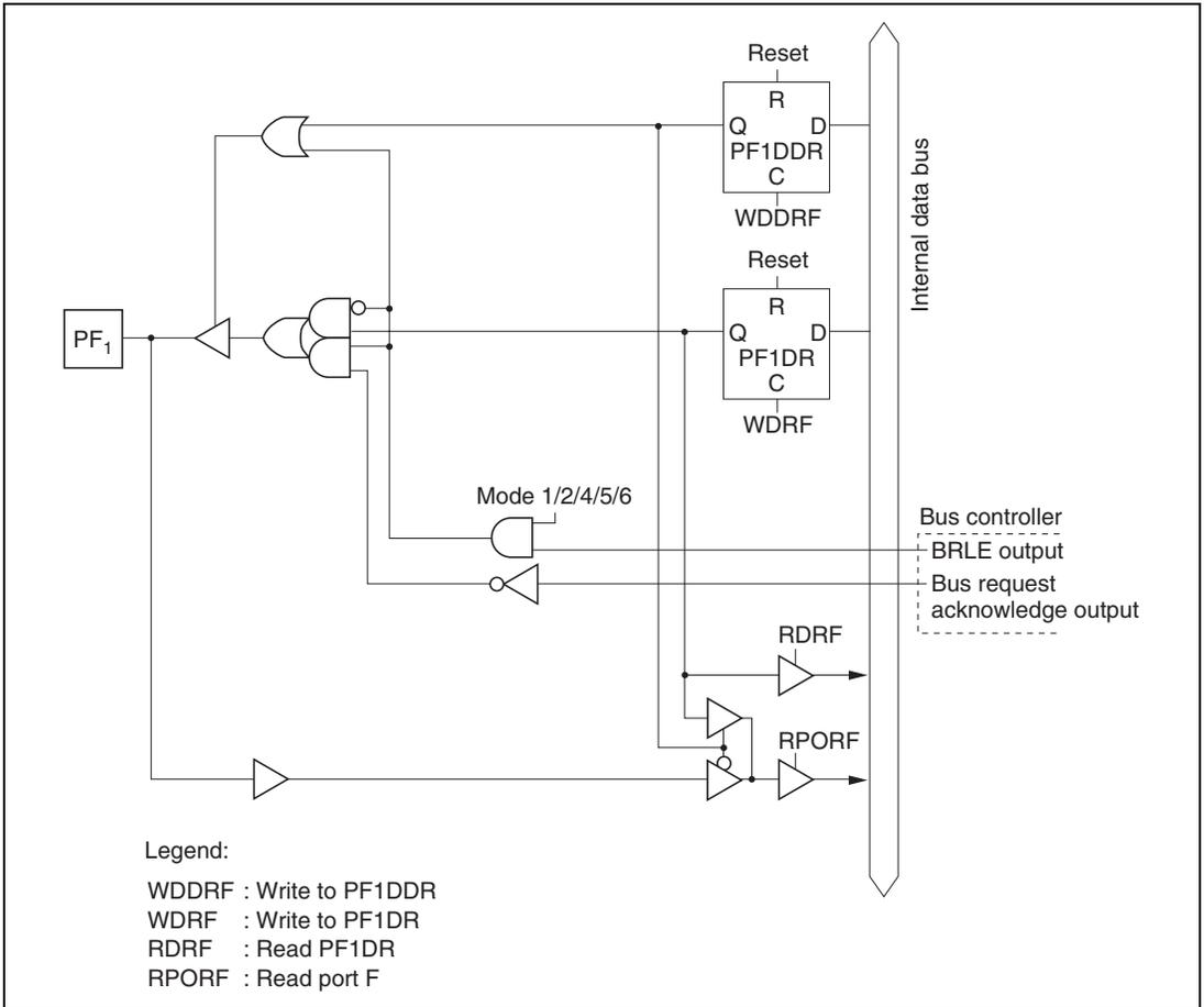
**Figure C.12 (b) Port F Block Diagram (Pin PF<sub>1</sub>)**
