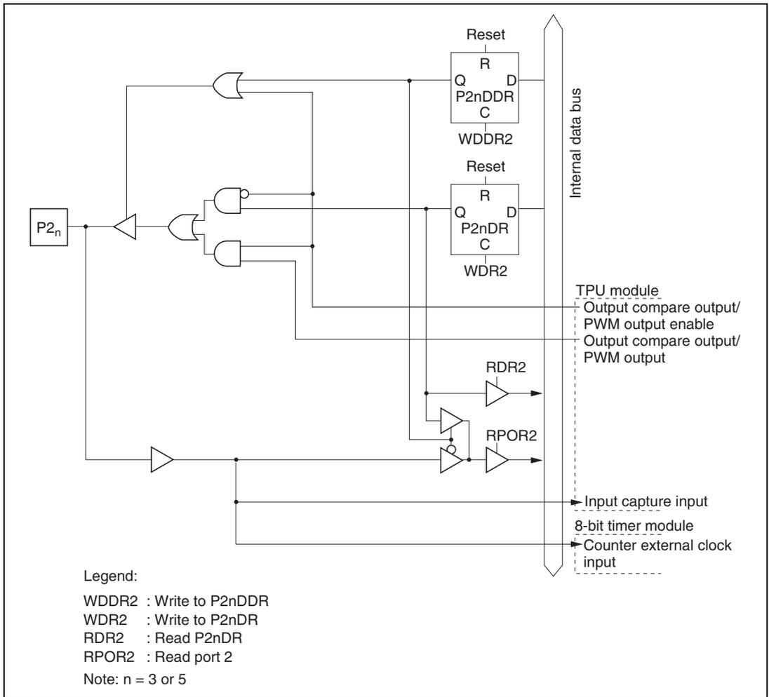
Figure C.2 (c) Port 2 Block Diagram (Pins P2<sub>3</sub> and P2<sub>5</sub>)
