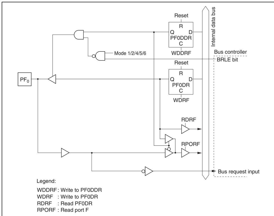
**Figure C.12 (a) Port F Block Diagram (Pin PF<sub>0</sub>)**
