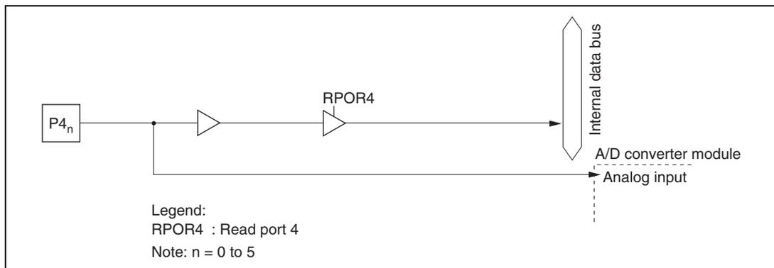
**Figure C.4 (a) Port 4 Block Diagram (Pins P4<sub>0</sub> to P4<sub>5</sub> in H8S/2355 and H8S/2353, Pins P4<sub>0</sub> to P4<sub>7</sub> in H8S/2393)**
