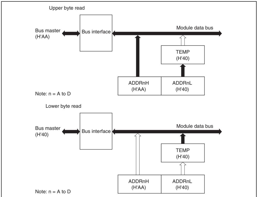
**Figure 14.2 ADDR Access Operation (Reading H'AA40)**
