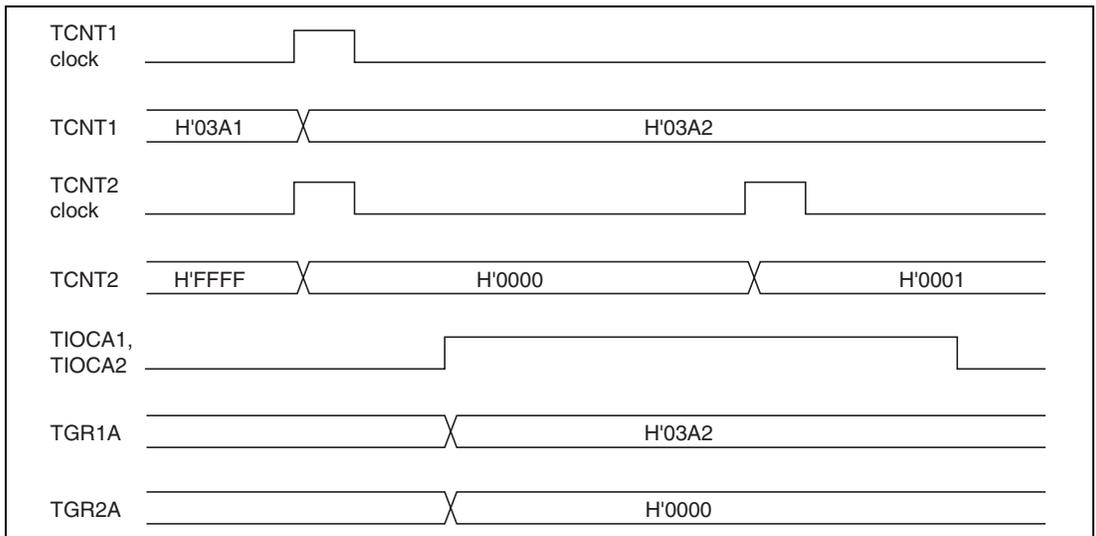
**Figure 9.22 Example of Cascaded Operation (1)**
