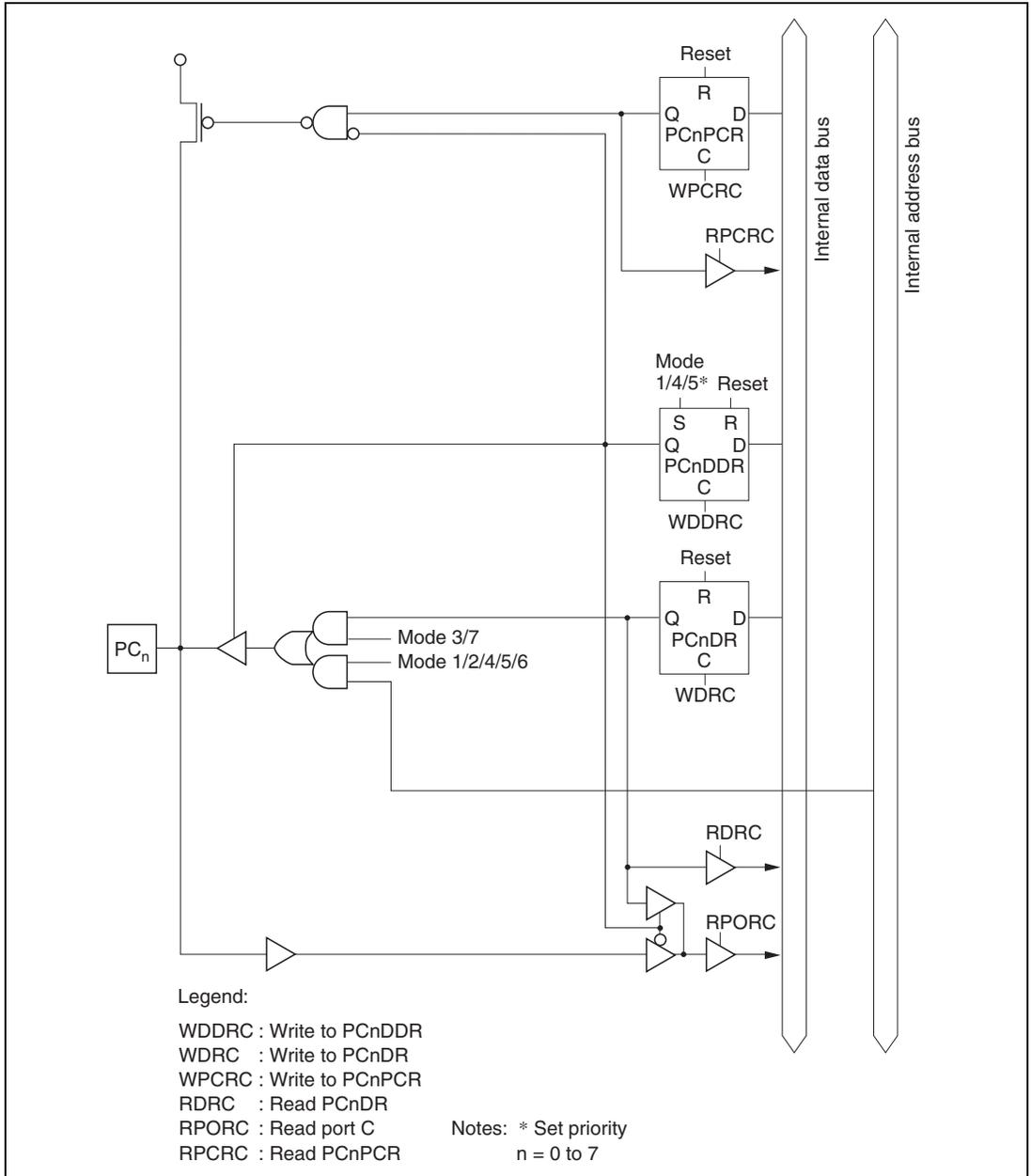
Figure C.9 Port C Block Diagram (Pin PC<sub>n</sub>)
