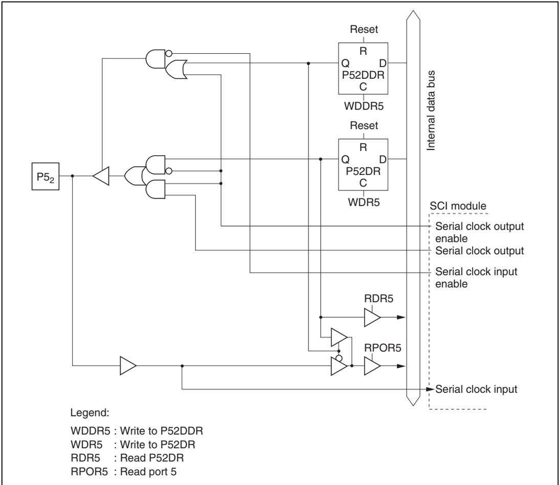
**Figure C.5 (c) Port 5 Block Diagram (Pin P5<sub>2</sub>)**
