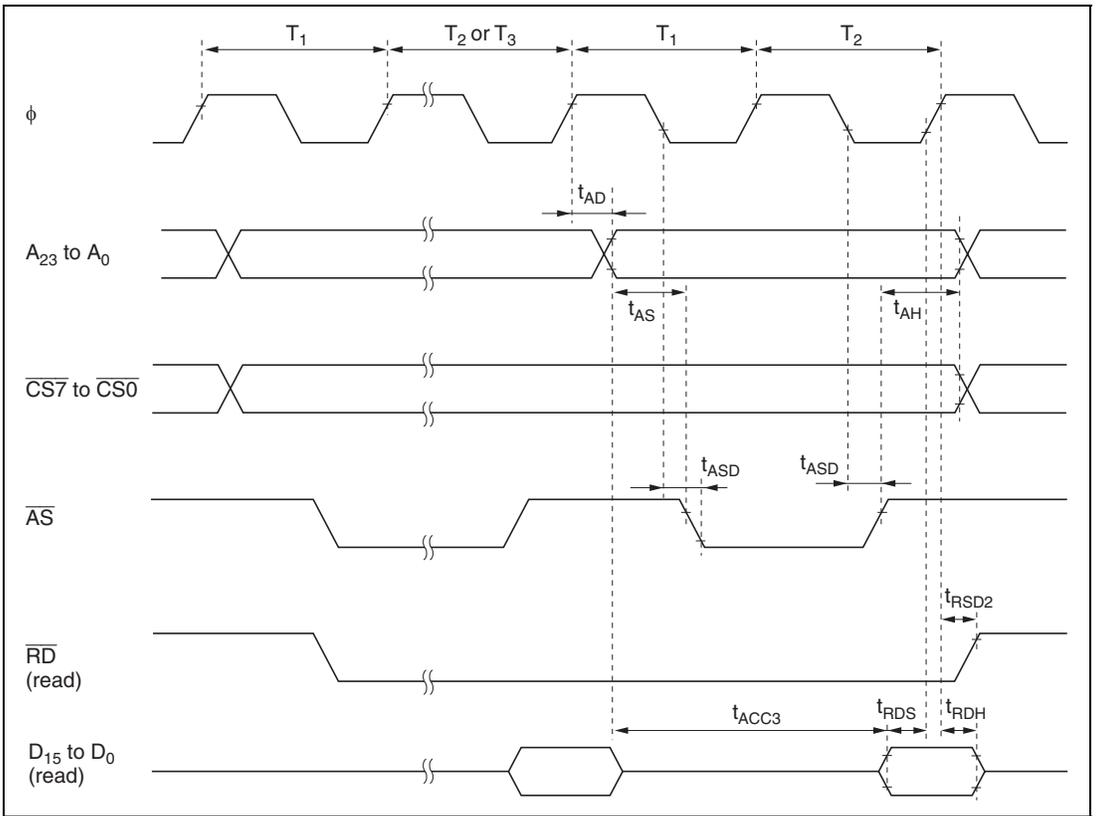
**Figure 20.11 Burst ROM Access Timing (Two-State Access)**
