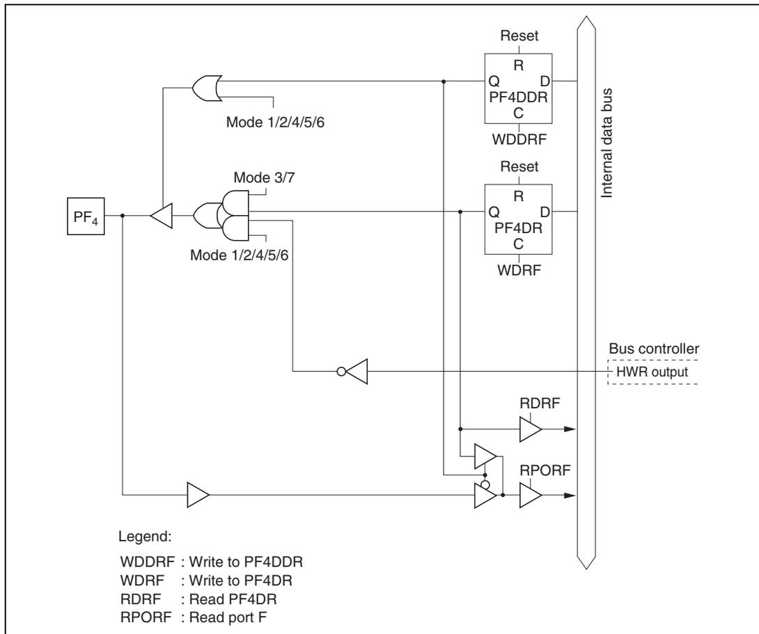
Figure C.12 (e) Port F Block Diagram (Pin PF<sub>4</sub>)
