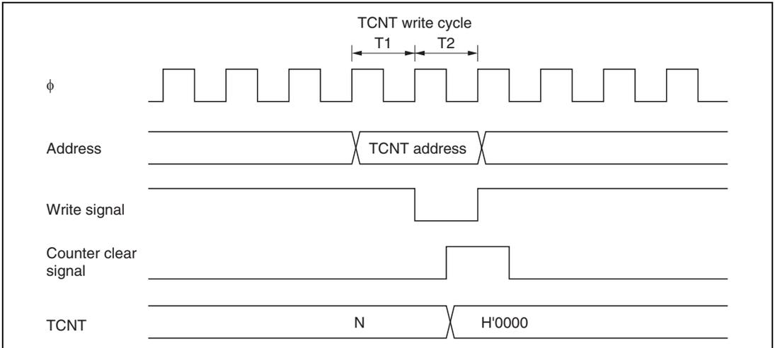
**Figure 9.49** Contention between TCNT Write and Clear Operations
