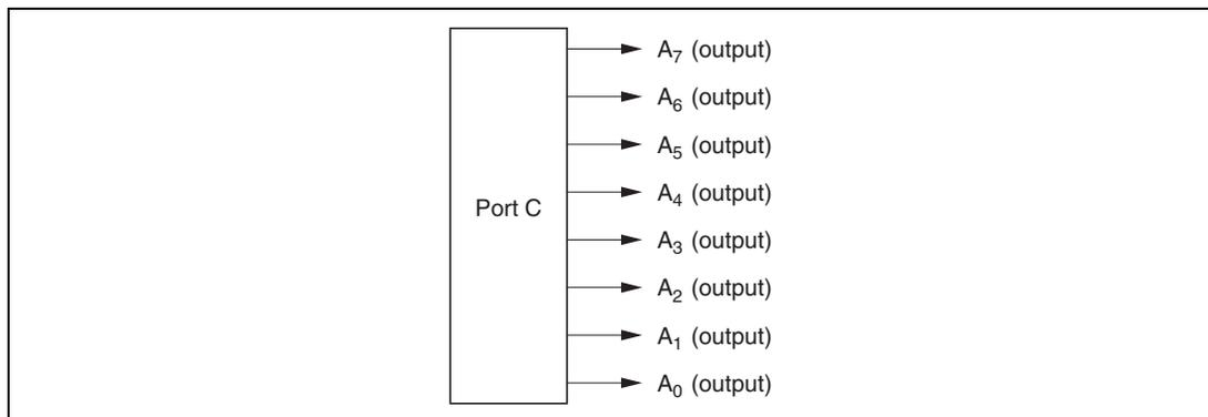
**Figure 8.16 Port C Pin Functions (Modes 1, 4, and 5)**
