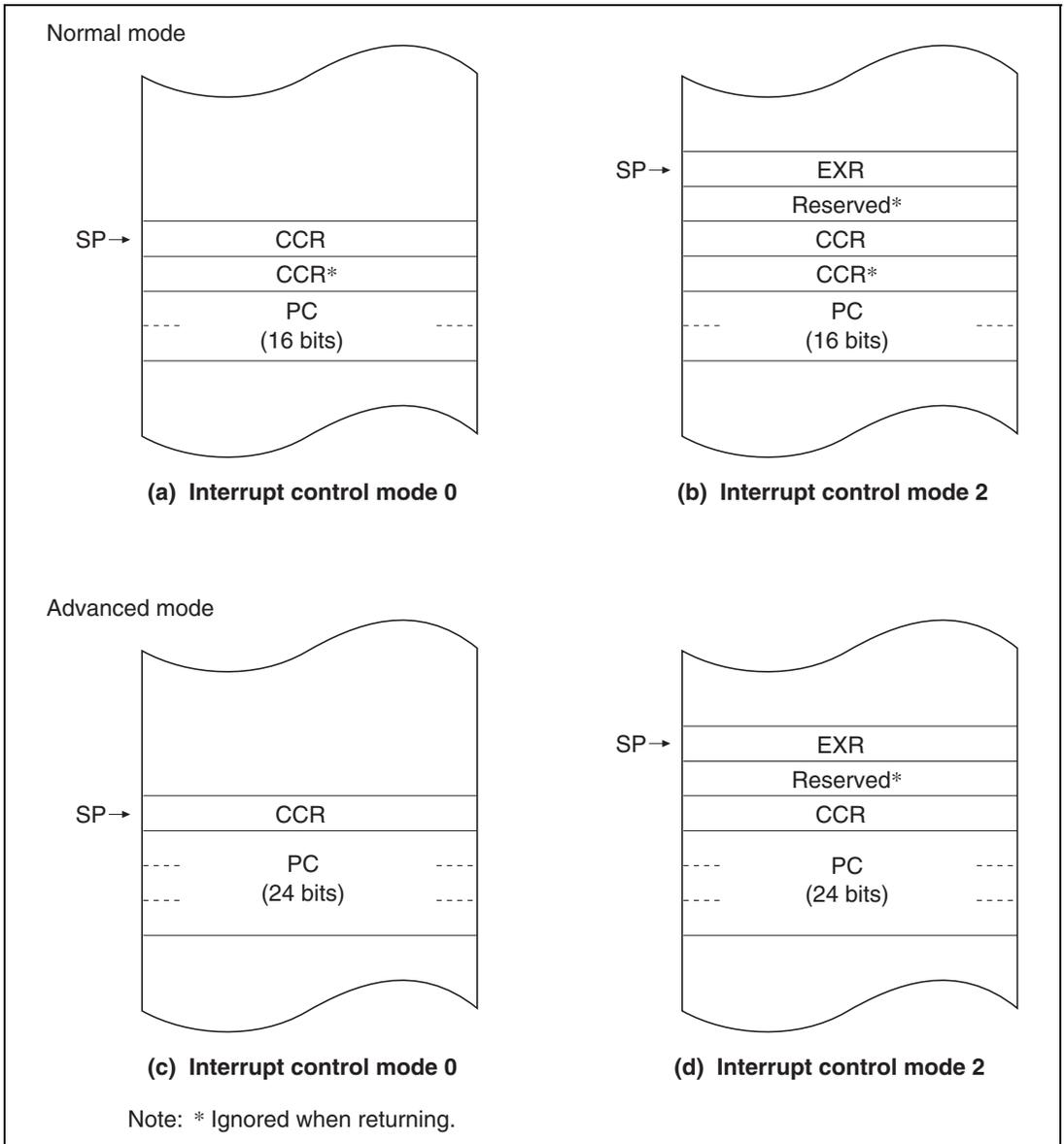
**Figure 2.16 Stack Structure after Exception Handling (Examples)**
