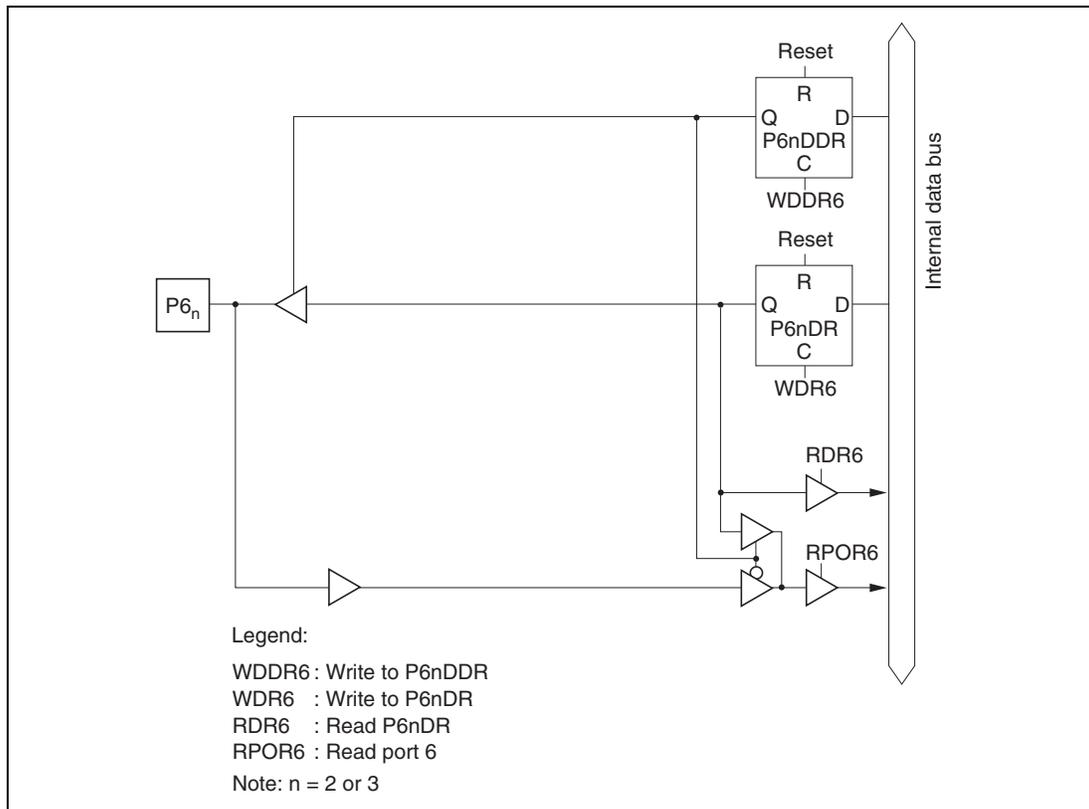
**Figure C.6 (b) Port 6 Block Diagram (Pins P6<sub>2</sub> and P6<sub>3</sub>)**
