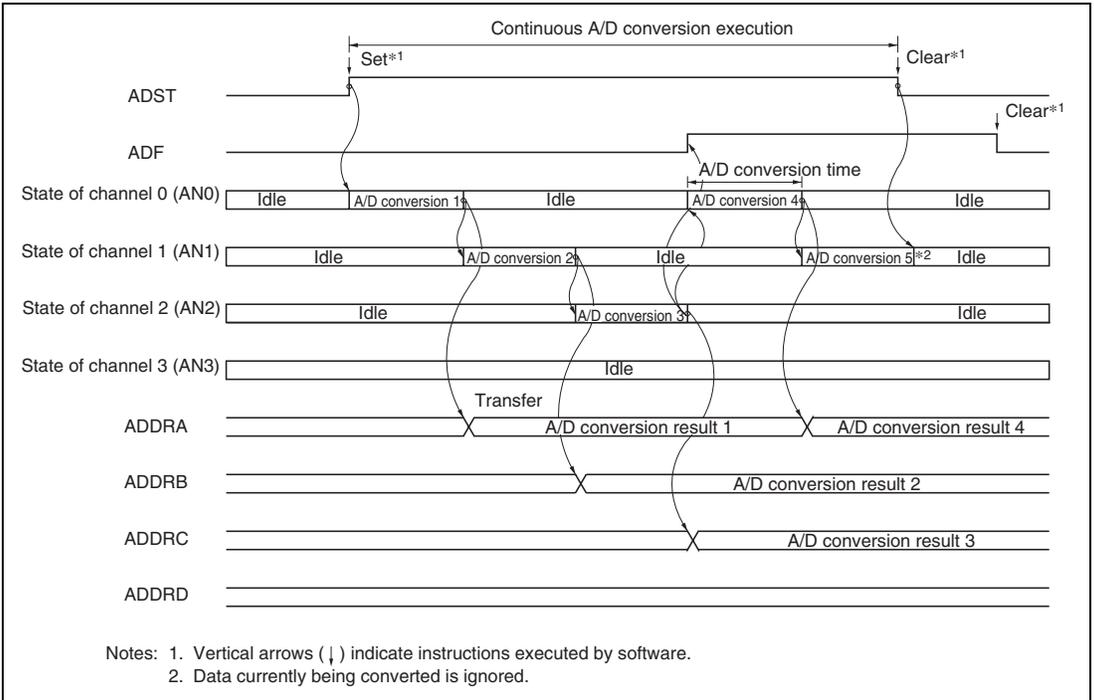
**Figure 14.4 Example of A/D Converter Operation
