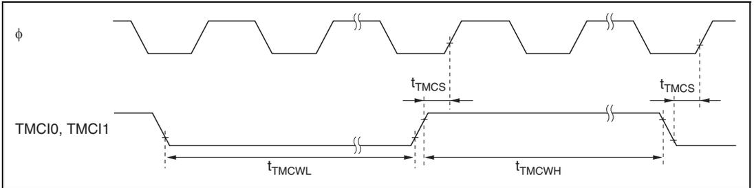
**Figure 20.18 8-Bit Timer Clock Input Timing**
