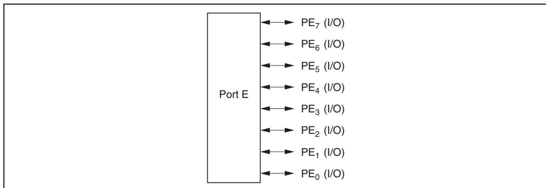
**Figure 8.24 Port E Pin Functions (Modes 3 and 7)**
