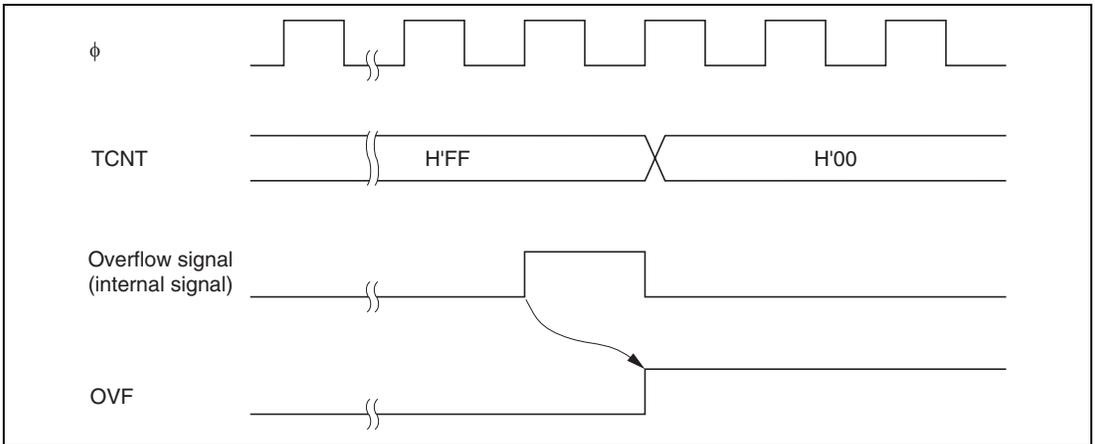
**Figure 11.6 Timing of Setting of OVF**
