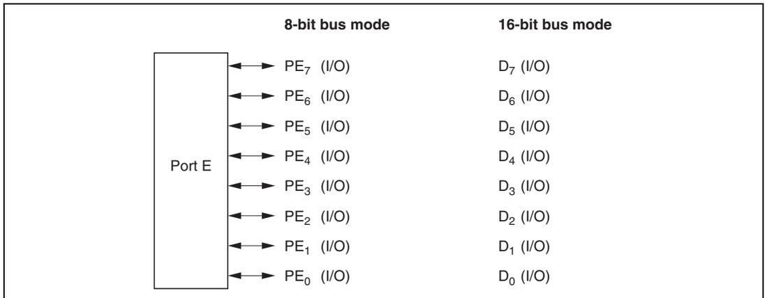
**Figure 8.23 Port E Pin Functions (Modes 1, 2, 4, 5, and 6)**
