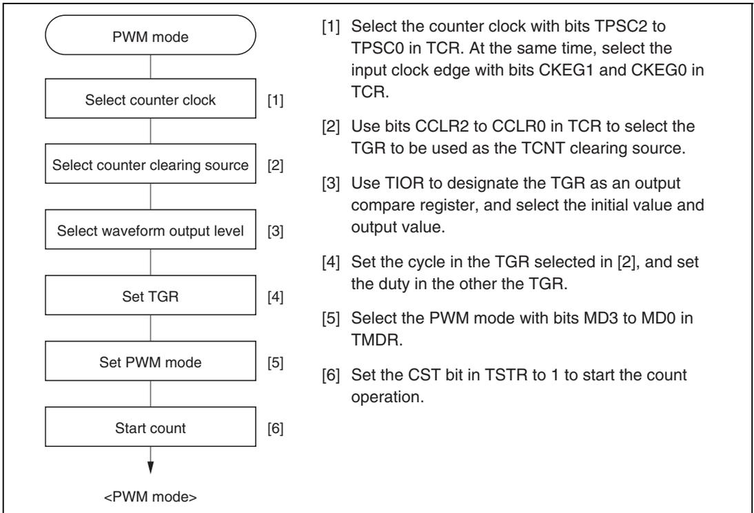
**Figure 9.24 Example of PWM Mode Setting Procedure**
