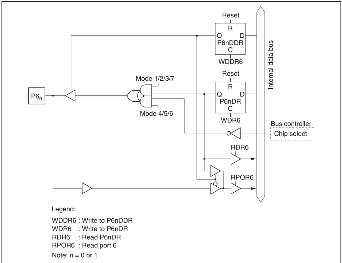
**Figure C.6 (a) Port 6 Block Diagram (Pins P6<sub>0</sub> and P6<sub>1</sub>)**
