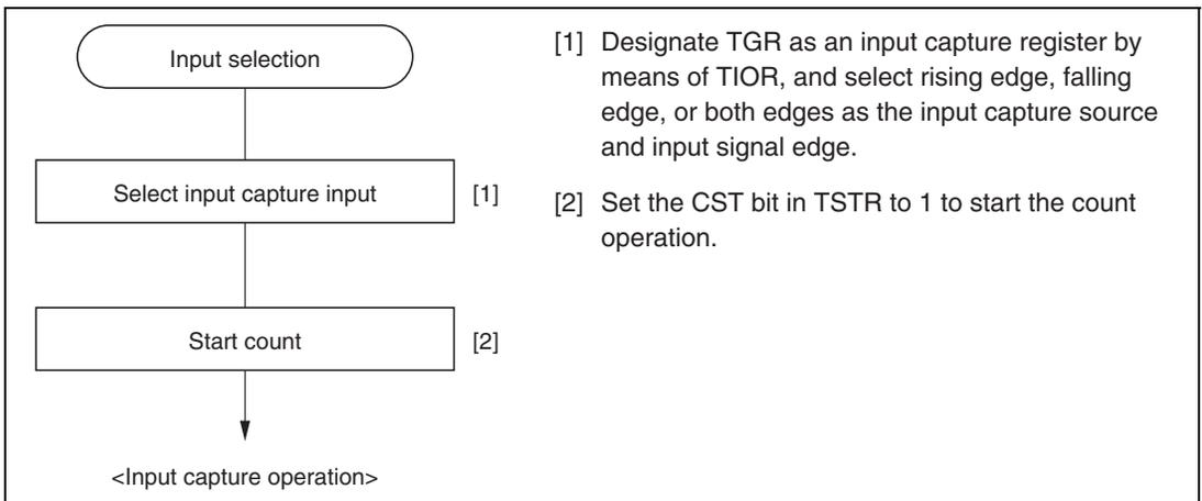
**Figure 9.12 Example of Input Capture Operation Setting Procedure**
