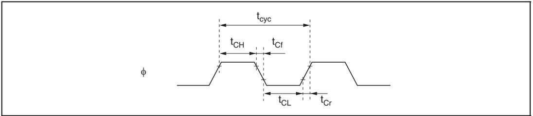
Figure 20.4 System Clock Timing
