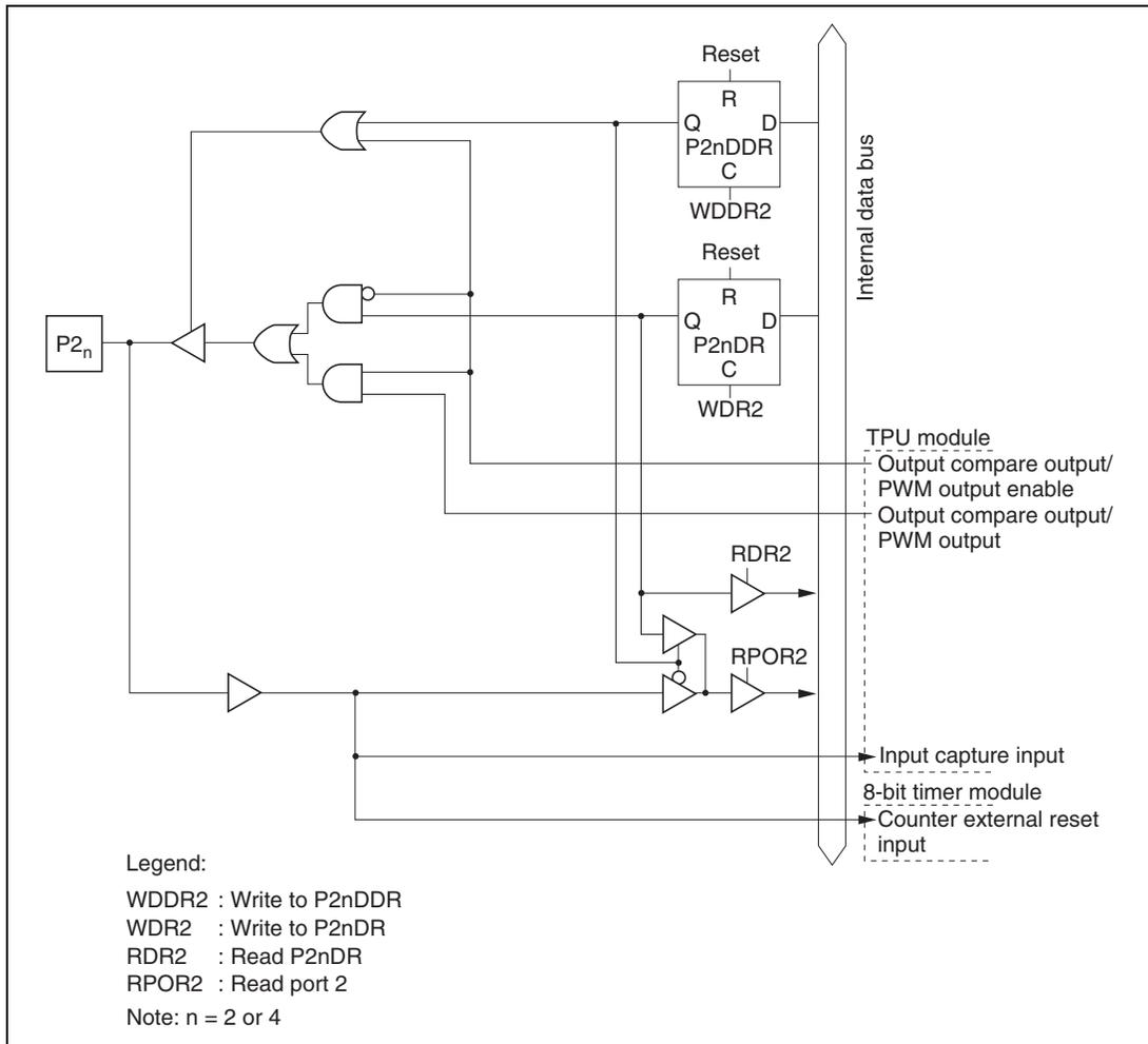
Figure C.2 (b) Port 2 Block Diagram (Pins P2<sub>2</sub> and P2<sub>4</sub>)
