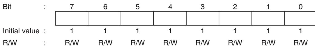
TDR is an 8-bit register that stores data for serial transmission.
