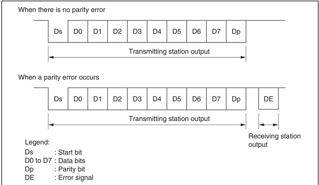
**Figure 13.3 Smart Card Interface Data Format**
