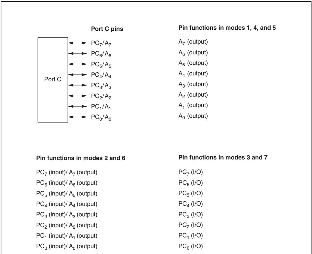
**Figure 8.15 Port C Pin Functions**
