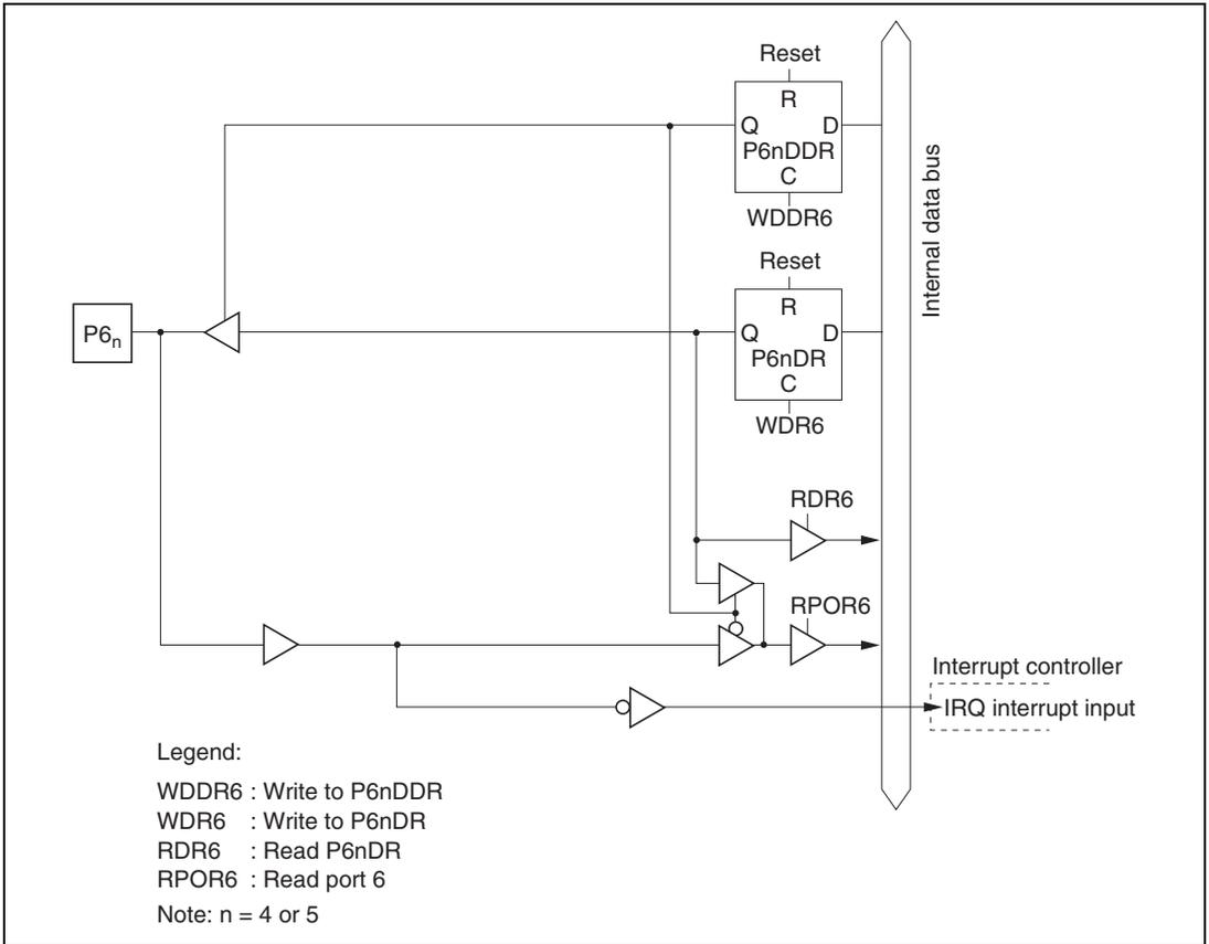
Figure C.6 (c) Port 6 Block Diagram (Pins P6<sub>4</sub> and P6<sub>5</sub>)
