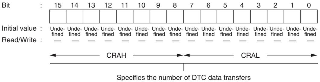
**CRB—DTC Transfer Count Register B****H'F800—H'FBFF****DTC**
