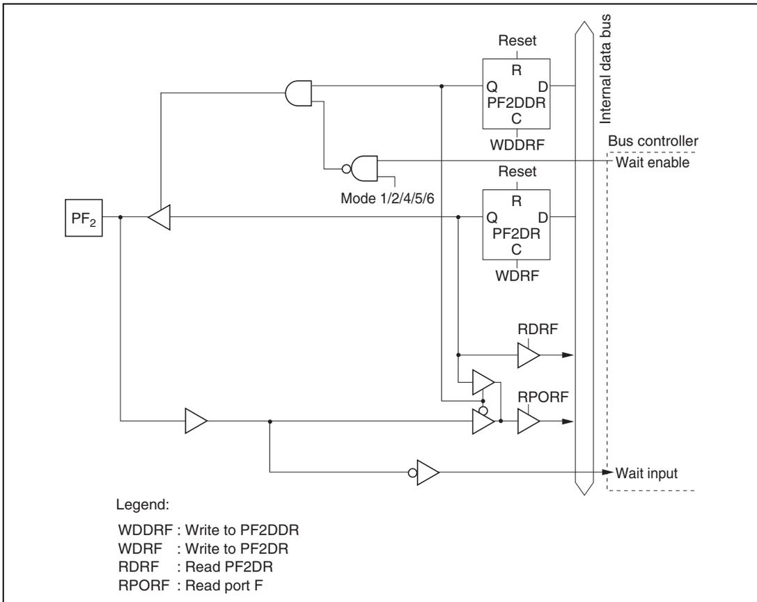
Figure C.12 (c) Port F Block Diagram (Pin PF<sub>2</sub>)
