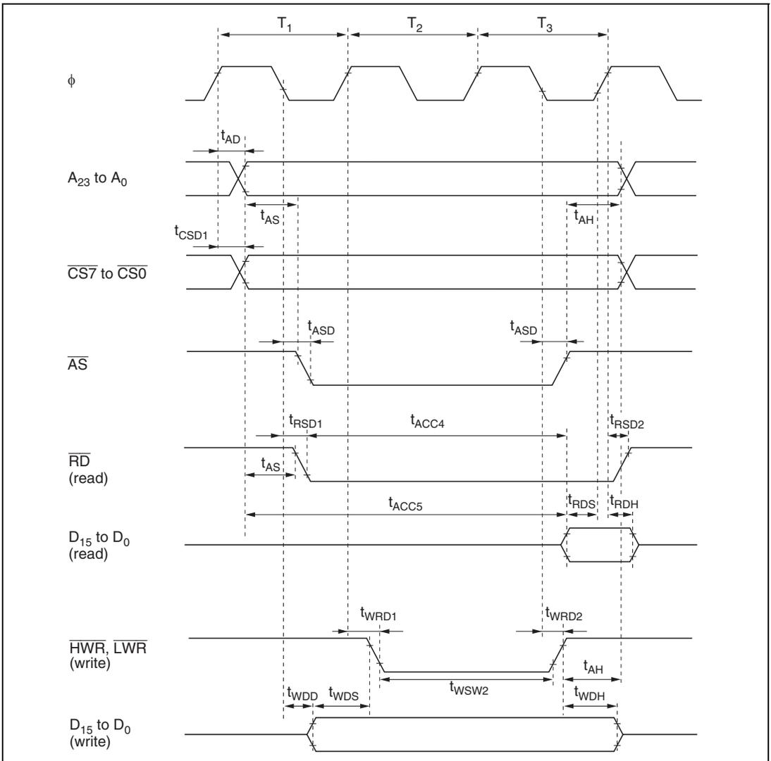
Figure 20.9 Basic Bus Timing (Three-State Access)
