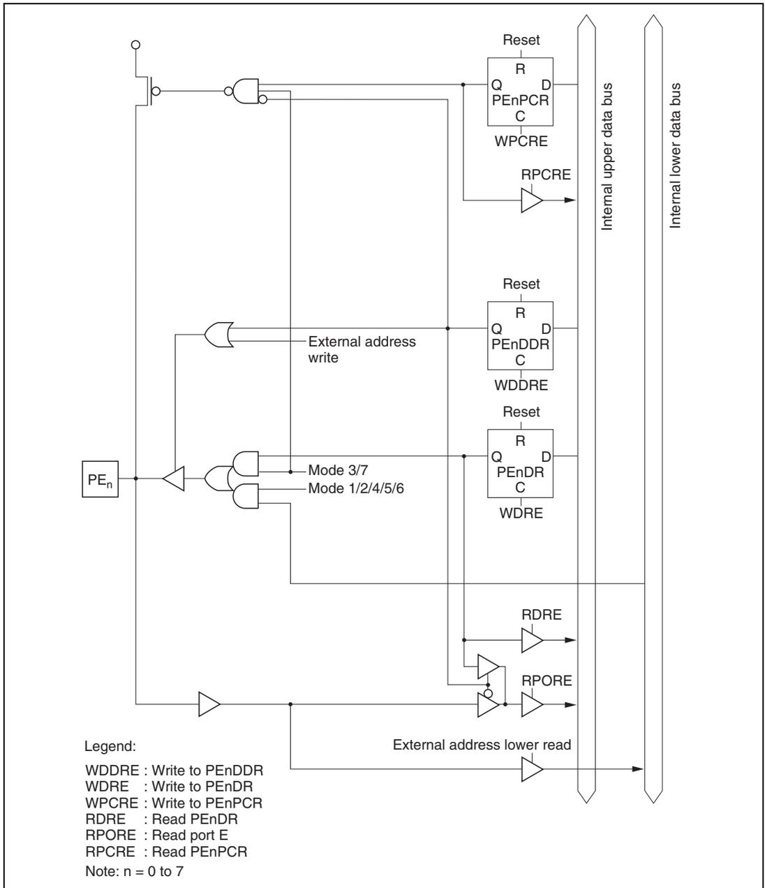
**Figure C.11 Port E Block Diagram (Pin  $PE_n$ )**
