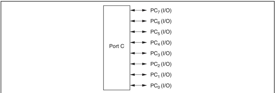
**Figure 8.18 Port C Pin Functions (Modes 3 and 7)**
