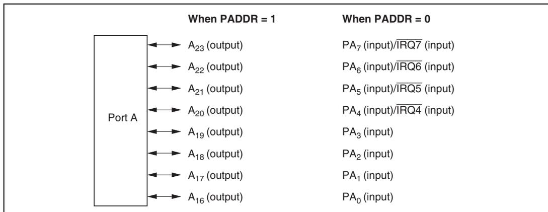
**Figure 8.10 Port A Pin Functions (Mode 6)**
