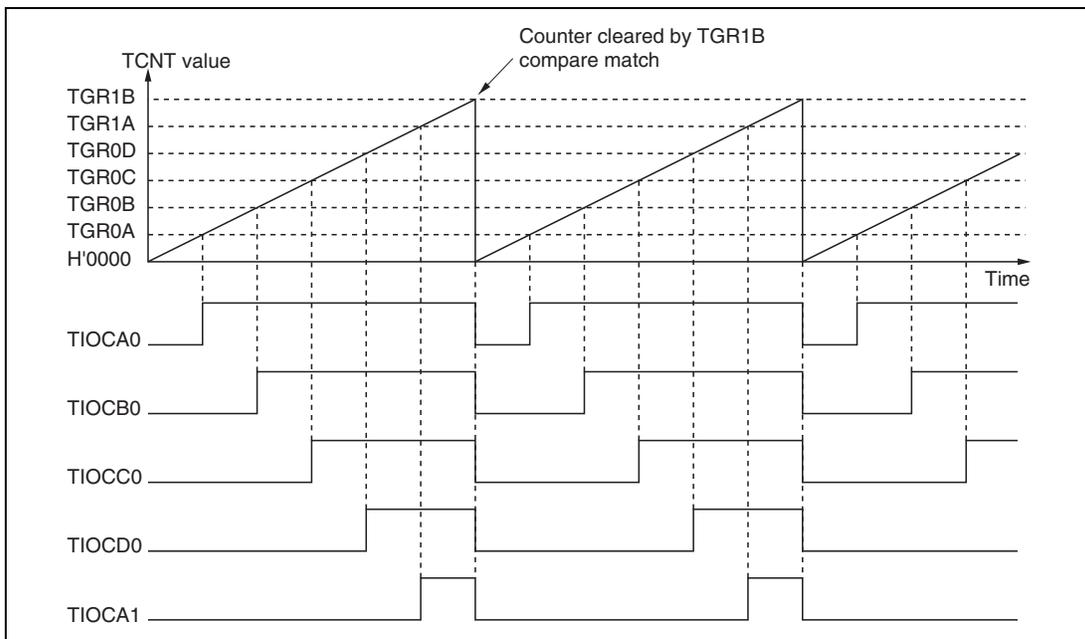
**Figure 9.26 Example of PWM Mode Operation (2)**
