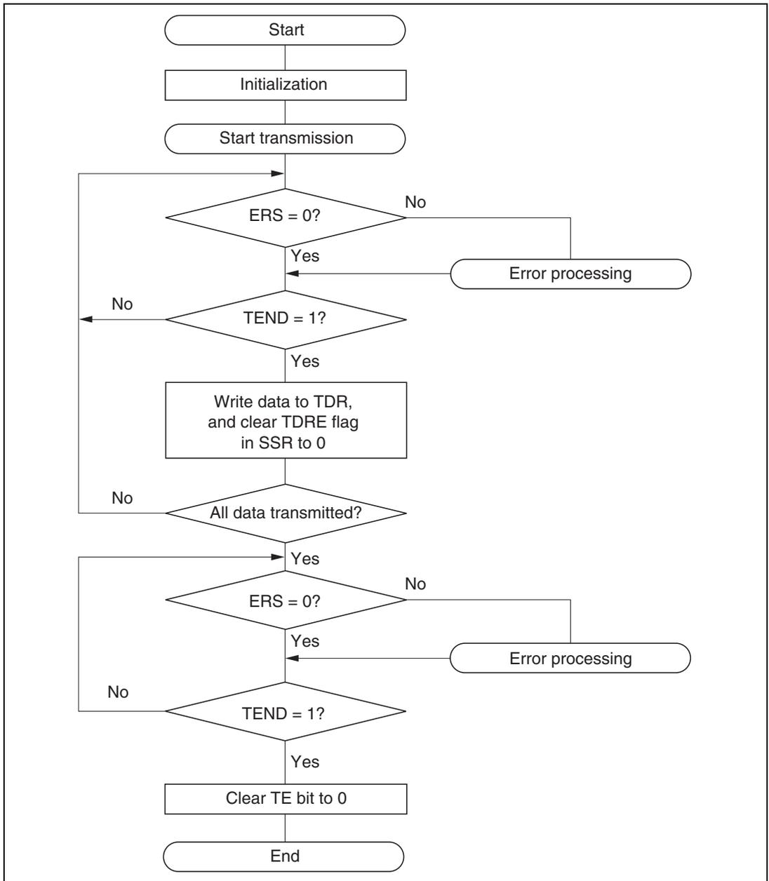
**Figure 13.4 Example of Transmission Processing Flow**
