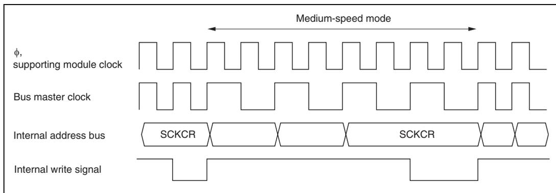
**Figure 19.1 Medium-Speed Mode Transition and Clearance Timing**
