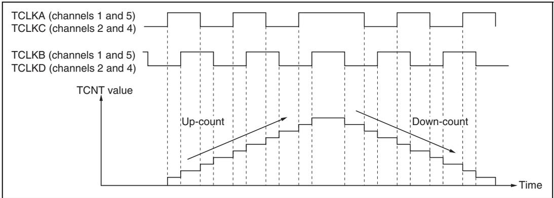
**Figure 9.29 Example of Phase Counting Mode 1 Operation**
