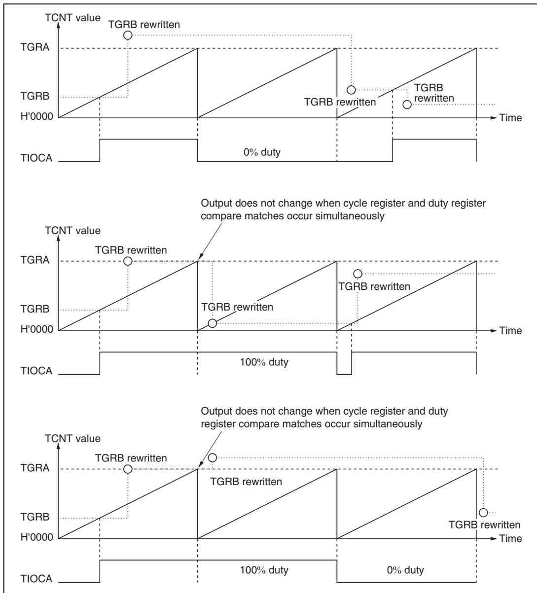
**Figure 9.27 Example of PWM Mode Operation (3)**
