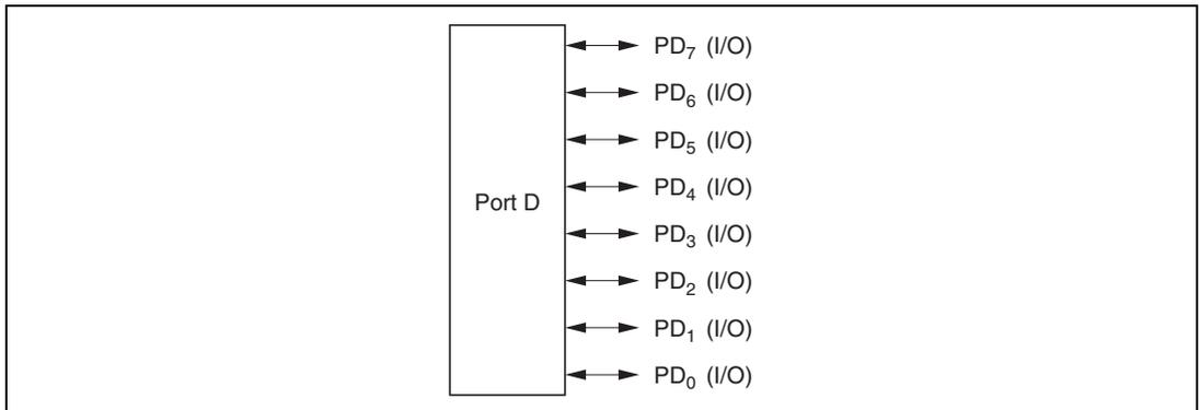
**Figure 8.21 Port D Pin Functions (Modes 3 and 7)**
