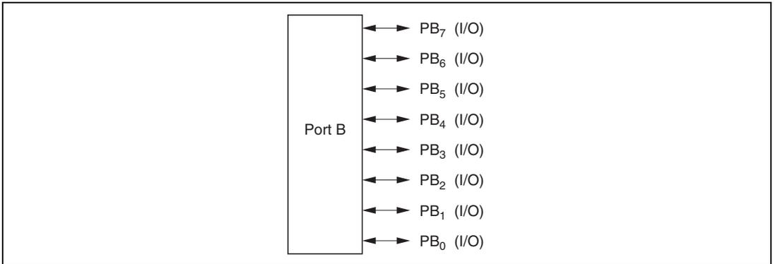
**Figure 8.14 Port B Pin Functions (Modes 3 and 7)**
