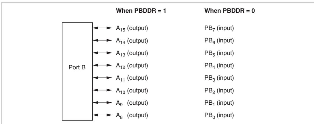
**Figure 8.13 Port B Pin Functions (Modes 2 and 6)**
