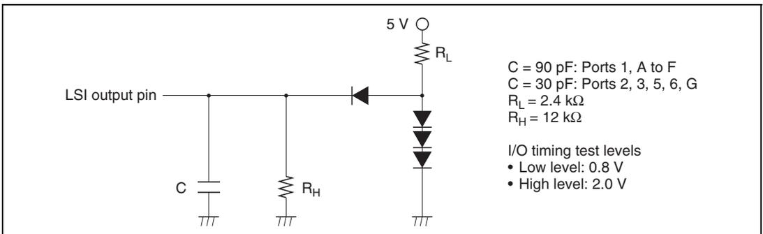
**Figure 20.3 Output Load Circuit**
