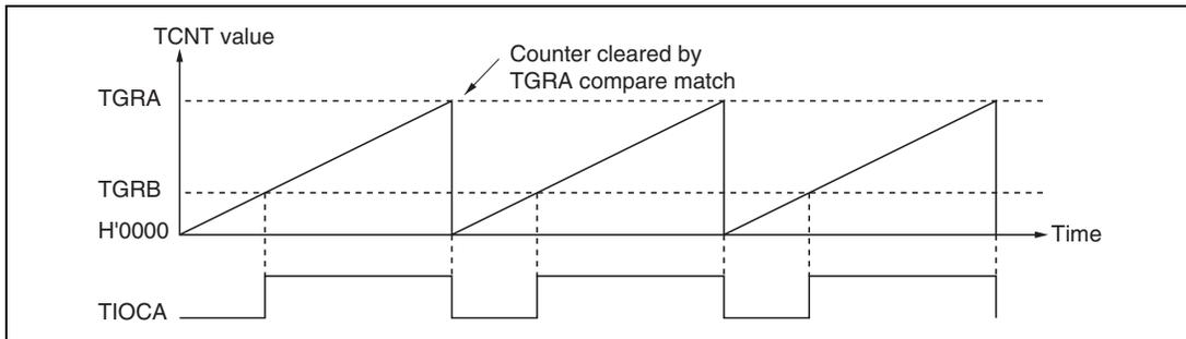
**Figure 9.25 Example of PWM Mode Operation (1)**
