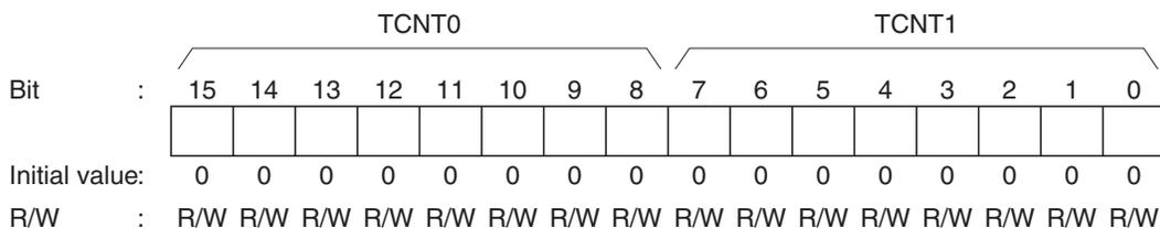
TCNT0 and TCNT1 are 8-bit readable/writable up-counters that increment on pulses generated from an internal or external clock source. This clock source is selected by clock select bits CKS2 to CKS0 of TCR. The CPU can read or write to TCNT0 and TCNT1 at all times.
