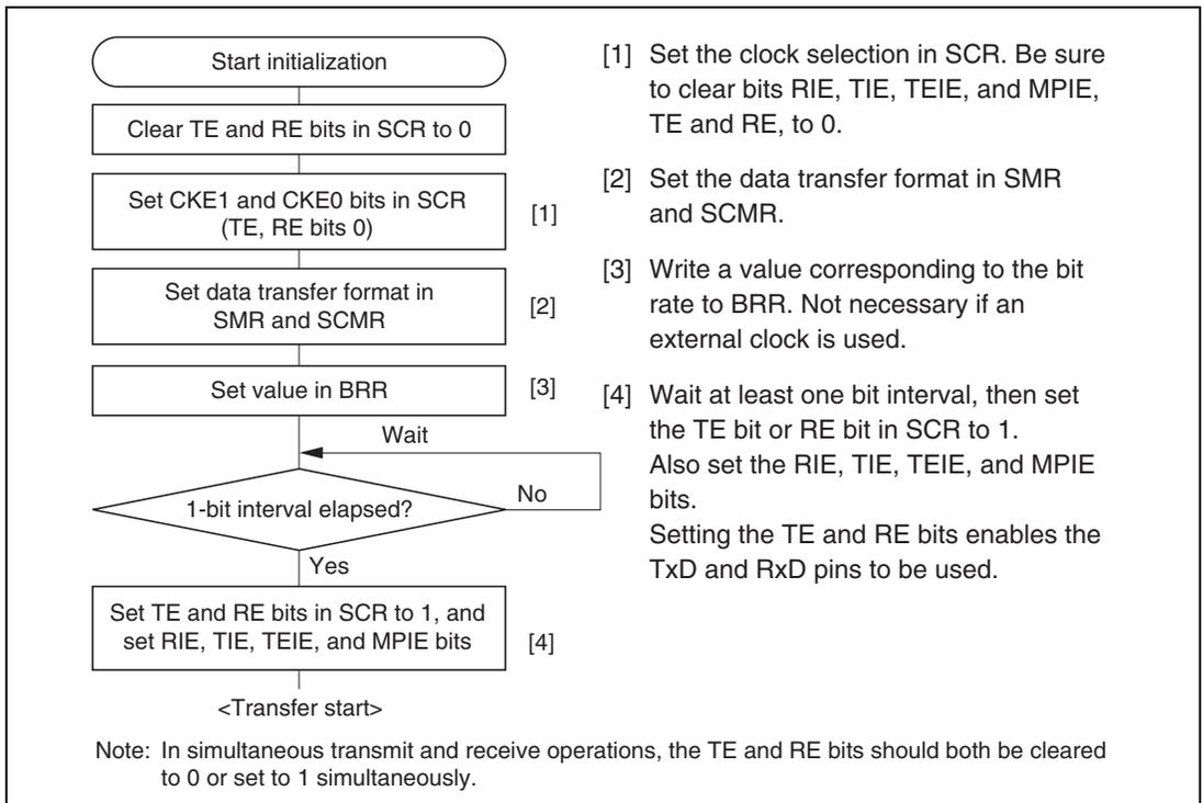
**Figure 12.15 Sample SCI Initialization Flowchart**
