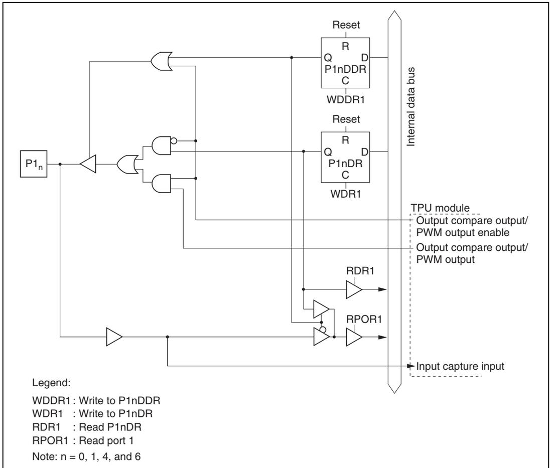
**Figure C.1 (a) Port 1 Block Diagram (Pins P1<sub>0</sub>, P1<sub>1</sub>, P1<sub>4</sub> and P1<sub>6</sub>)**
