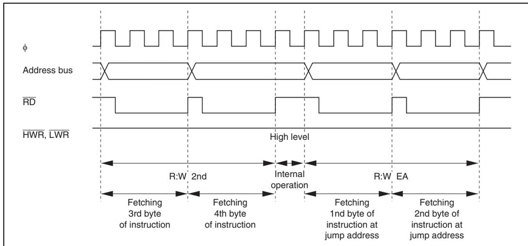
**Figure A.1 Address Bus,  $\overline{RD}$ ,  $\overline{HWR}$ , and  $\overline{LWR}$  Timing
