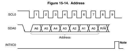
Note INTIIC0 is not issued if data other than a local address or extension code is received during slave device operation.
