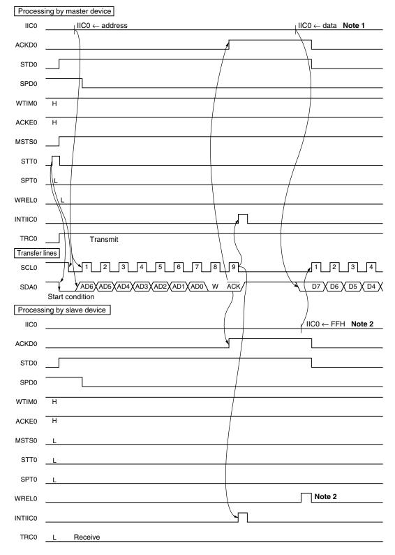
Notes 1. Write data to IIC0, not setting WREL0, in order to cancel a wait state during master transmission.2. To cancel slave wait, write "FFH" to IIC0 or set WREL0.
