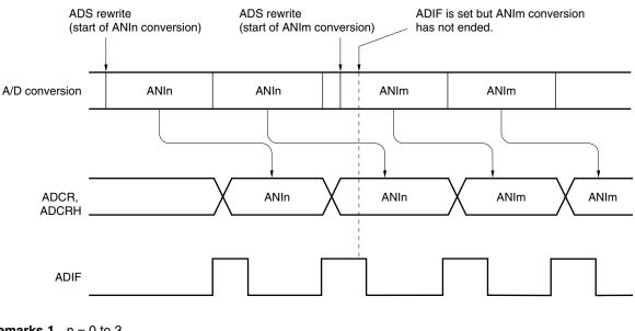
Figure 11-21. Timing of A/D Conversion End Interrupt Request Generation
