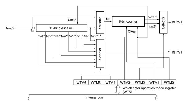
Figure 9-1. Block Diagram of Watch Timer
