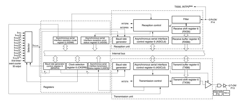
Figure 13-4. Block Diagram of Serial Interface UART6
