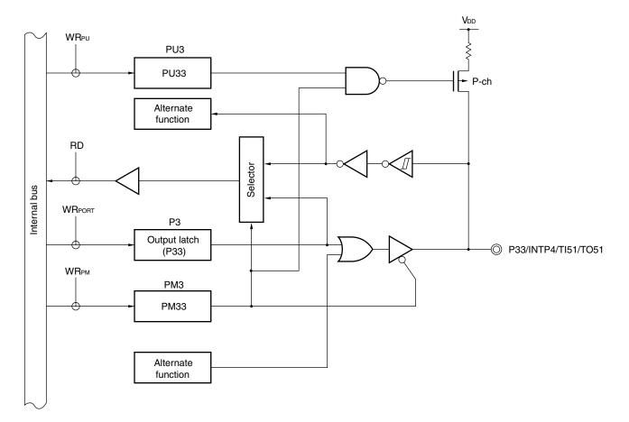
Figure 4-10. Block Diagram of P33
