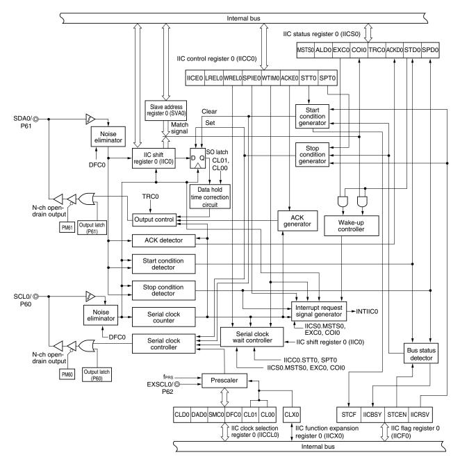
Figure 15-1. Block Diagram of Serial Interface IIC0
