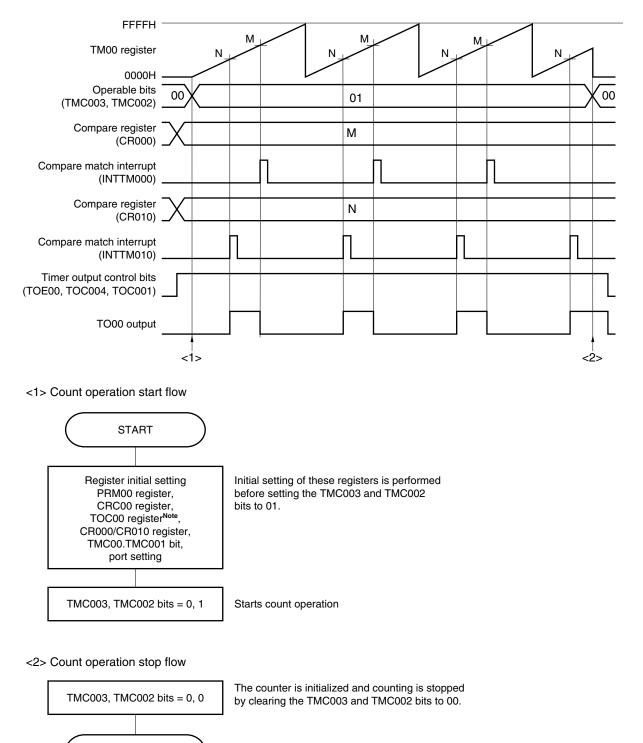
Figure 6-39. Example of Software Processing in Free-Running Timer Mode
