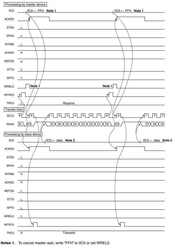
2. Write data to IIC0, not setting WREL0, in order to cancel a wait state during slave transmission.
