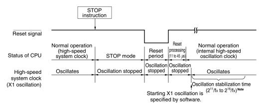
**Note** Oscillation stabilization time is not required when using the external main system clock (fexclk) as the high-speed system clock.
