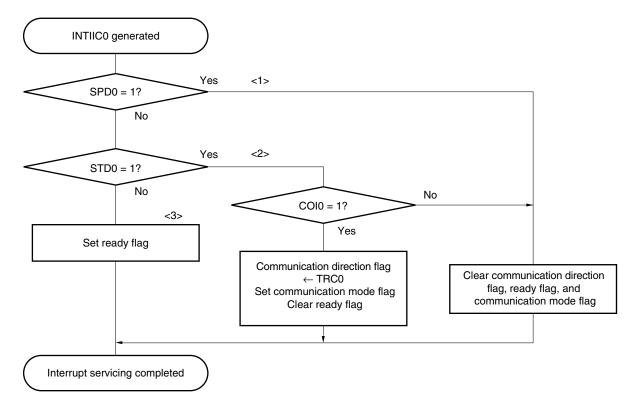
Figure 15-26. Slave Operation Flowchart (2)
