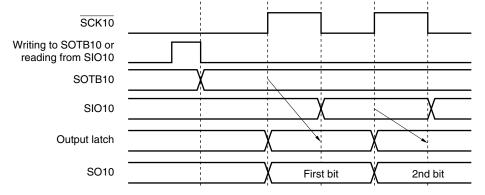
The first bit is directly latched by the SOTB10 register to the output latch at the falling (or rising) edge of  $\overline{SCK10}$ , and output from the SO10 pin via an output selector. Then, the value of the SOTB10 register is transferred to the SIO10 register at the next rising (or falling) edge of  $\overline{SCK10}$ , and shifted one bit. At the same time, the first bit of the receive data is stored in the SIO10 register via the SI10 pin.
