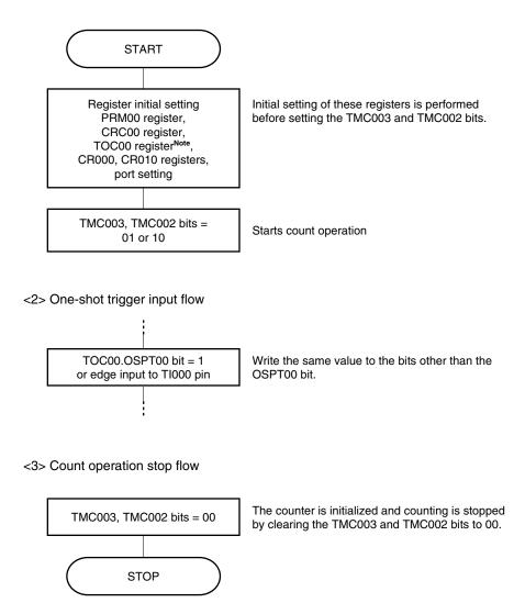
Note Care must be exercised when setting TOC00. For details, refer to 6.3 (3) 16-bit timer output control register 00 (TOC00).
