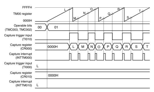
Figure 6-37. Timing Example of Free-Running Timer Mode (CR000: Capture Register, CR010: Capture Register) (2/2)
