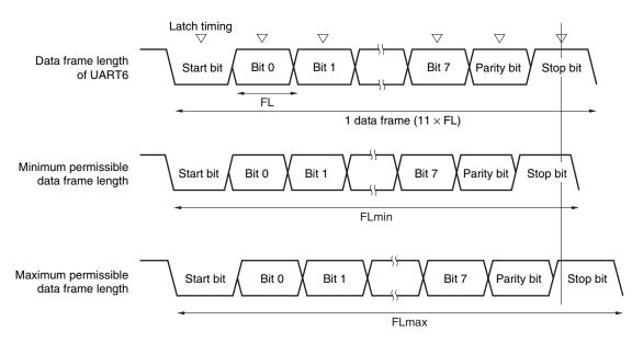
Figure 13-25. Permissible Baud Rate Range During Reception
