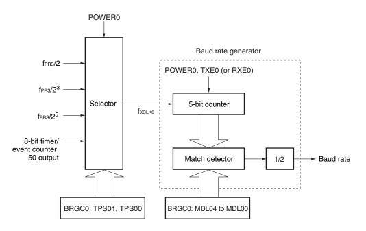
Figure 12-11. Configuration of Baud Rate Generator
