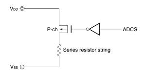
Figure 11-2. Circuit Configuration of Series Resistor String
