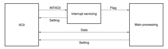
Therefore, data communication processing is performed by preparing the following three flags and passing them to the main processing instead of INTIICO.
