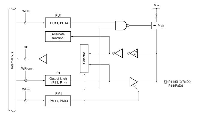
Figure 4-4. Block Diagram of P11 and P14
