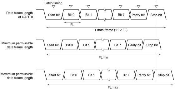
Figure 12-12. Permissible Baud Rate Range During Reception
