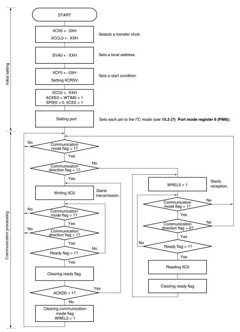
Figure 15-25. Slave Operation Flowchart (1)
