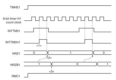
Figure 8-13. Transfer Timing
