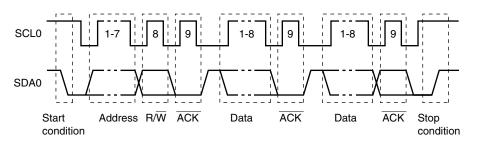
The master device generates the start condition, slave address, and stop condition.
