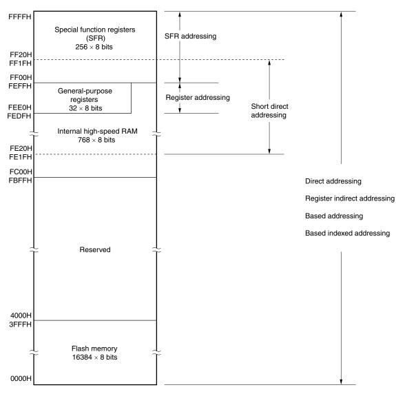
Figure 3-4. Correspondence Between Data Memory and Addressing (R7F0C011B)
