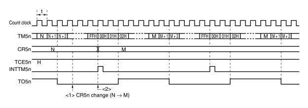
(a) CR5n value is changed from N to M before clock rising edge of FFH  $\rightarrow$  Value is transferred to CR5n at overflow immediately after change.
