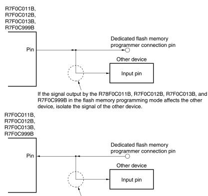
Figure 22-7. Malfunction of Other Device
