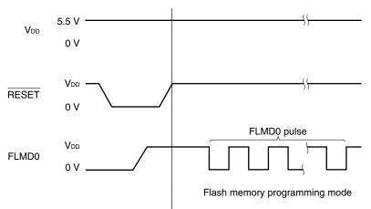
Table 22-5. Relationship Between FLMD0 Pin and Operation Mode After Reset Release
