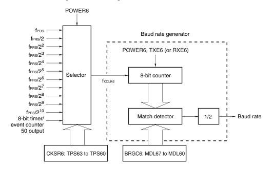
Figure 13-24. Configuration of Baud Rate Generator
