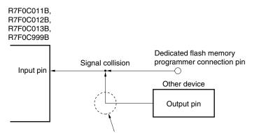
In the flash memory programming mode, the signal output by the device collides with the signal sent from the dedicated flash programmer. Therefore, isolate the signal of the other device.
