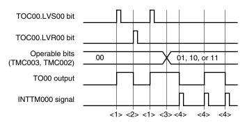
Figure 6-54. Timing Example of LVR00 and LVS00
