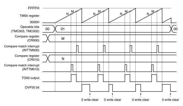
Figure 6-33. Timing Example of Free-Running Timer Mode (CR000: Compare Register, CR010: Compare Register)
