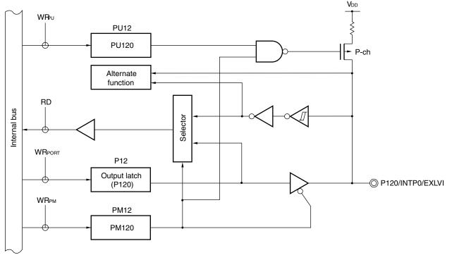
Figure 4-14. Block Diagram of P120
