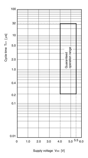
TCY vs. VDD (Main System Clock Operation)
