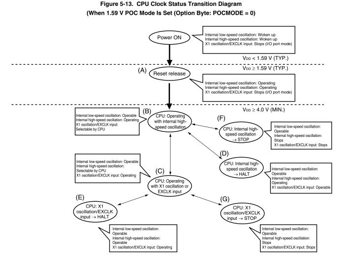
**Remark** In the 2.7 V/1.59 V POC mode (option byte: POCMODE = 1), the CPU clock status changes to (A) in the above figure when the supply voltage exceeds 2.7 V (TYP.), and to (B) after reset processing (11 to  $45 \ \mu$ s).
