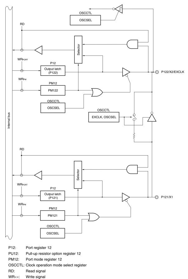
Figure 4-15. Block Diagram of P121 and P122
