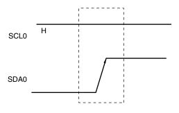
A stop condition is generated when bit 0 (SPT0) of IIC control register 0 (IICC0) is set to 1. When the stop condition is detected, bit 0 (SPD0) of IIC status register 0 (IICS0) is set to 1 and INTIIC0 is generated when bit 4 (SPIE0) of IICC0 register is set to 1.
