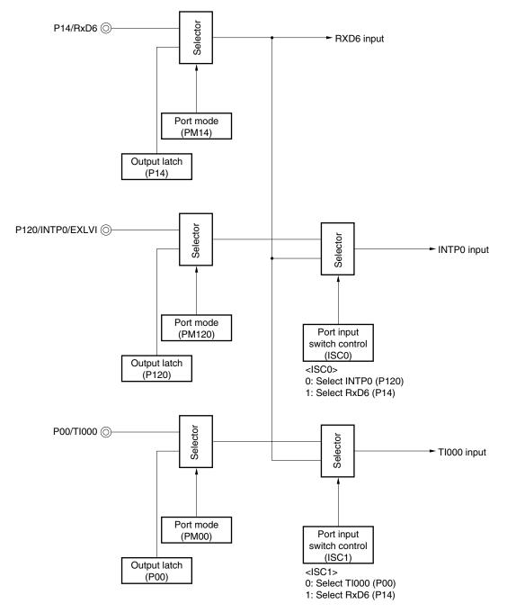
Remark ISC0, ISC1: Bits 0 and 1 of the input switch control register (ISC) (see Figure 13-11)
