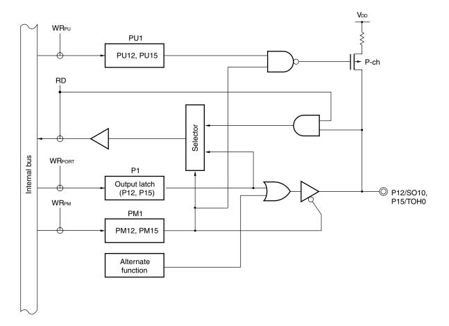
Figure 4-5. Block Diagram of P12 and P15
