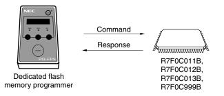
The flash memory control commands of the R7F0C011B, R7F0C012B, R7F0C013B, and R7F0C999B are listed in the table below. All these commands are issued from the programmer and the R7F0C011B, R7F0C012B, R7F0C013B, and R7F0C999B perform processing corresponding to the respective commands.
