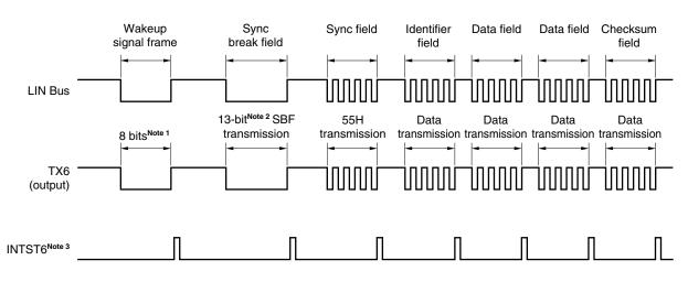
Figure 13-1. LIN Transmission Operation
