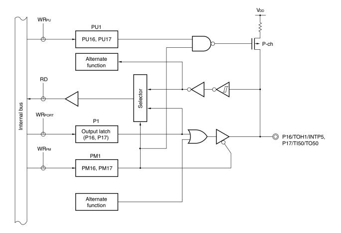
Figure 4-7. Block Diagram of P16 and P17
