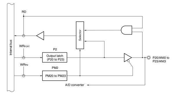
Figure 4-8. Block Diagram of P20 to P23
