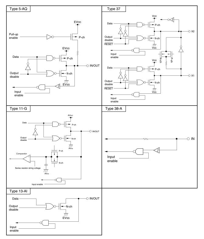
Figure 2-1. Pin I/O Circuit List (2/2)
