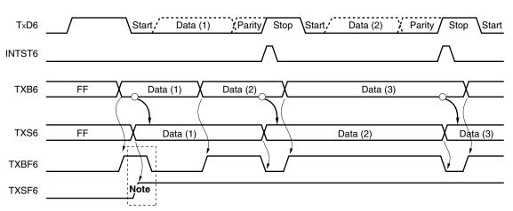
Figure 13-17. Timing of Starting Continuous Transmission
