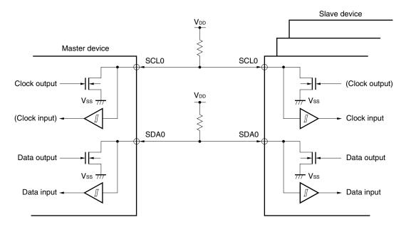
Figure 15-11. Pin Configuration Diagram
