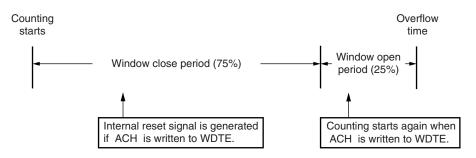
Caution The first writing to WDTE after a reset release clears the watchdog timer, if it is made before the overflow time regardless of the timing of the writing, and the watchdog timer starts counting again.
