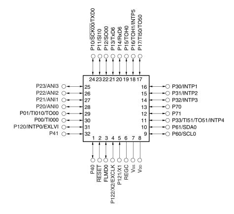
Cautions 1. Connect the REGC pin to Vss via a capacitor (0.47 to 1  $\mu$ F). 2. ANI0/P20 to ANI3/P23 are set in the analog input mode after release of reset.
